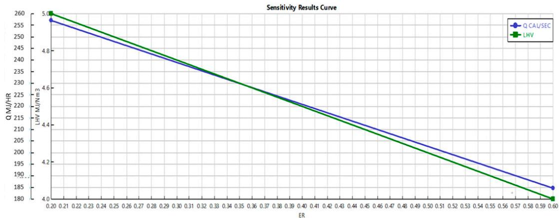
Figure 6. Gasifier heat demand and LHV vs. ER.
