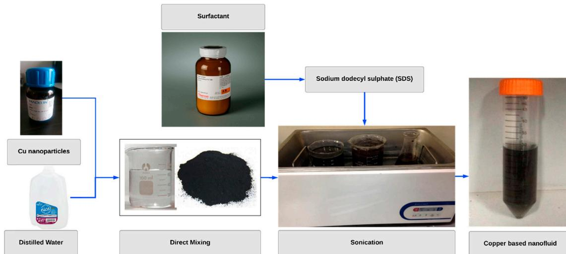
Figure 2. The preparation of copper based nanofluid.
