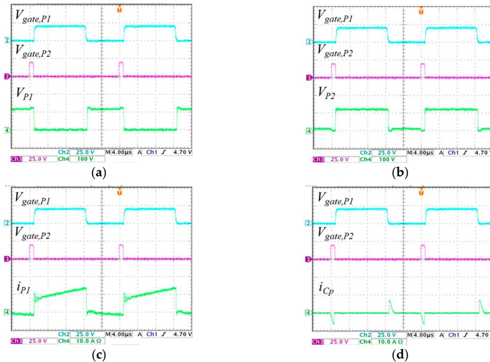
**Figure 12.** Experimental waveforms of the proposed inverter: (a)  $V_{gate,P1}$ ,  $V_{gate,P2}$ , and  $V_{P1}$ ; (b)  $V_{gate,P1}$ ,  $V_{gate,P2}$ , and  $V_{P2}$ ; (c)  $V_{gate,P1}$ ,  $V_{gate,P2}$ , and  $i_{P1}$ ; and (d)  $V_{gate,P1}$ ,  $V_{gate,P2}$ , and  $i_{Cp}$ .
