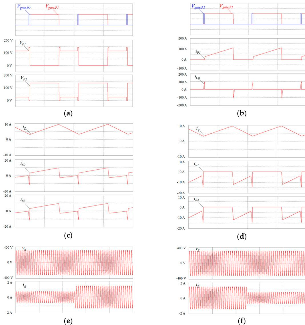
**Figure 10.** Simulation waveforms: (a)  $V_{gate,P1}$ ,  $V_{gate,P2}$ ,  $V_{P1}$ , and  $V_{P2}$ ; (b)  $V_{gate,P1}$ ,  $V_{gate,P2}$ ,  $i_{P1}$ , and  $i_{CP}$ ; (c)  $i_g$ ,  $i_{S2}$ , and  $i_{S3}$ ; (d)  $i_g$ ,  $i_{S1}$ , and  $i_{S4}$ ; (e)  $v_g$  and  $i_g$  from 110 W to 220 W; and (f)  $v_g$  and  $i_g$  from 220 W to 110 W.
