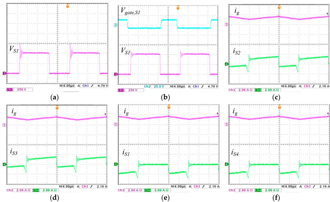
**Figure 13.** Experimental waveforms in the secondary circuit for the positive grid cycle: (a)  $V_{S1}$  in the previous inverter; (b)  $V_{gate,S1}$  and  $V_{S1}$  in the proposed inverter; (c)  $i_g$  and  $i_{S2}$  in the proposed inverter; (d)  $i_g$  and  $i_{S3}$  in the proposed inverter; (e)  $i_g$  and  $i_{S1}$  in the proposed inverter; and (f)  $i_g$  and  $i_{S4}$  in the proposed inverter.
