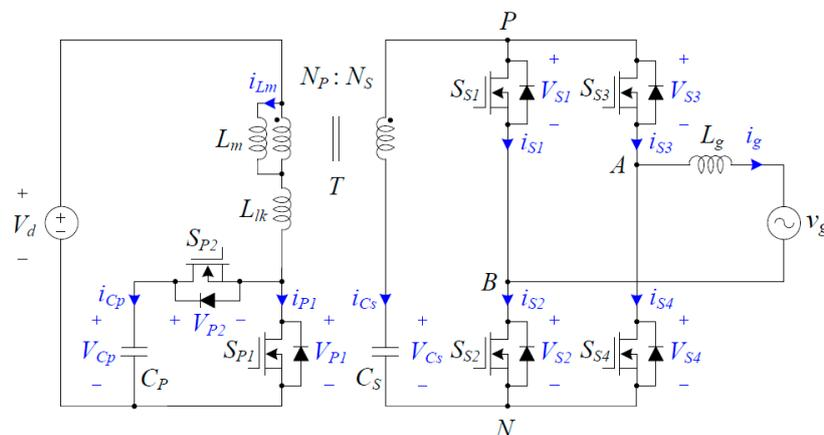
Figure 3. Circuit diagram of the proposed inverter with reference directions of currents and voltages.
