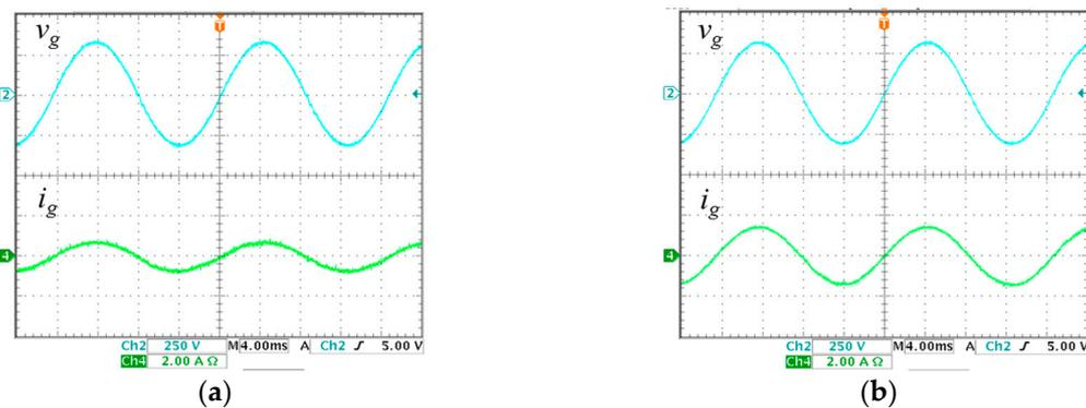
**Figure 14.** Experimental waveforms of the proposed inverter: (a)  $v_g$  and  $i_g$  as the proposed inverter supplies 110 W into the grid; and (b)  $v_g$  and  $i_g$  as the proposed inverter supplies 220 W into the grid.
