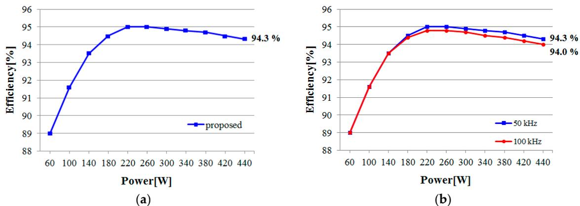
**Figure 16.** Measured power efficiency curves: (a) power efficiency curves up to 440 W; and (b) power efficiency curves for different switching frequencies.
