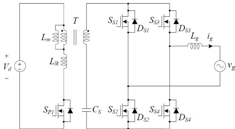
Figure 1. Circuit diagram of the zeta inverter.
