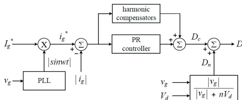
Figure 8. Control block diagram of the proposed inverter.
