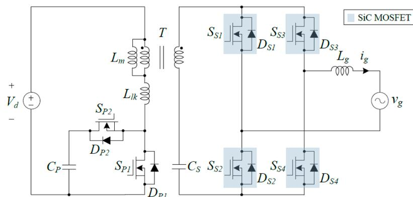
Figure 2. Circuit diagram of the proposed inverter.
