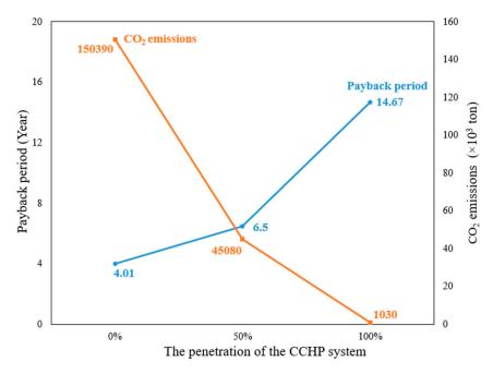
**Figure 11.** The economic and environmental performance of the CCHP system with different penetration rates.
