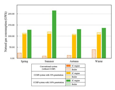
Figure 9. The seasonal natural gas consumption of the three systems simulated in the model.
