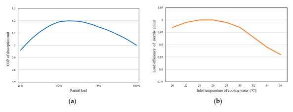
Figure 5. The performance of the absorption unit and electric chiller under partial load: (a) the part load performance of the absorption unit; and (b) the load efficiency of the electric chiller.
