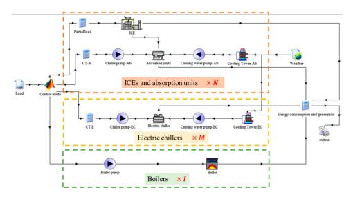
Figure 4. The simulation diagram of operation mode.
