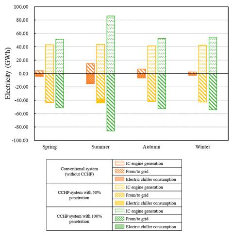
**Figure 10.** The seasonal electricity consumption and generation of the three systems simulated in the model.
