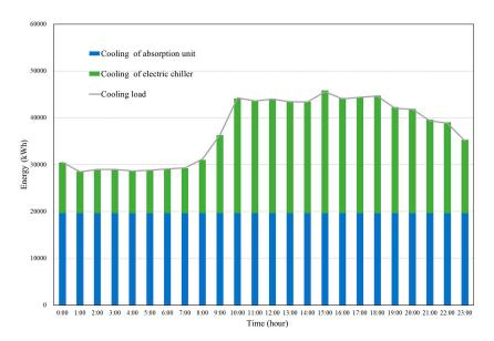
Figure 6. Hourly cooling supply and demand balance in summer.
