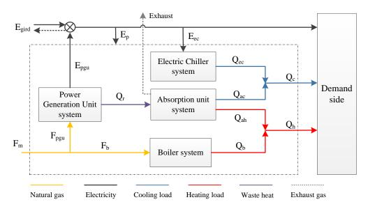
Figure 2. Energy flow diagram of the CCHP system.
