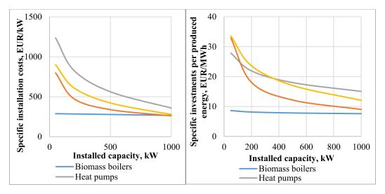
Figure 4. Estimated benchmarks for different RE technologies in individual heating.
