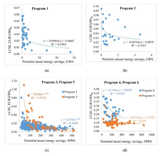
**Figure 6.** Regression analyses for analysed energy efficiency programs: (**a**) Program 1 for manufacturing companies; (**b**) Program 2 for district heating companies; (**c**) Program 3 and Program 5 for apartment building renovation; (**d**) Program 4 and Program 6 for municipalities' building renovation.
