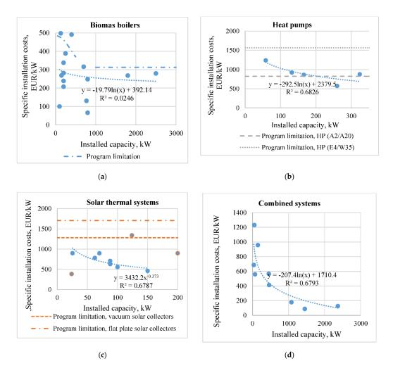
**Figure 3.** Regression analyses and the set specific cost limits of the program for different RES technologies: (**a**) biomass boilers; (**b**) heat pumps; (**c**) solar thermal systems and (**d**) combined systems.
