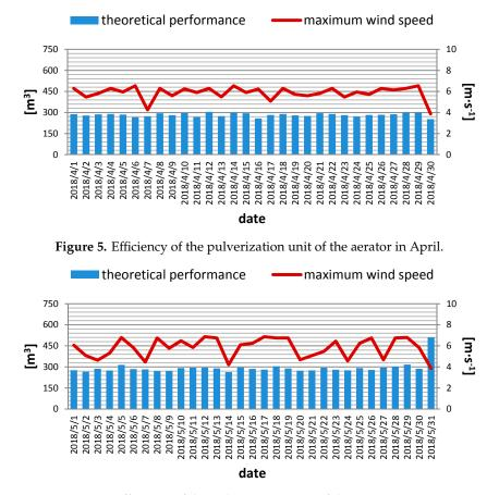
Figure 6. Efficiency of the pulverization unit of the aerator in May.
