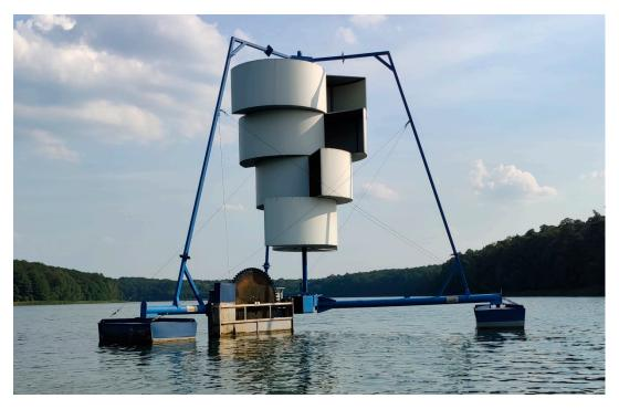
Figure 1. Wind-driven pulverizing aerator located on Góreckie Lake.
