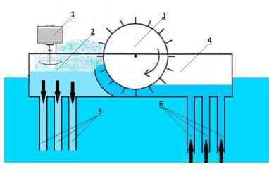
**Figure 2.** Scheme of the pulverization unit in the aerator. Note: 1, coagulant applicator; 2, pressuring chamber; 3, pulverizing circle; 4, suction chamber; 5, pressuring hoses; 6, suction hoses.
