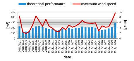
Figure 12. Efficiency of the pulverization unit of the aerator in November.
