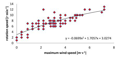
Figure 3. Rotational speed model of the aerator pulverization wheel in relation to wind speed.
