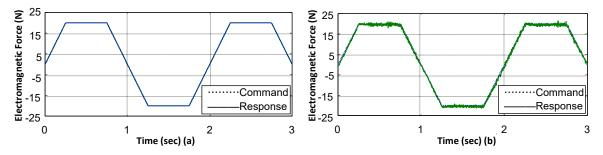
**Figure 9.** Feedback linearization control experiment—simulated (**a**) and measured (**b**) responses from electromagnetic force (trapezoidal wave) commands.
