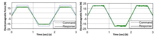
**Figure 10.** Measured responses from electromagnetic force (trapezoidal wave) commands with stator flux set to 1.5 times the original setting: (a) feedback linearization controller only; (b) robust control mechanism added.
