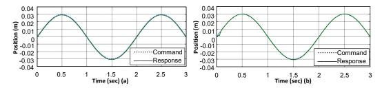
**Figure 12.** Feedback linearization control experiment—(a) simulated and (b) measured responses from position (sine wave) commands.
