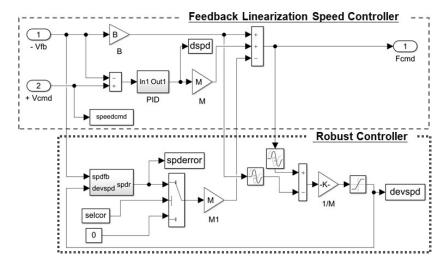
Figure 5. Design block diagrams of robust controller and feedback linearization speed controller.
