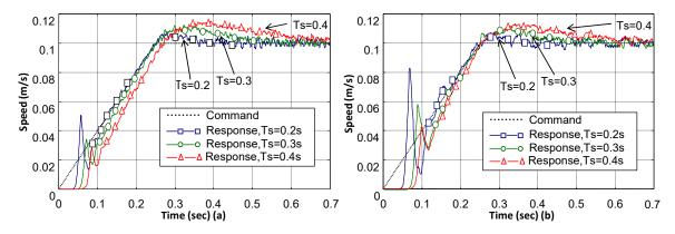
**Figure 16.** Settling time tests of feedback linearization controller with robust control—measured responses from speed (trapezoidal wave): (a) original parameter settings; (b) stator flux changed to 1.5 times the original settings.
