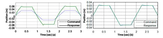
**Figure 14.** Measured responses from position (trapezoidal wave) commands with stator flux changed to 1.5 times the original setting: (a) feedback linearization controller only; (b) robust control mechanism added.
