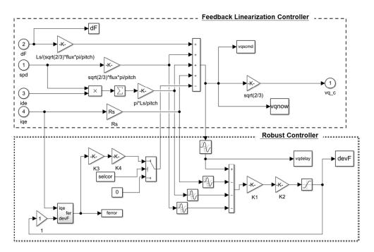
**Figure 3.** Design block diagrams of robust and feedback linearization controller for electromagnetic force control system.
