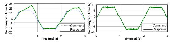
**Figure 11.** Measured responses from electromagnetic force (trapezoidal wave) commands with stator flux and resistivity changed to 1.5 times the original settings: (a) feedback linearization controller only; (b) robust control mechanism added.
