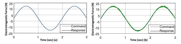
**Figure 8.** Feedback linearization control experiment—simulated (**a**) and measured (**b**) responses from 3 (sine wave) commands.
