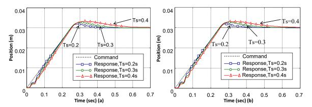
**Figure 17.** Settling time tests of feedback linearization controller with robust control—measured responses from position (trapezoidal wave): (a) original parameter settings; (b) stator flux changed to 1.5 times the original settings.
