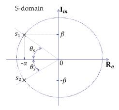
Figure 4. Poles placed on the s-plane.
