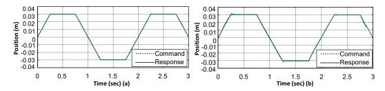
**Figure 13.** Feedback linearization control experiment—(a) simulated and (b) measured responses from position (trapezoidal wave) commands.
