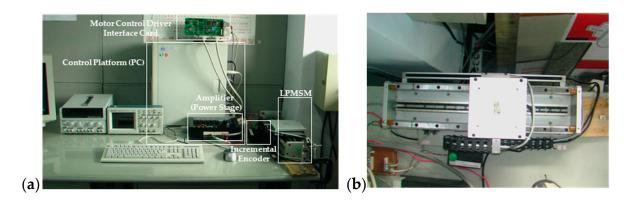
Figure 7. (a) PC-based LPMSM experiment system. (b) The top view of LPMSM.
