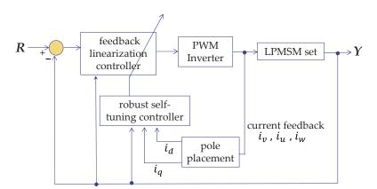
Figure 1. Block diagram of the linear permanent magnet synchronous motors (LPMSM) control system.
