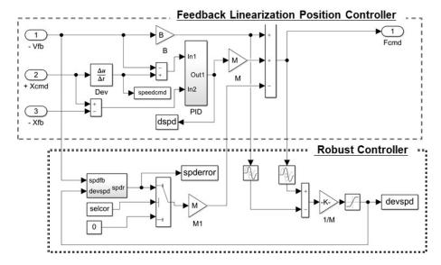
Figure 6. Design block diagrams of robust controller and feedback linearization position controller.
