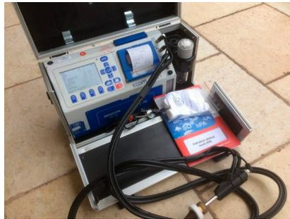
Figure 3. Exhaust gas analyzer with a measuring probe.
