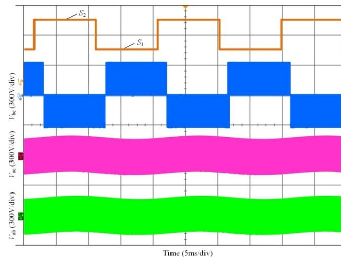
**Figure 16.** The curves of the sector and line-to-line voltage for the proposed MPDTC.
