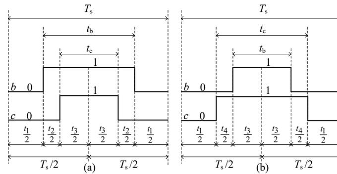
Figure 5. Switching sequence diagram (a) Switching sequence I (b) Switching sequence II.
