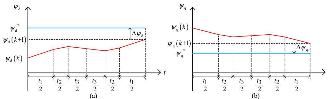
Figure 6. Trajectory of (a)  $\Psi_d$  and (b)  $\Psi_q$  with the switching sequence I.
