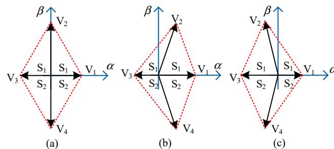
Figure 4. Space vector diagram for 3P4SI. (a)  $V_{c1} = V_{c2}$  (b)  $V_{c1} < V_{c2}$  (c)  $V_{c1} > V_{c2}$ .
