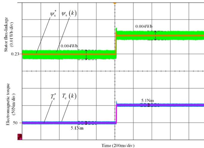
**Figure 11.** The curves of stator flux-linkage and electromagnetic torque for the proposed MPDTC.
