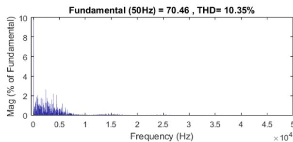
**Figure 14.** Spectrum of the phase current for the conventional MPDTC.
