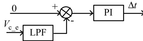
Figure 7. Diagram of capacitor voltage balancing strategy.
