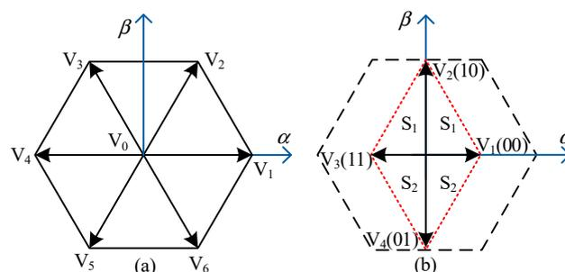
Figure 2. Space vector diagrams. (a) In normal mode. (b) In switch-open fault-tolerant mode.
