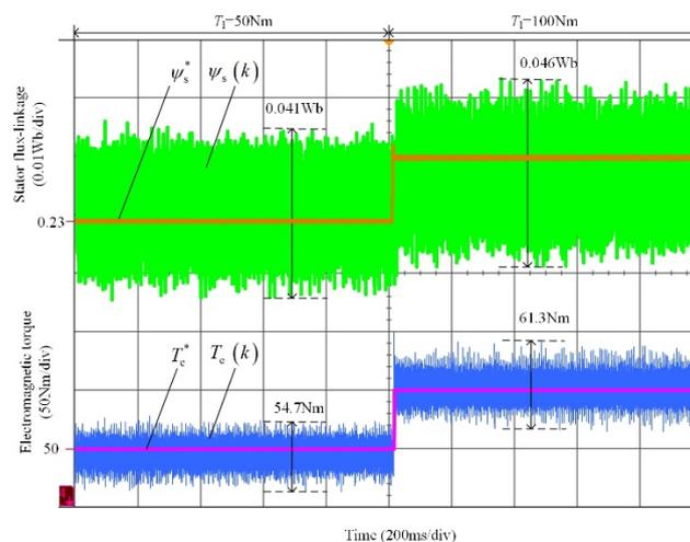
Figure 10. The curves of stator flux-linkage and electromagnetic torque for the conventional MPDTC.
