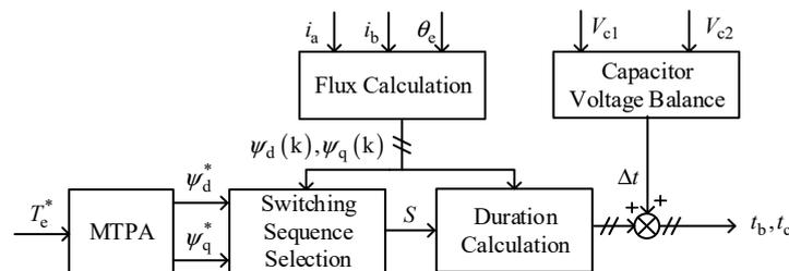
Figure 8. Control diagram of the switching sequence MPDTC.
