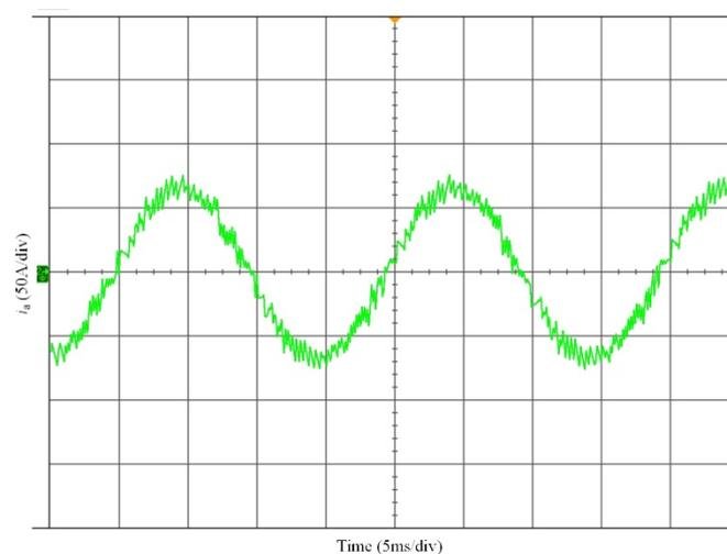
**Figure 12.** The curve of phase current for the conventional MPDTC.
