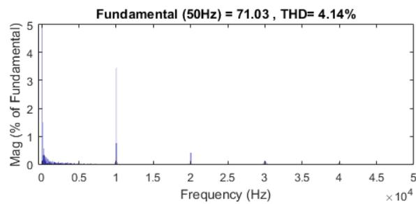
**Figure 15.** Spectrum of the phase current for the proposed MPDTC.
