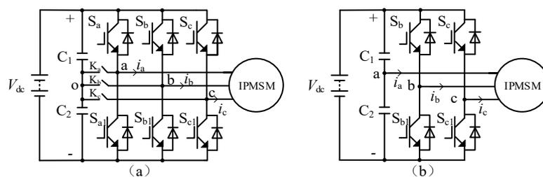
Figure 1. Speed regulation system of EVs on the basis of IPMSMs (a) 2L-VSI (b) 3P4SI.
