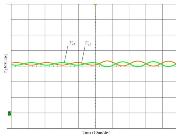
**Figure 17.** Curves of the capacitor voltages for the proposed MPDTC.
