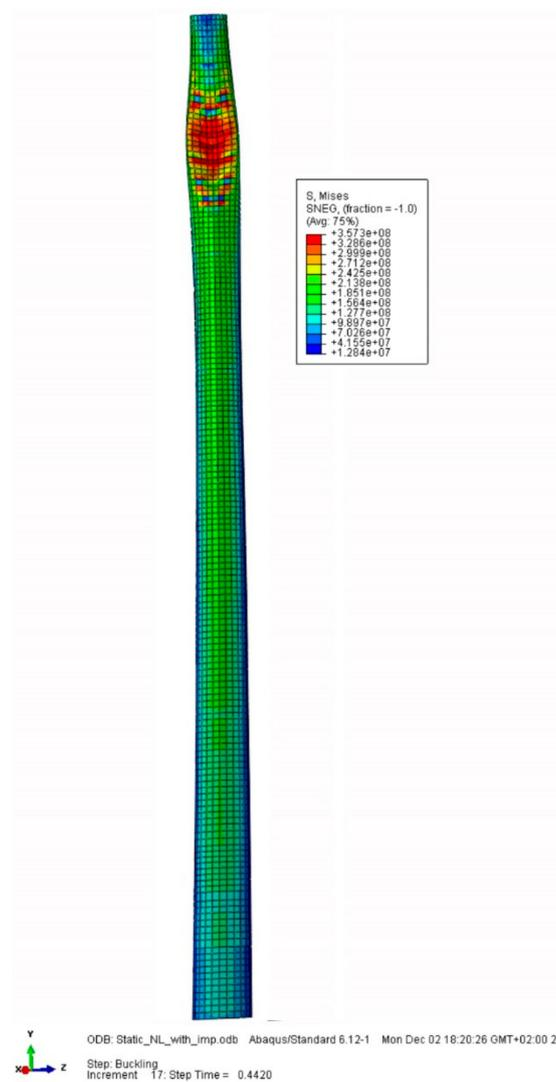
**Figure 8.** Material non-linear imperfection analysis results for Tower\_T\_A.
