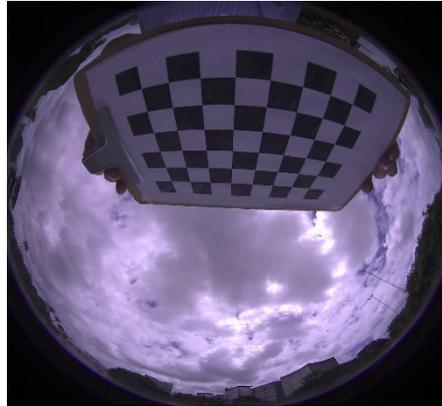
**Figure 5.** Chessboard image used to feed a model to undistort images of the fish-eye camera.
