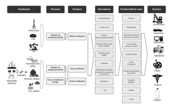
Figure 4. The methanol value chain. Adapted from [30,129].
