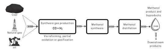
Figure 2. Schematic of the conventional methanol production process.
