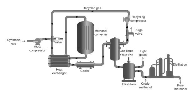
Figure 3. Schematic of a generic methanol synthesis process.
