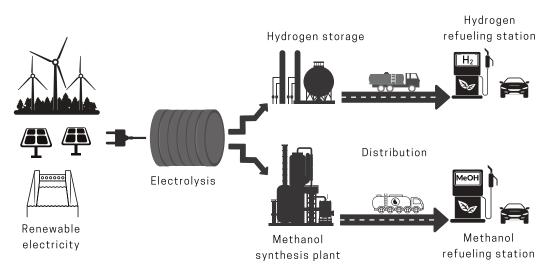
**Figure 7.** Renewable energy transformation pathways in the cases of methanol and hydrogen as energy carriers.
