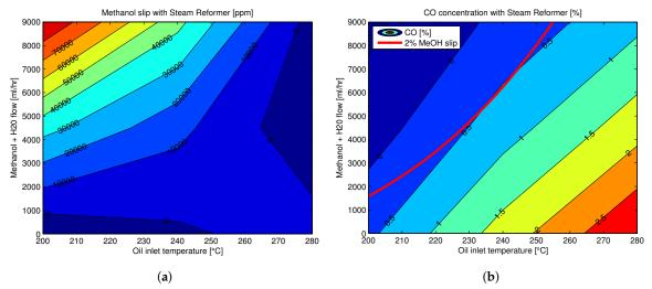
**Figure 6.** Reformate composition at the steam methanol reformer outlet at different reforming temperatures (given by the temperature at the inlet of the reformer) (**a**) Methanol concentration in reformate mixture at different reforming temperatures (**b**) CO concentration in reformate mixture at different reforming temperatures, with the red line showing the 2% methanol slip. Reprinted with permission from [161]; 2016, Aalborg Universitetsforlag.
