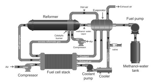
Figure 5. A schematic of a reformed methanol fuel cell system.
