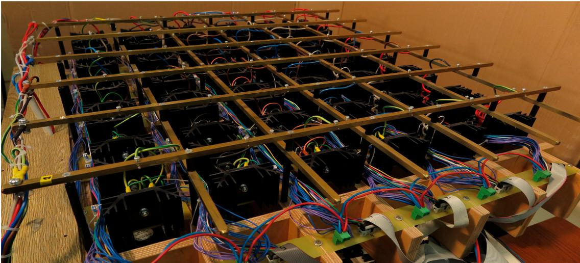
**Figure 4.** The 30 kVA-rated MC laboratory model of the  $6 \times 6$  structure used for evaluation of the converter ability to control reactive power flow.
