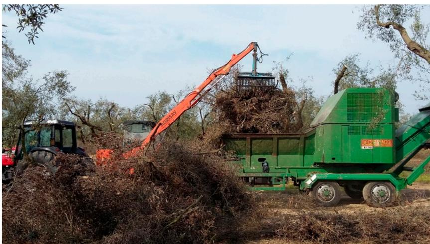
**Figure 2.** Stationary chipper Caravaggi and tractor with uploading equipment.
