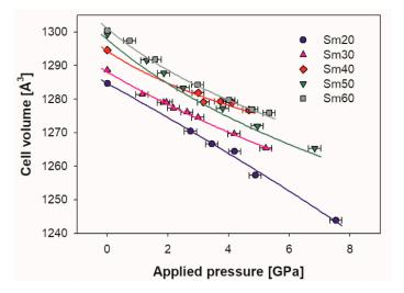
**Figure 5.** Evolution with pressure of the Sm-doped ceria cell volume for all the samples; experimental data are fitted by the third order Vinet EoS (continuous lines). Cell volumes of samples Sm20 and Sm30 are multiplied by 8 in order to make them comparable with those of Sm40, Sm50 and Sm60. Vertical error bars are hidden by data markers.
