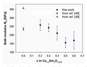
**Figure 6.** Zero-pressure bulk modulus ( $B_0$ ) as a function of the Sm content alongside literature data for CeO<sub>2</sub> [48,49].
