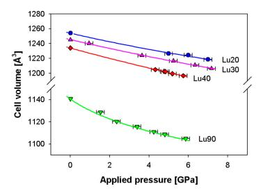
**Figure 8.** Dependence of the Lu-doped ceria cell volume vs. applied pressure; experimental data are taken from [13] and fitted by the third order Vinet EoS (continuous lines). Cell volumes of samples Lu20, Lu30 and Lu40 are multiplied by 8 in order to make them comparable with Sm90. Vertical error bars are hidden by data markers.
