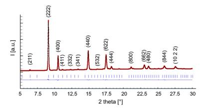
**Figure 3.** Rietveld refinement plot of sample Sm50\_6.94. The dotted (red) and the continuous (black) lines are the experimental and the calculated diffractograms, respectively; the lower line is the difference curve; vertical bars indicate the calculated positions of Bragg peaks. Miller indexes related to the H structure (space group  $Ia\bar{3}$ ) are reported too.
