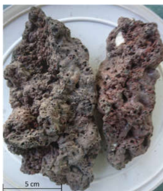
Figure 4. Bottom ash slag from the co-combustion of sewage sludge with soft wood, MSS-SW 30–70.
