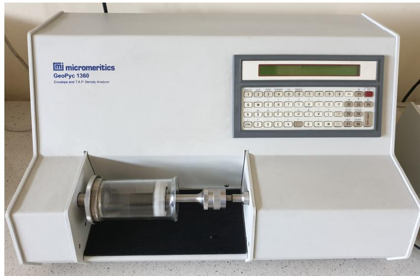
Figure 3. GeoPyc 1360 density determination station.
