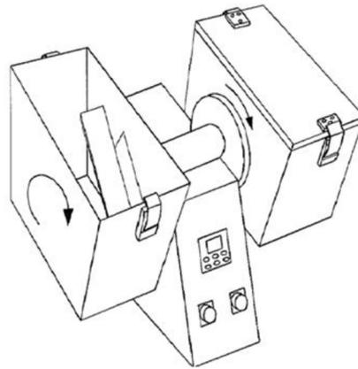
Figure 4. Mechanical durability determination station [48].
