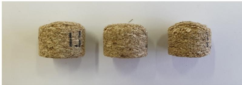
**Figure 8.** Samples after mechanical durability test-Sida.
