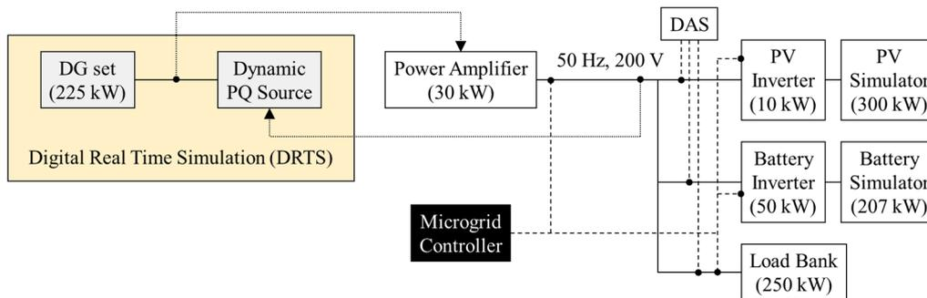
**Figure 5.** Power-hardware-in-the-loop (PHIL) testing setup for the microgrid controller in the test lab. The limitation of lab equipment is removed by integrating test lab with DRTS as PHIL environment.
