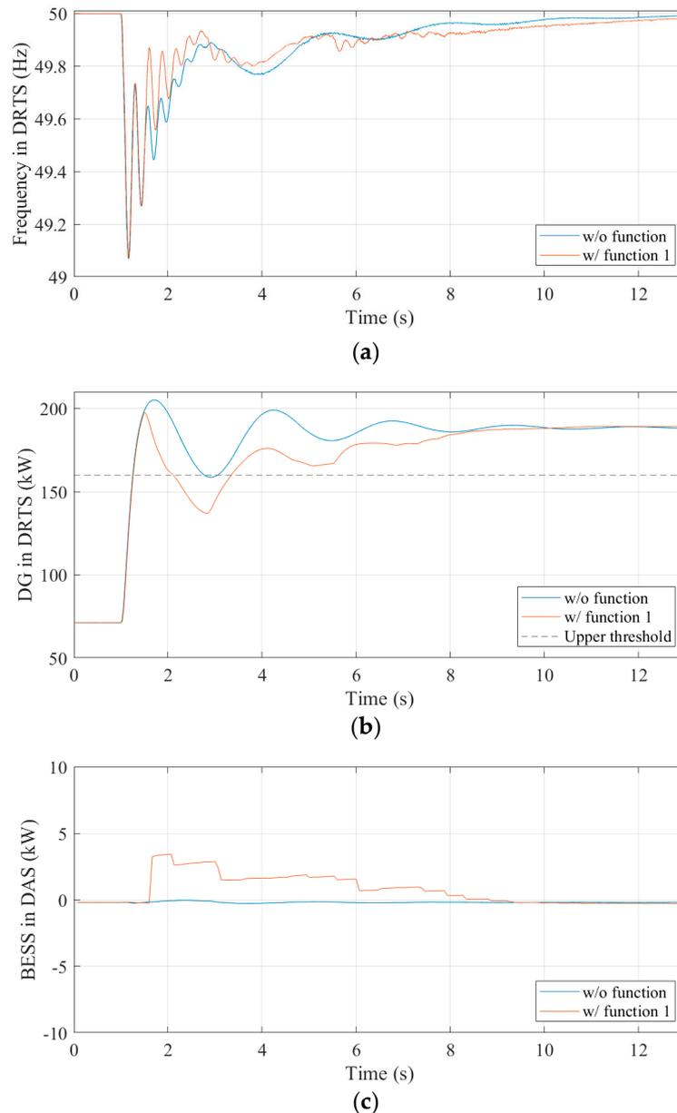
**Figure 6.** Function 1 results (load increase from 7 kW to 19 kW): (a) frequency; (b) DG set output; (c) BESS output. Note that 10 times scaled measurement of actual lab equipment output, i.e., BESS and load, is fed back to the DRTS in this PHIL simulation.
