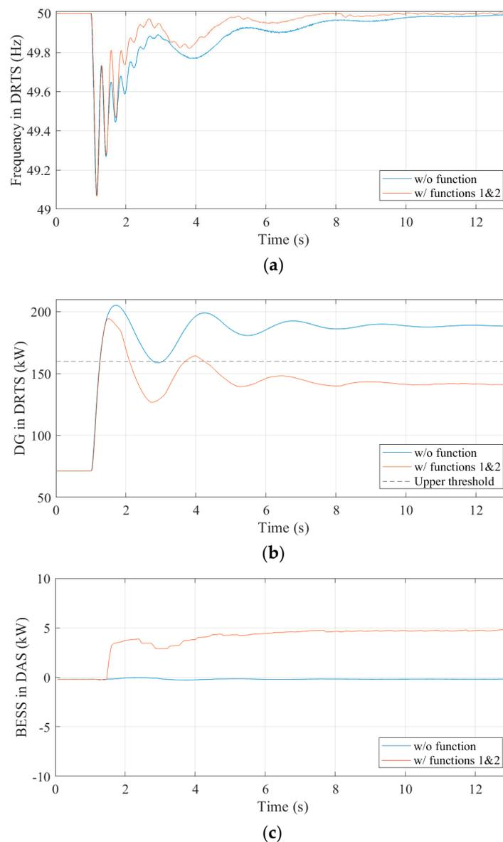
**Figure 8.** Test results when functions 1 and 2 are activated (load increase from 7 kW to 19 kW): (a) frequency; (b) DG set output; (c) battery output. Note that 10 times scaled measurement of actual lab equipment output, i.e., BESS and load, is fed back to the DRTS in this PHIL simulation.
