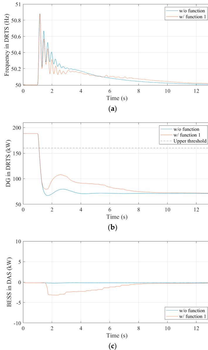
**Figure 7.** Function 1 test results (load reduction from 19 kW to 7 kW): (a) frequency; (b) DG set output; (c) BESS output. Note that 10 times scaled measurement of actual lab equipment output, i.e., BESS and load, is fed back to the DRTS in this PHIL simulation.
