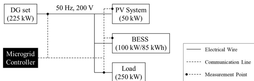
**Figure 4.** Microgrid configuration. The microgrid controller follows outputs of diesel generator (DG) set, battery energy storage system (BESS), photovoltaic (PV), and load and commands to PV and BESS according to functions 1 and 2.
