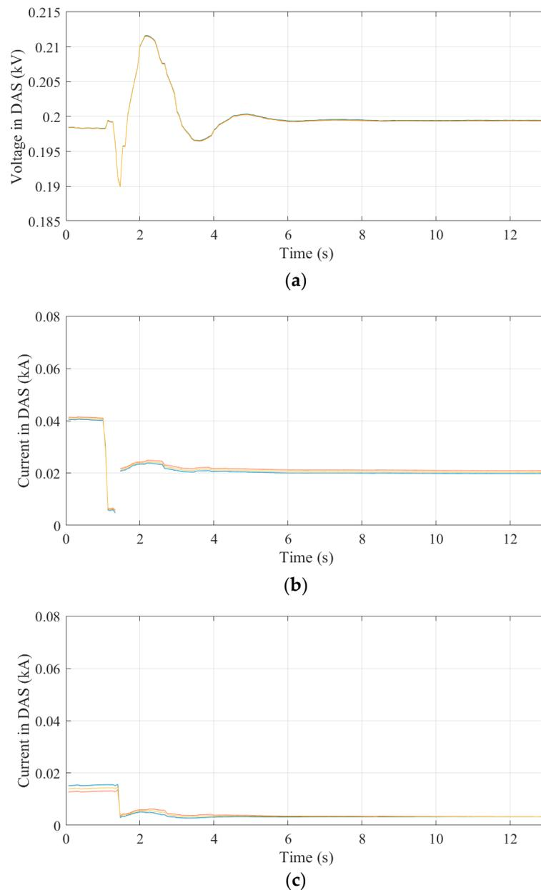
**Figure A2.** Test results when functions 1 and 2 are activated (load reduction from 19 kW to 7 kW): (a) line-to-line bus voltages; (b) line currents of DG set; (c) line currents of BESS.
