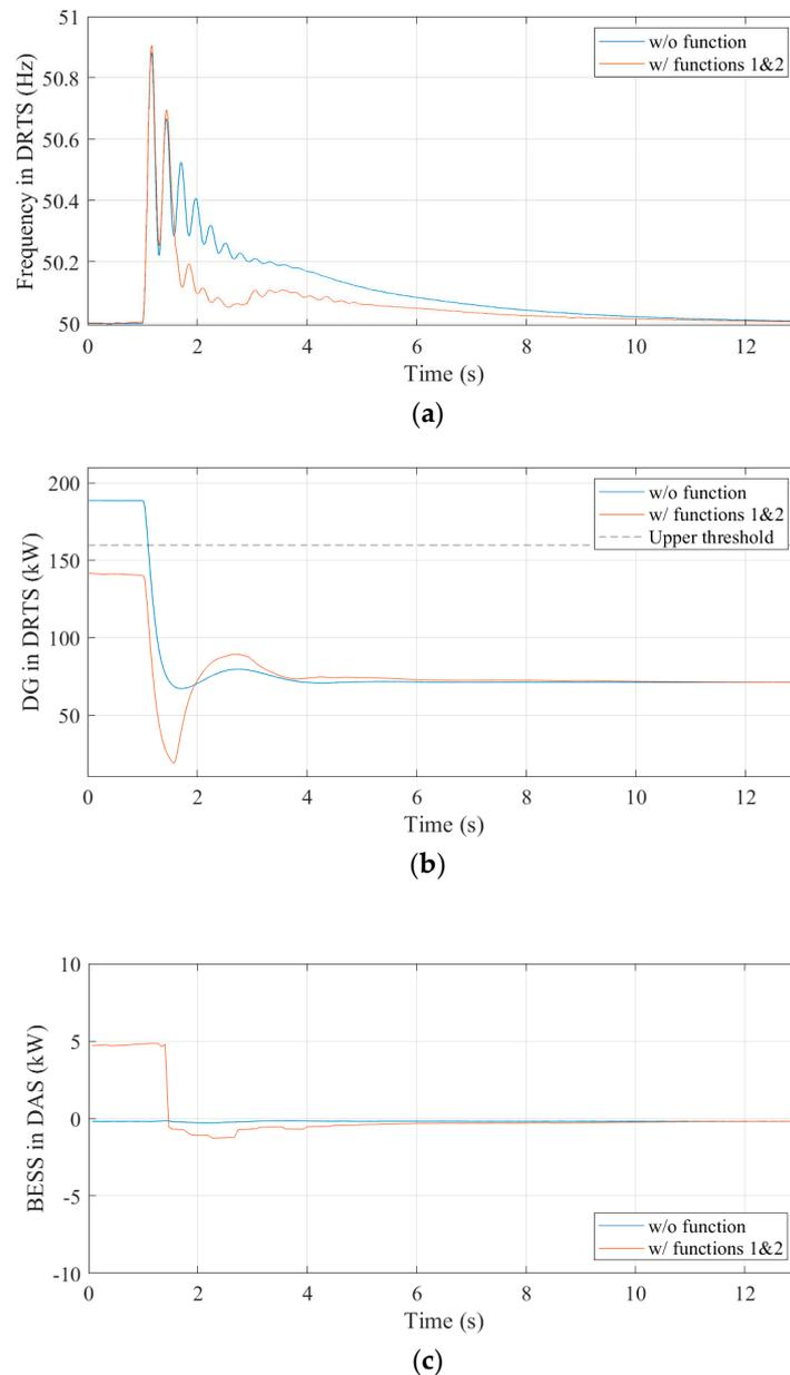
**Figure 9.** Test results when functions 1 and 2 are activated (load reduction from 19 kW to 7 kW): (a) frequency; (b) DG set output; (c) battery output. Note that 10 times scaled measurement of actual lab equipment output, i.e., BESS and load, is fed back to the DRTS in this PHIL simulation.
