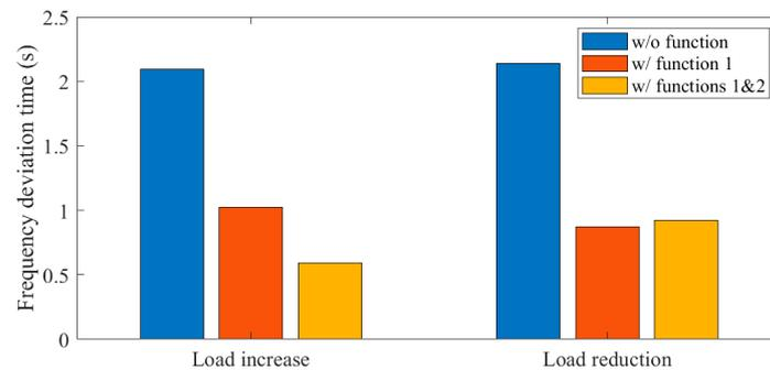
**Figure 10.** Time duration that frequency deviation from the nominal frequency 50 Hz is larger than 0.2 Hz.
