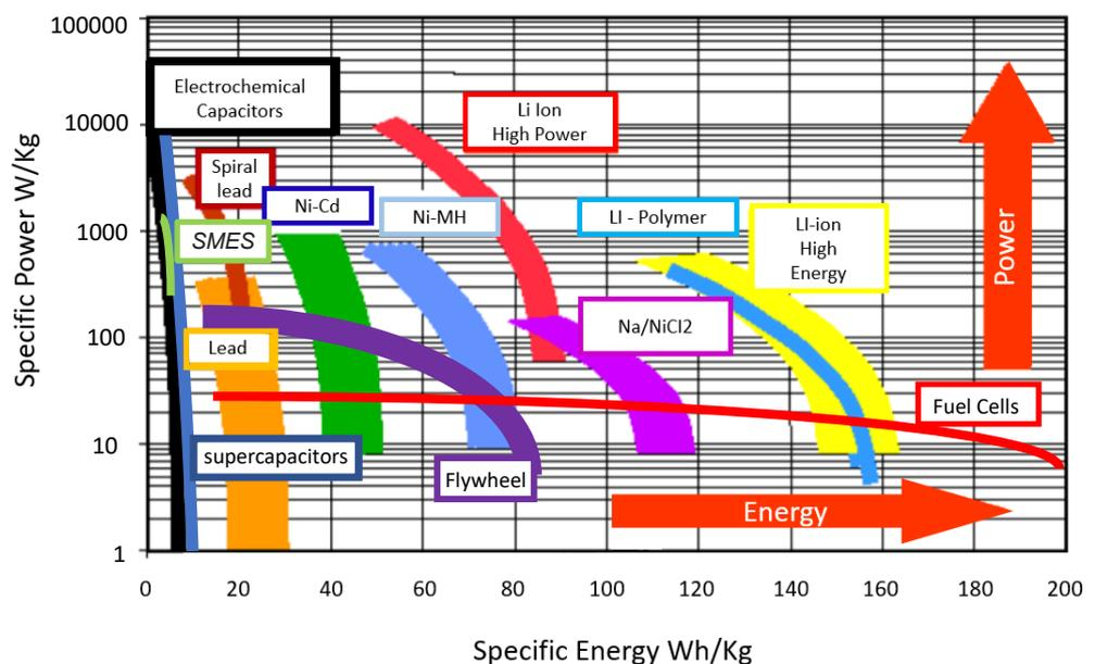
Figure 4. Ragone plot showing specific energy versus specific power for various energy-storing devices [52].
