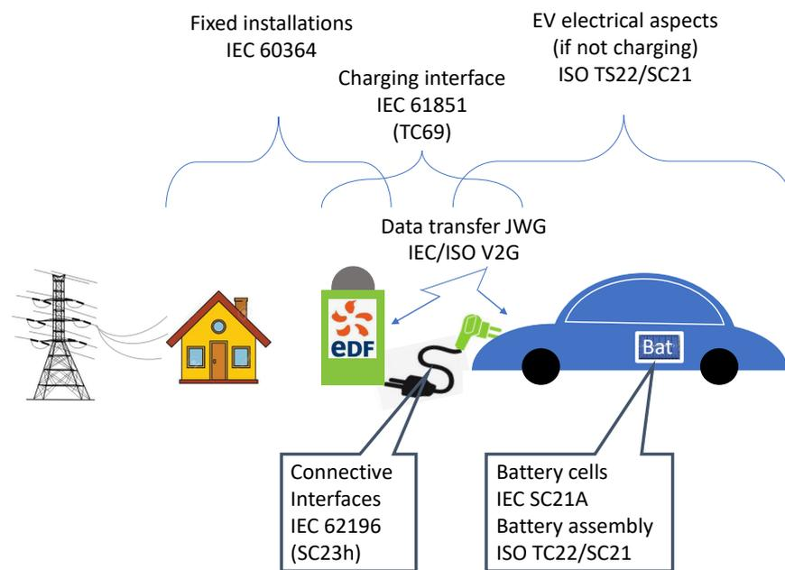
**Figure 9.** Diagram of the standards surrounding the connection of the EV to the electrical grid [83].
