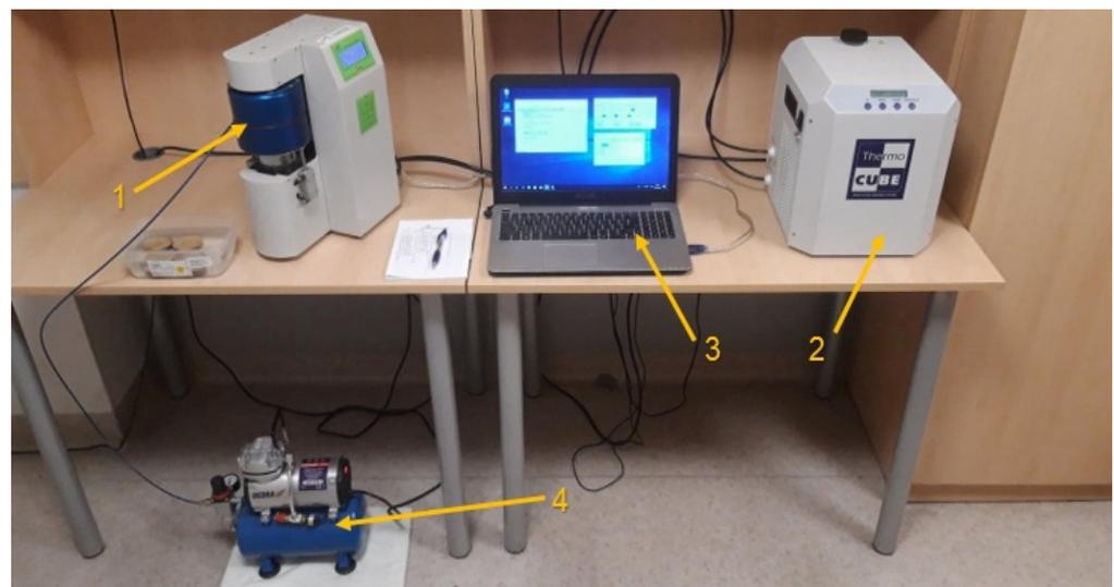
**Figure 2.** Measuring station, 1—FOX 50 Lambdameter by TA Instruments, 2—ThermoCube 200–500 thermoelectric recirculation cooler by Solid State Cooling System, 3—laptop with Win Therm50v2 software, 4—DED7472 compressor by Dedra.
