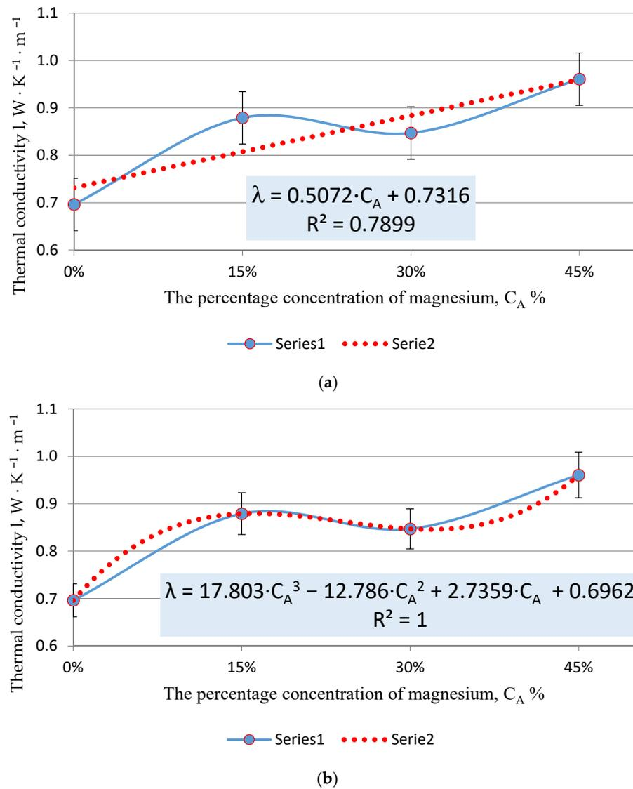
**Figure 5.** The influence of magnesium shavings concentration on the average thermal conductivity values: (a) trend line as a linear function, (b) trend line as a polynomial function; Series 1—graph based on the measurement results, Serie 2—trend line.
