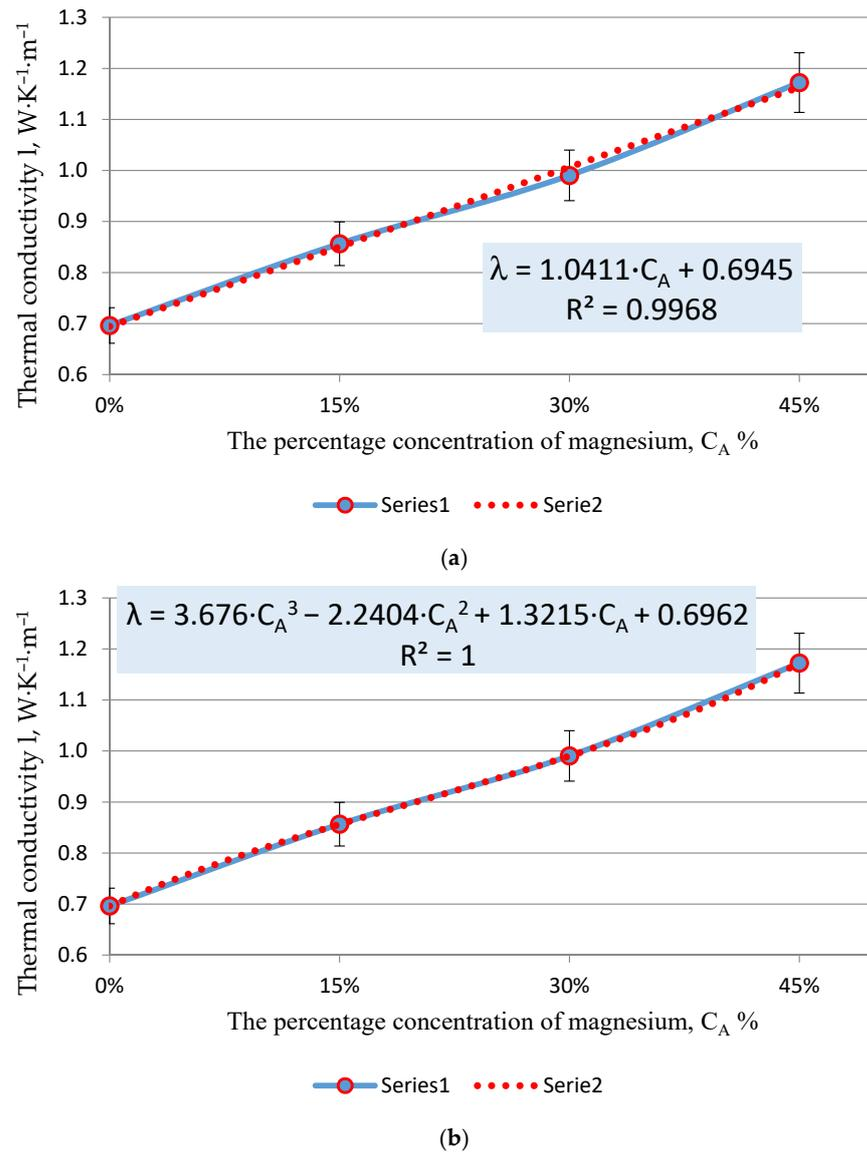
**Figure 4.** The influence of the magnesium flakes concentration on the sample's average thermal conductivity values: (a) trend line as a linear function, (b) trend line as a polynomial function; Series 1—graph based on the measurement results, Serie 2—trend line.
