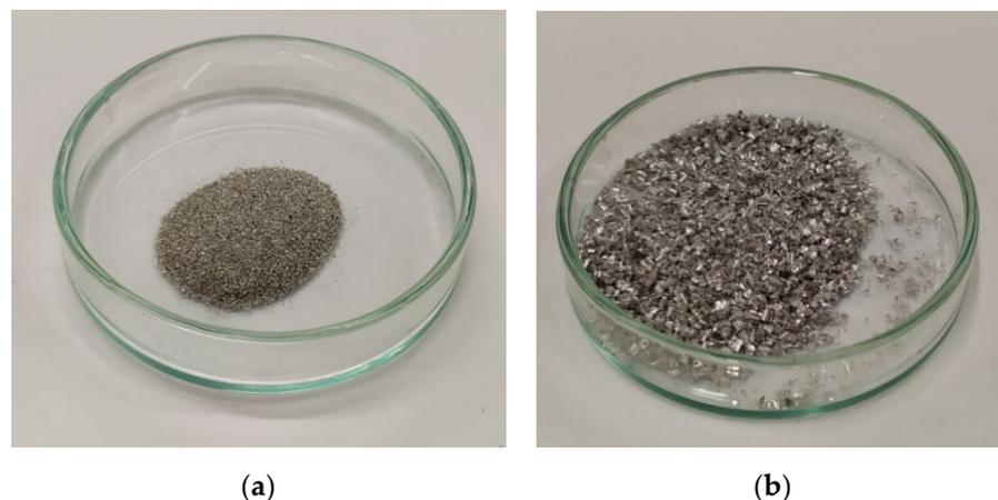
**Figure 1.** (a) magnesium in flakes with a granulation  $<0.25 \text{ mm}$ , (b) magnesium in shavings.
