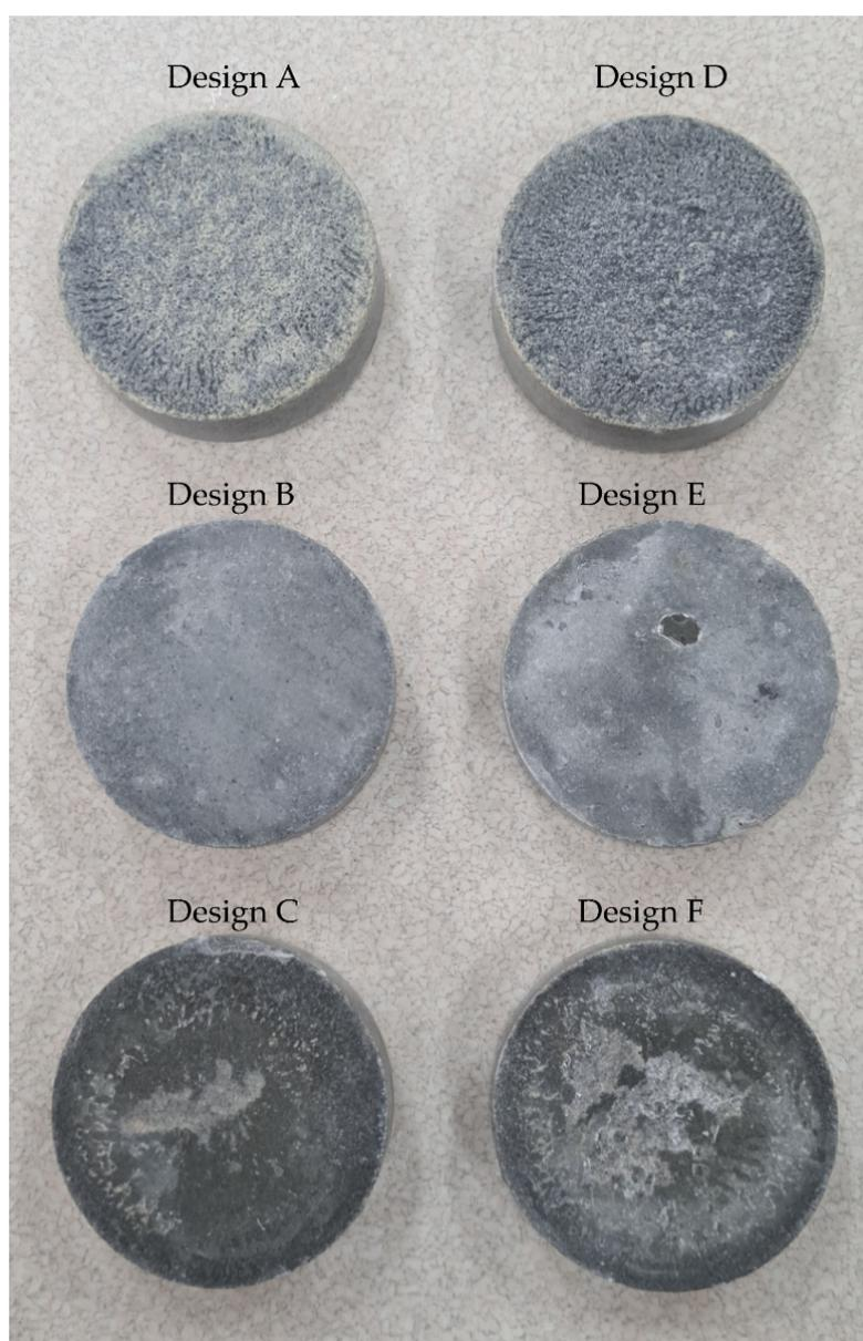
Figure 3. Sample prepared for thermal conductivity tests.
