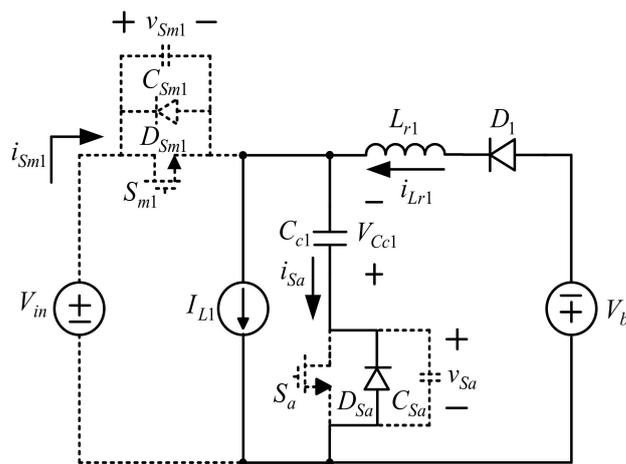
Figure 9. First-stage current flow in state 5.
