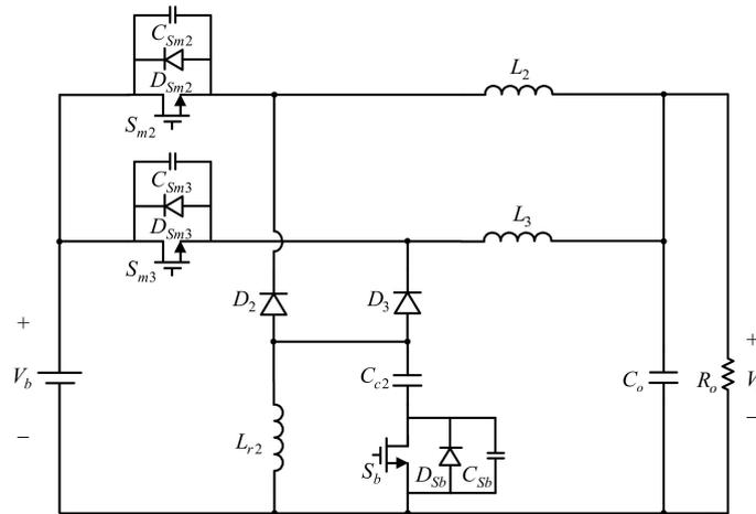
Figure 14. Two-phase interleaved buck converter with active clamp.
