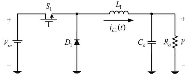
Figure 24. Traditional buck converter.
