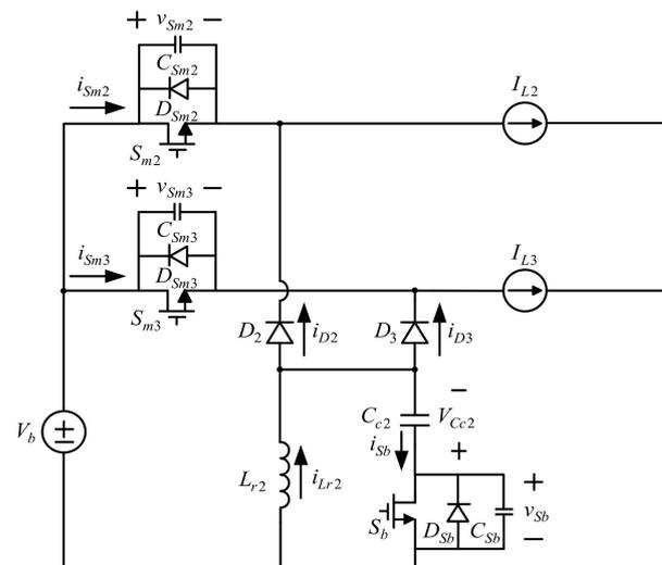
Figure 15. Equivalent circuit for the circuit shown in Figure 14.
