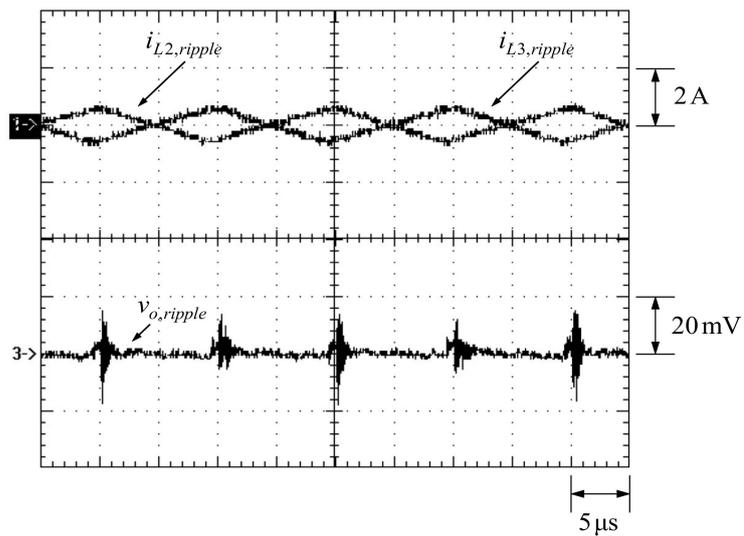
Figure 39. Current ripples of two phases,  $i_{L2,ripple}$  and  $i_{L3,ripple}$ , and output voltage ripple  $v_{o,ripple}$ .
