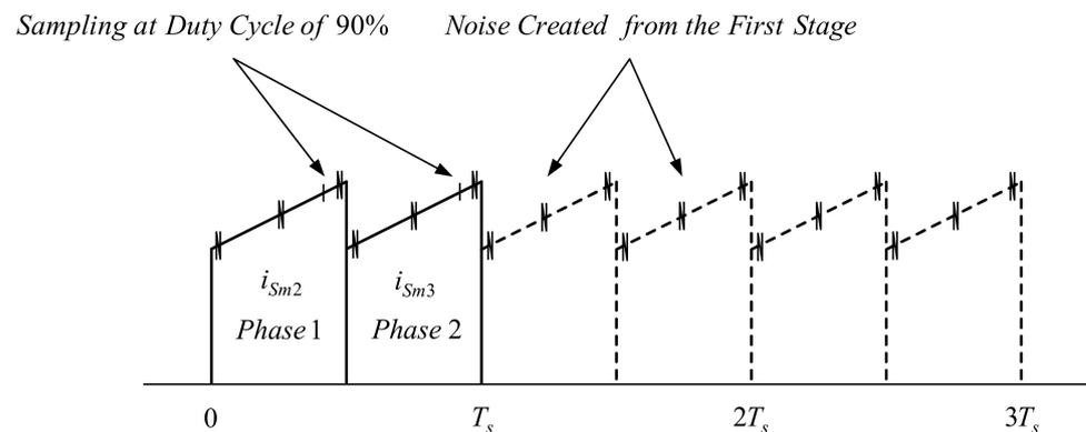
**Figure 31.** Proposed sampling method for current sharing.
