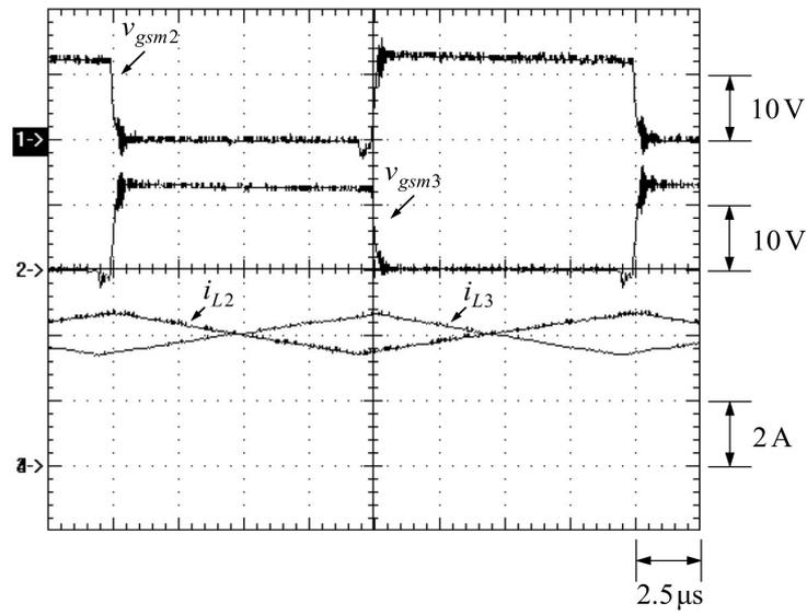
Figure 38. Gate driving signals  $v_{gsm2}$  and  $v_{gsm3}$  and inductor currents  $i_{L2}$  and  $i_{L3}$  of two phases.
