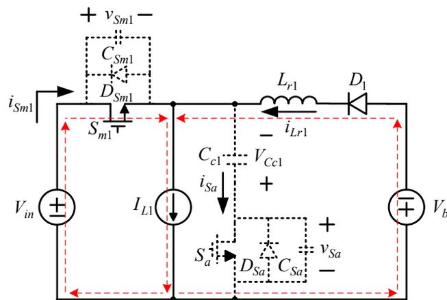
Figure 6. First-stage current flow in state 2.
