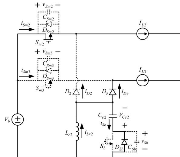
Figure 19. Second-stage current flow in state 3.
