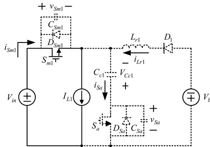
Figure 7. First-stage current flow in state 3.
