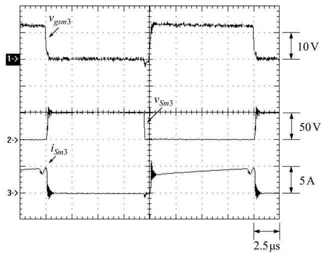
Figure 36. ZVS turn-on of  $S_{m3}$  of the first phase.
