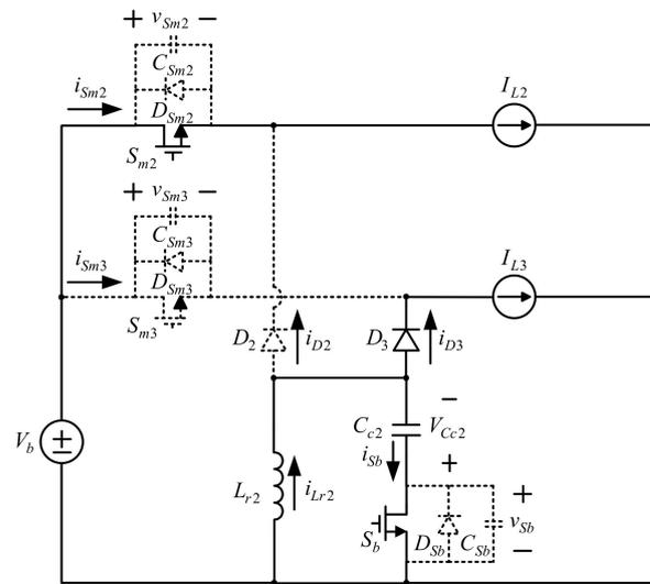
Figure 21. Second-stage current flow in state 5.
