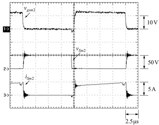
Figure 35. ZVS turn-on of  $S_{m2}$  of the first phase.
