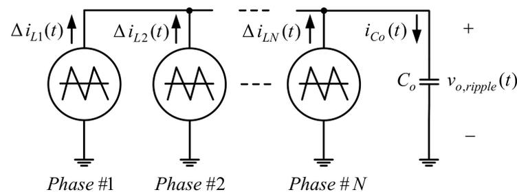
Figure 28. Equivalent circuit for the output voltage ripple of the  $N$ -phase interleaved buck converter.
