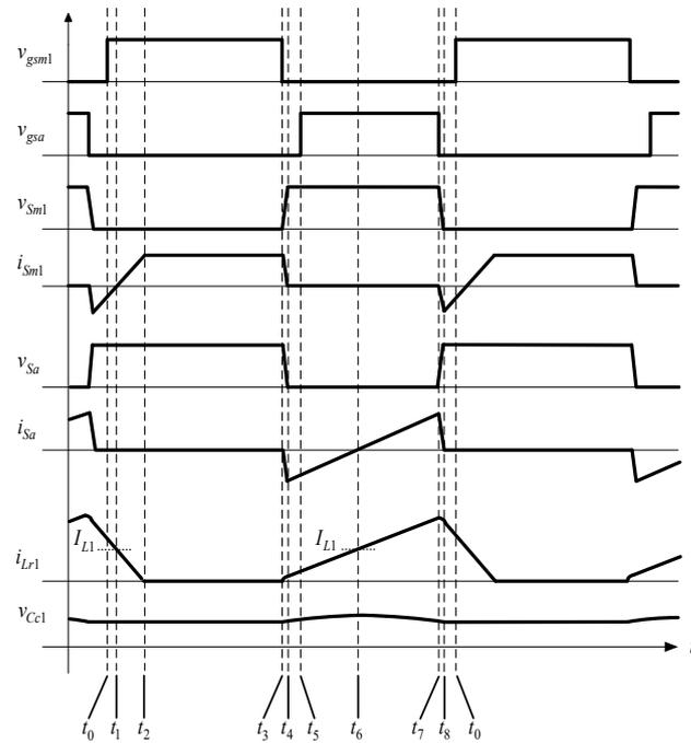
Figure 4. Illustrated waveforms for the buck-boost converter with active clamp.
