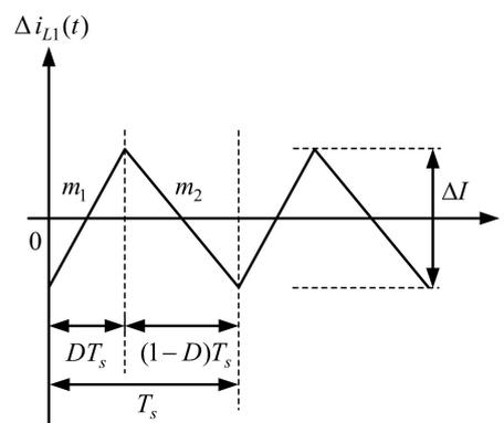
Figure 26. AC part of the inductor current.
