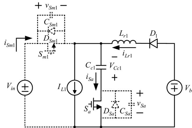
Figure 10. First-stage current flow in state 6.
