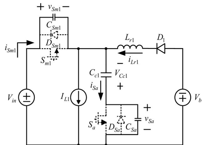
Figure 12. First-stage current flow in state 8.
