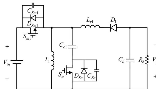
Figure 2. Buck-boost converter with active clamp.
