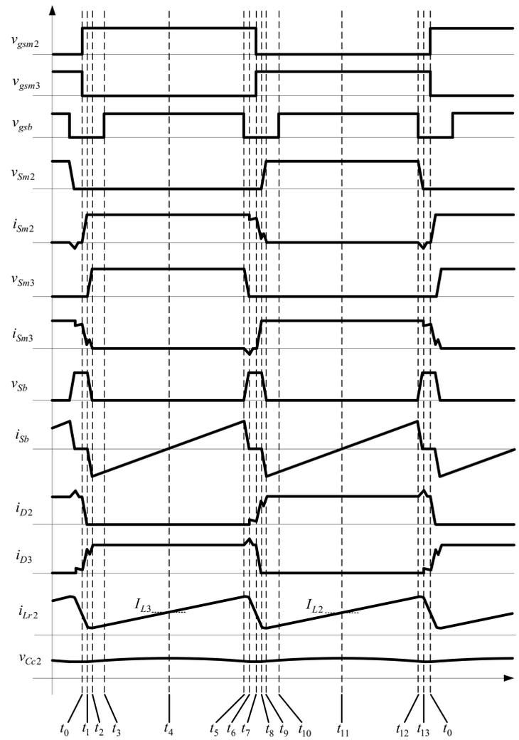
Figure 16. Illustrated waveforms for the two-phase interleaved buck converter with active clamp.
