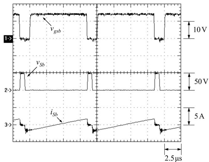
Figure 37. ZVS turn-on of  $S_b$ .
