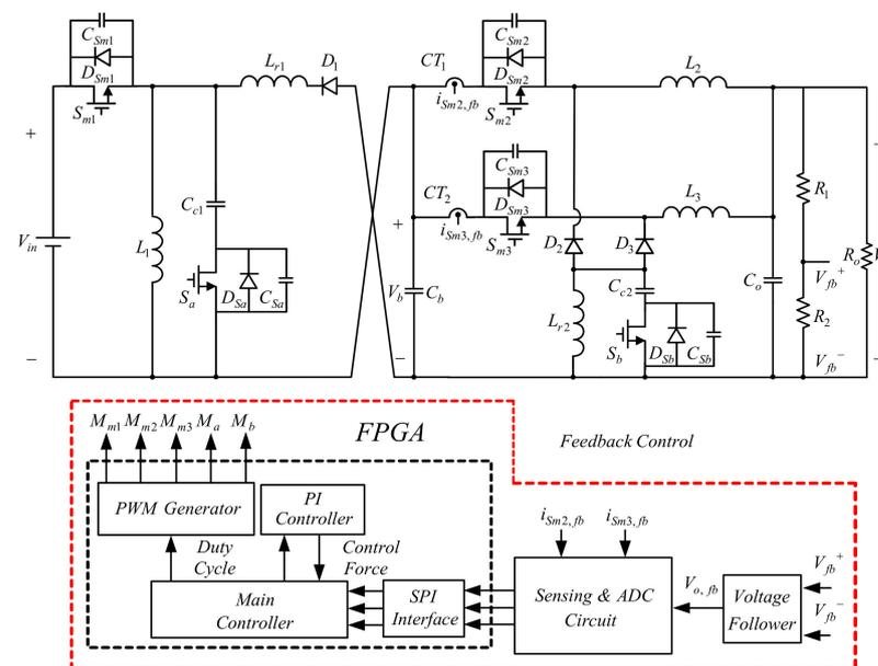
Figure 1. System configuration.
