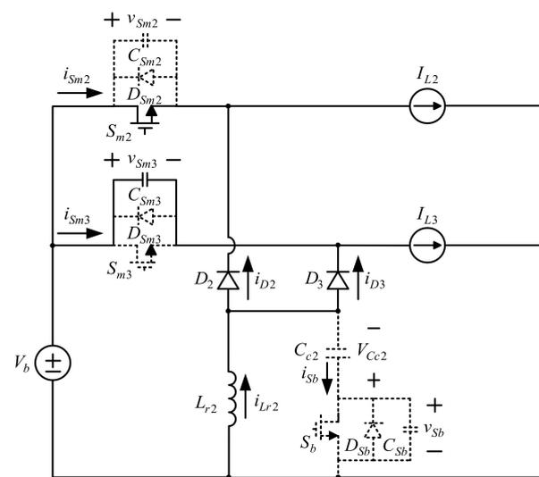
Figure 17. Second-stage current flow in state 1.
