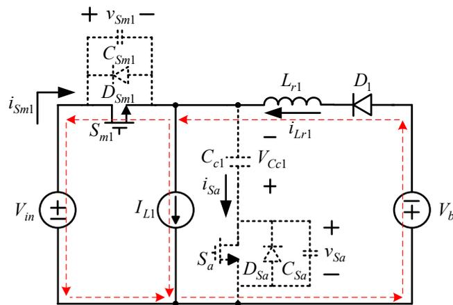
Figure 5. First-stage current flow in state 1.
