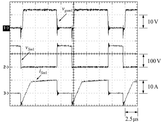
Figure 33. ZVS turn-on of  $S_{m1}$ .
