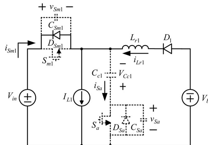
Figure 13. First-stage current flow in state 9.
