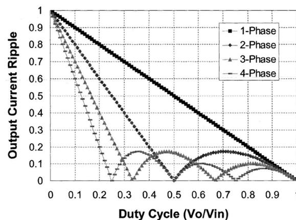
Figure 29. Curves for relationship between phase number, duty cycle, and output current ripple.
