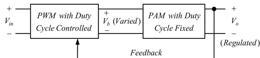
Figure 30. Schematic diagram for the control strategy based on PAM cooperated with PWM.
