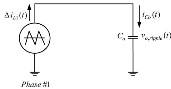
Figure 27. Equivalent circuit for the output voltage ripple.
