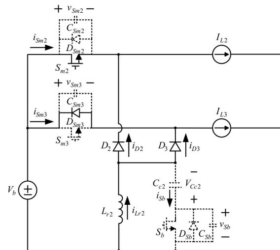
Figure 23. Second-stage current flow in state 7.
