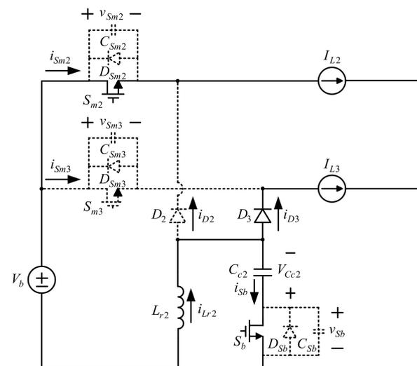
Figure 20. Second-stage current flow in state 4.
