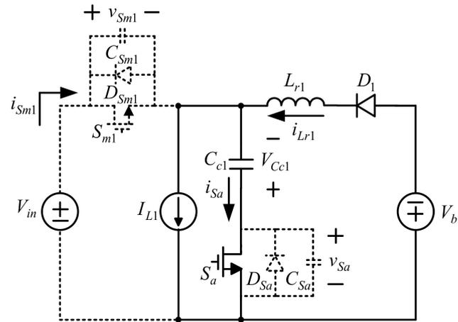
Figure 11. First-stage current flow in state 7.
