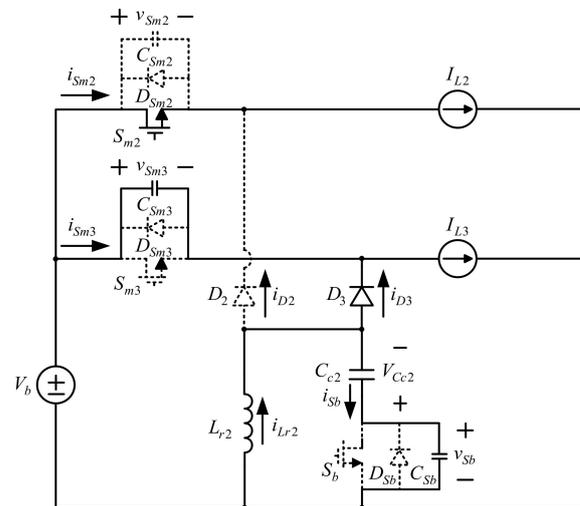
Figure 22. Second-stage current flow in state 6.
