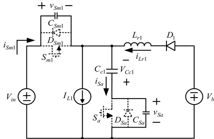
Figure 8. First-stage current flow in state 4.
