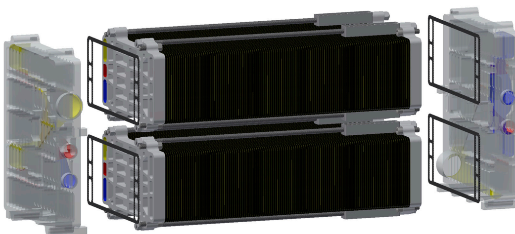
Figure 4. Connection of both stacks ( middle ) with the developed manifolds ( left, right ) for educt distribution and collection.
