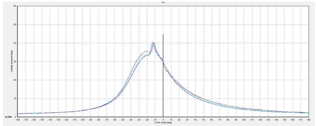
Figure 17. In-cylinder pressure curves obtained with the MarPrime software at 50% load (36 kVA).
