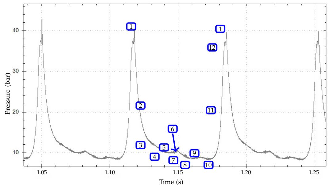
Figure 18. In-cylinder pressure curve obtained with the proposed sensor at 50% load (36 kVA).
