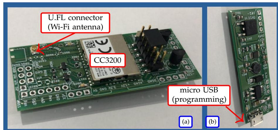
Figure 10. Microcontroller board (Wi-Fi, analog, and GPIOs)—(a) top layer—(b) bottom layer.
