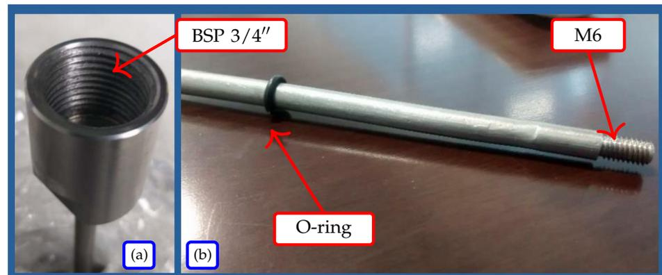
**Figure 5.** Adaptation tube for in-cylinder pressure measurement—(a) zoom on the BSP 3/4'' thread (where the Thompson valve is inserted)—(b) tube with male M6 thread (which is inserted at the combustion chamber).
