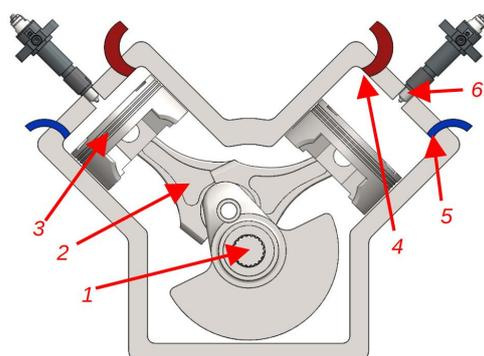
**Figure 1.** Representation of combustion engine with cylinders in “V” (such as the Wärtsilä 18V46). From [22].
