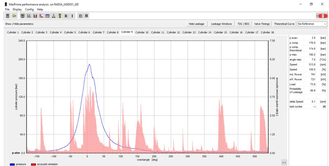
Figure 27. Ultrasound noise at valves monitoring—screen capture of the Marprime Ultra software.
