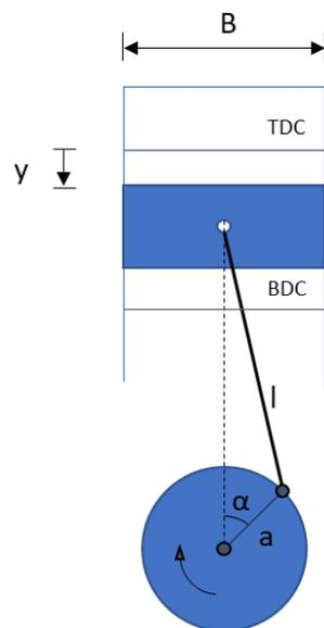
**Figure 2.** Crank geometry of a cylinder. Developed from [23].
