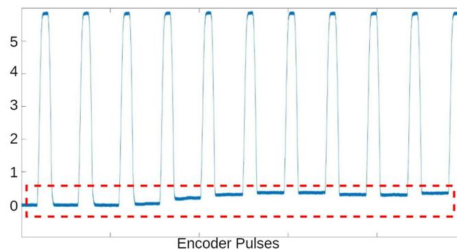
**Figure 31.** Inlet valve position, measured with the proposed resistive sensor—Loose Valve Clearance.
