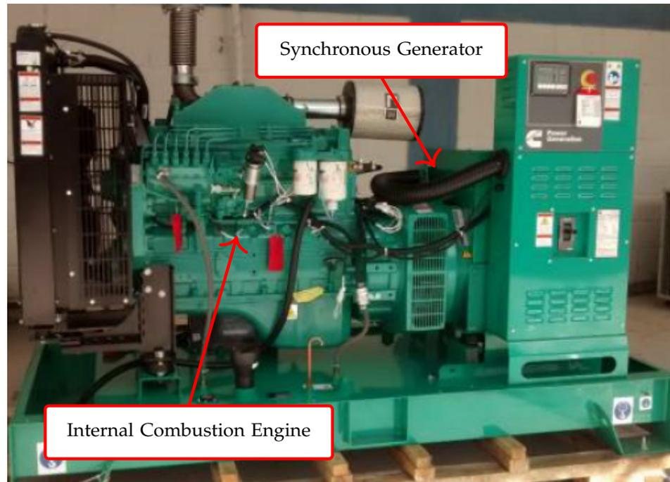
**Figure 4.** Unmodified diesel generator of the reduced scale laboratory.
