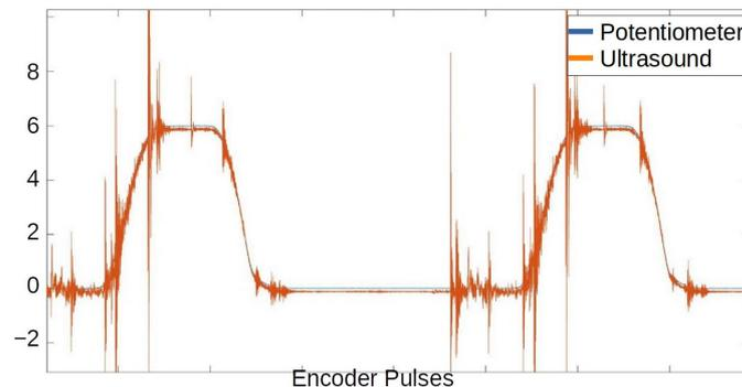
Figure 28. Comparison between Ultrasound and proposed Rocker Arm sensor based on Potentiometer.
