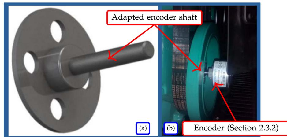
**Figure 8.** Adaptation of the encoder to the crankshaft pulley—(a) 3D concept of the adapter—(b) actual photograph.
