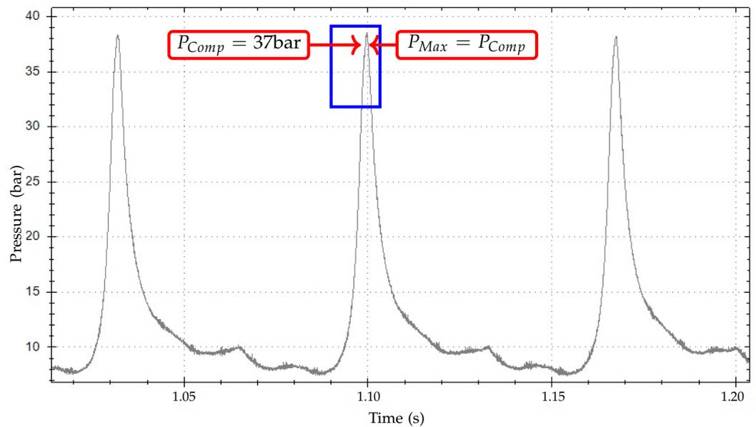
**Figure 21.** In-cylinder pressure curve obtained with the proposed sensor at 50% load (36 kVA) with fuel injection failure.
