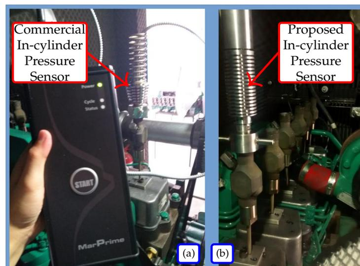
Figure 16. In-cylinder pressure sensors installed at the reduced scale laboratory—(a) commercial system—(b) proposed system.
