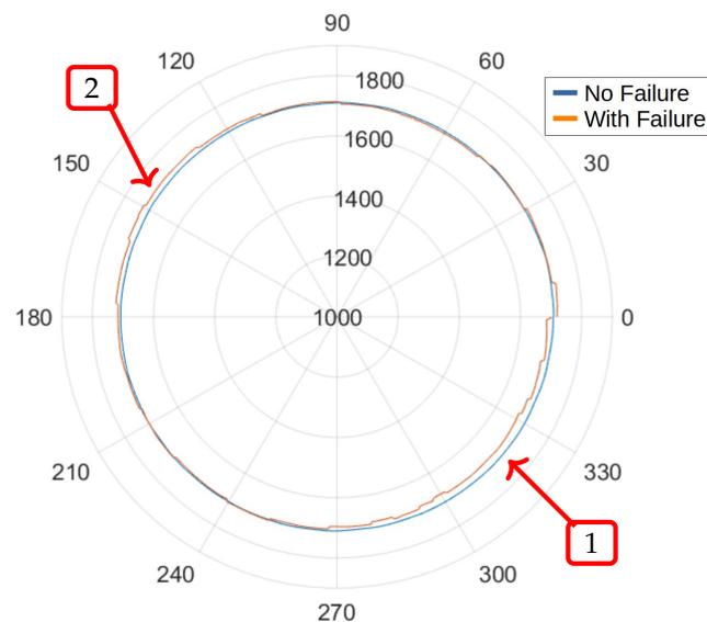
**Figure 24.** Instantaneous velocity measured with the proposed sensor—50% Load-Fuel Injection Failure.
