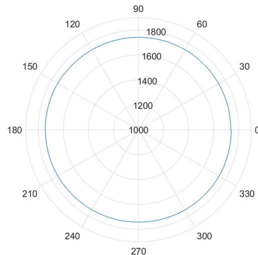
**Figure 22.** Instantaneous velocity measured with the proposed sensor—No Load-No Failures.
