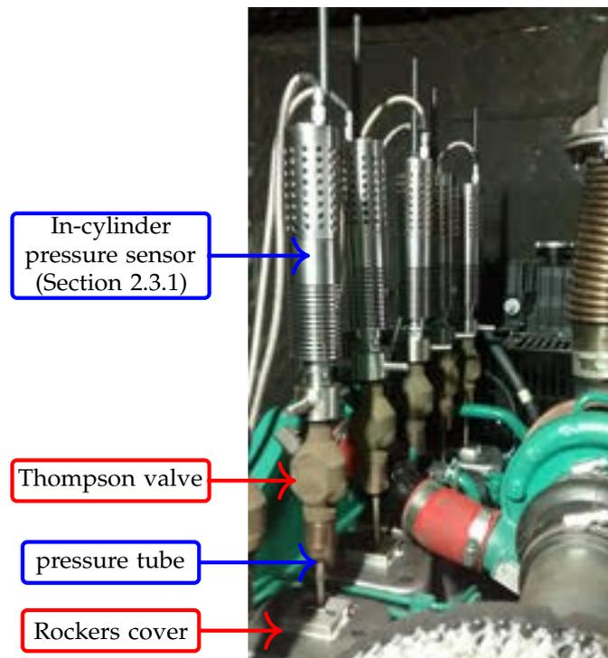
**Figure 7.** In-cylinder pressure sensors attached to the Thompson valves.
