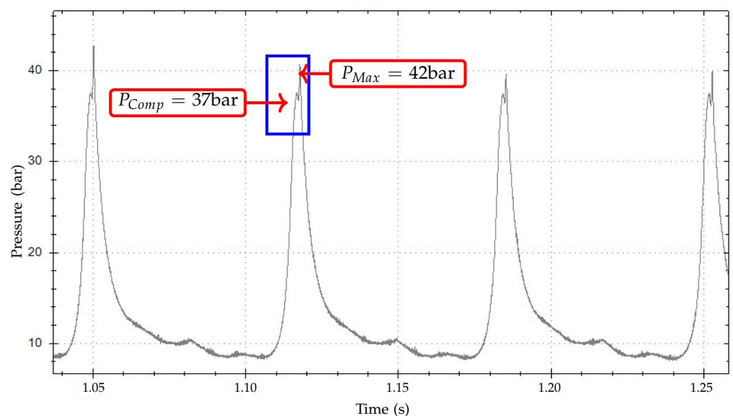
Figure 20. In-cylinder pressure curve obtained with the proposed sensor at 50% load (36 kVA) without failures.
