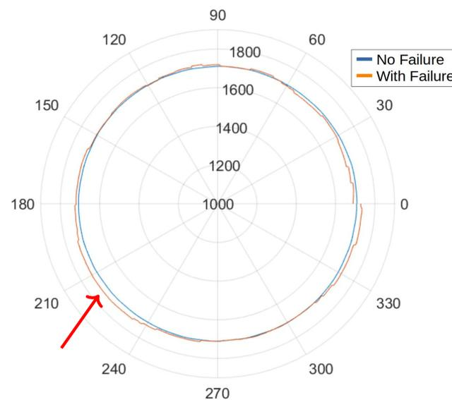
**Figure 26.** Instantaneous velocity measured with the proposed sensor—50% Load-Loose Clearance of Inlet Valve Failure.
