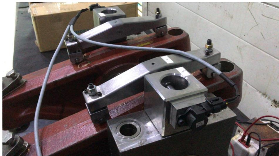
**Figure 14.** Resistive sensors installed at the rocker arms.
