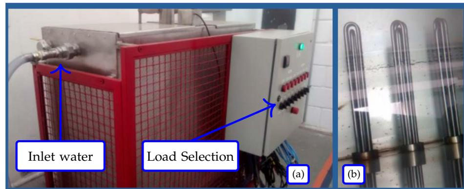
Figure 15. Variable load—(a) general view—(b) resistors immersed in water.
