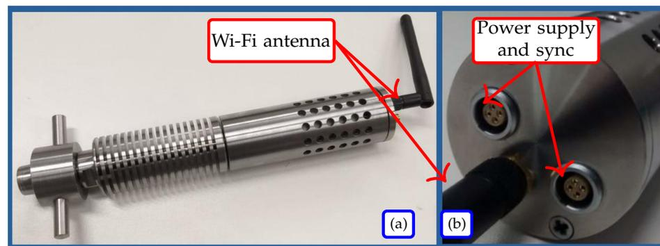
**Figure 11.** Proposed In-Cylinder pressure sensor with Wi-Fi connectivity—(a) general view—(b) zoom of the top part of the sensor.
