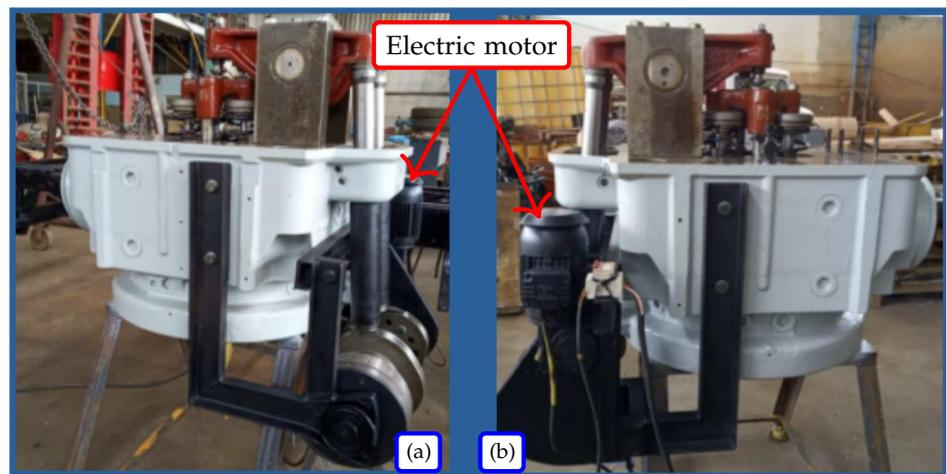
**Figure 13.** 1/18 of Wärtsilä 18v46 Cylinder Head with adapted electric motor at the crankshaft—(a) left view—(b) right view.
