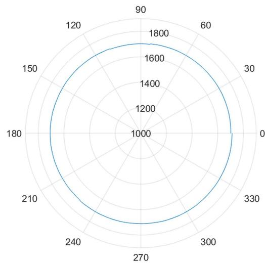
**Figure 23.** Instantaneous velocity measured with the proposed sensor—50% Load-No Failures.
