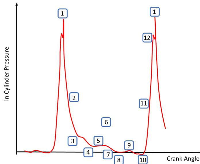
**Figure 3.** Variation of in-cylinder pressure in relation to the crank angle.
