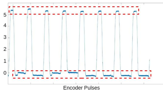
**Figure 30.** Inlet valve position, measured with the proposed resistive sensor—Tight Valve Clearance.
