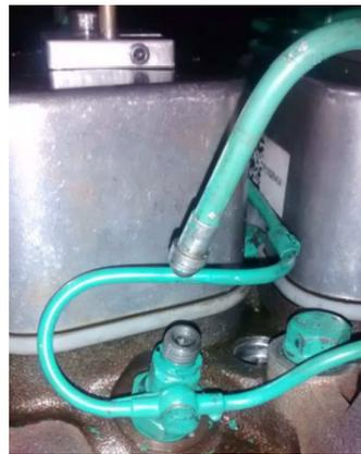
Figure 19. Simulated failure at the fuel injection of Cylinder 06.
