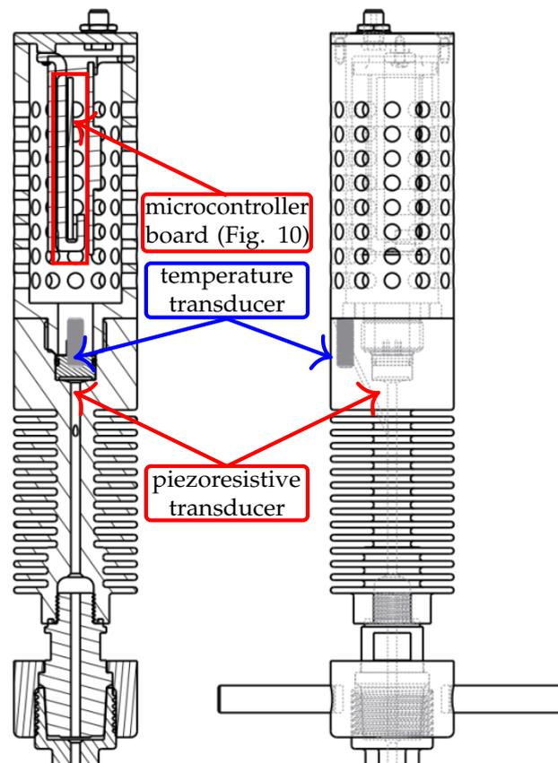
Figure 9. Conceptual drawing of the sensor housing.
