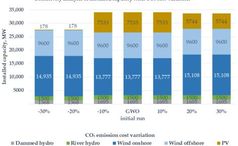
Sensitivity analysis of installed capacity with CO2 cost variation
