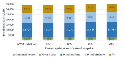
Sensitivity analysis of RES capacity with natural gas cost icrease
