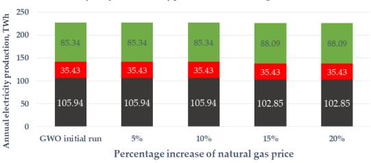
Sensitivity analysis of electricity production with natural gas cost icrease
