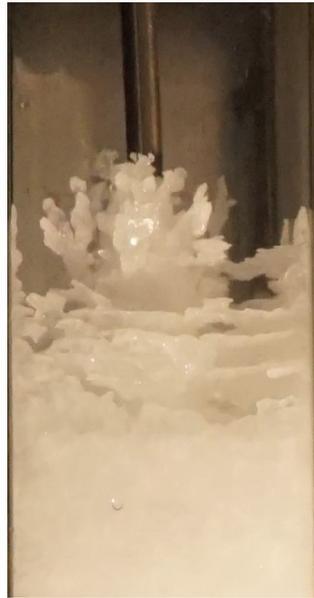
**Figure 6.** PCM solidification along the immersed nozzle.
