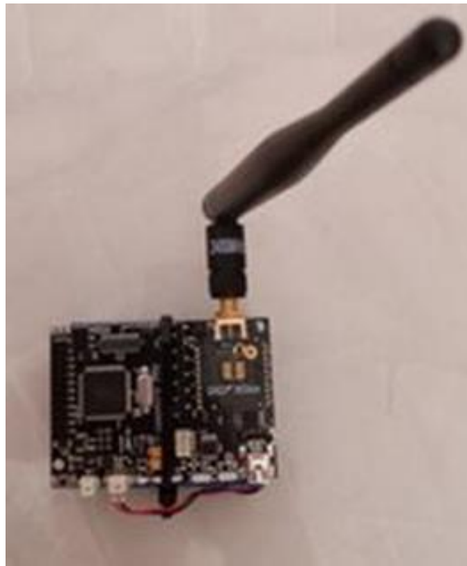
Figure 14. Wasp mote device equipped with the 802.15.4 module.
