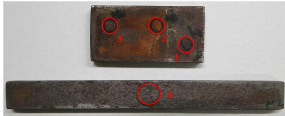
**Figure 8.** Topography studies of surface in Figure 7, microstructure and chemical composition of the top layer as well as the microstructure of the corroded sample, pressure-conditioned at 80 °C.
