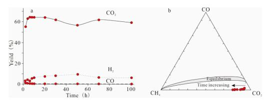
**Figure 3.** The evolution character of inorganic gases (a) during pyrolysis of oil shale with time series; (b) CH<sub>4</sub>-CO<sub>2</sub>-CO diagram (modified from [21]); the gray field represents the thermodynamic equilibrium of CH<sub>4</sub>-CO<sub>2</sub>-CO gases.
