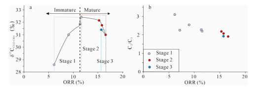
**Figure 7.** Evolution characteristics of  $\delta^{13}C_{CO_2-CH_4}$  with ORR at time series (a) and plot of  $C_2/C_3$  with ORR (b).
