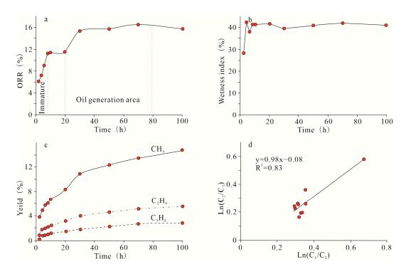
**Figure 2.** The evolution characteristics of ORR (**a**) wetness (**b**) and organic gases (**c**) during the pyrolysis of oil shale with time series; (**d**) the plots of  $\ln(C_1/C_2)$  versus  $\ln(C_2/C_3)$  for gas products.
