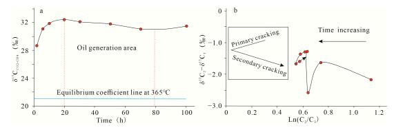
**Figure 5.** Carbon isotope fractionation coefficient between  $CO_2$  and  $CH_4$  (a) and plots of  $ln(C_2/C_3)$  versus  $\delta^{13}C_2$ - $\delta^{13}C_3$  (b) from time-series pyrolysis experiments. The calculated equilibrium coefficient at 365 °C was based on the study [29]; "b" is modified from [47].
