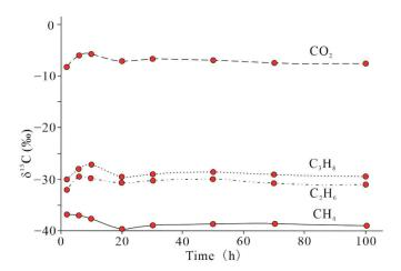
Figure 4. Stable carbon isotope values for CO<sub>2</sub>, CH<sub>4</sub>, C<sub>2</sub>H<sub>6</sub>, and C<sub>3</sub>H<sub>8</sub> with increasing times at 365 °C.
