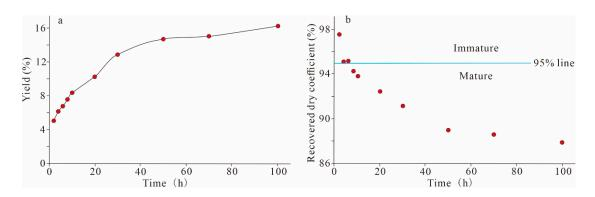
Figure 6. Recovered CH<sub>4</sub> (a) and dry coefficient (b) evolution characteristics with time increasing.
