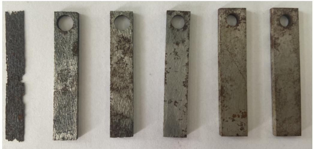
**Figure 8.** Photographs of N80 steel sheet corrosion (left to right: 0%, 0.5%, 0.8%, 1.0%, 1.5%, and 2.0%).
