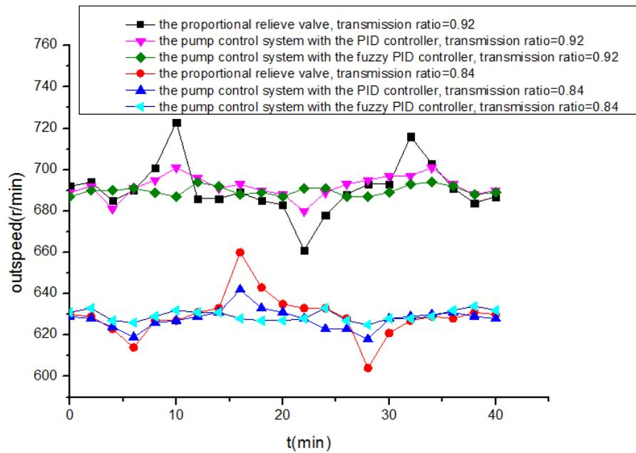
**Figure 12.** Output speed fluctuation of HVC.
