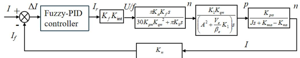
Figure 5. Transfer function block diagram of the new system for HVC.
