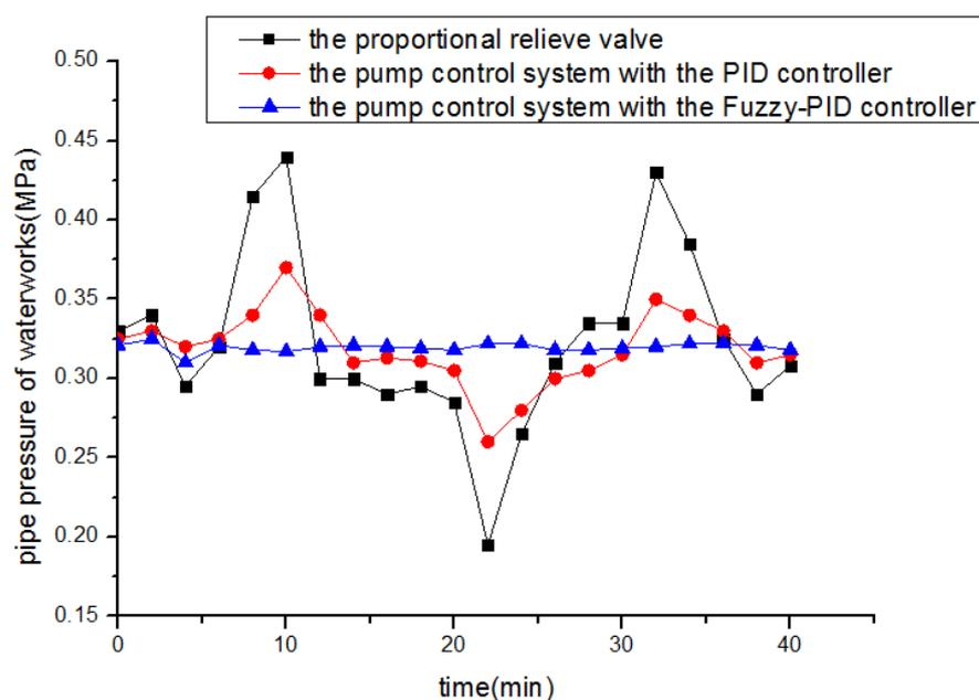
Figure 14. Pipe pressure fluctuation when transmission ratio = 0.92.
