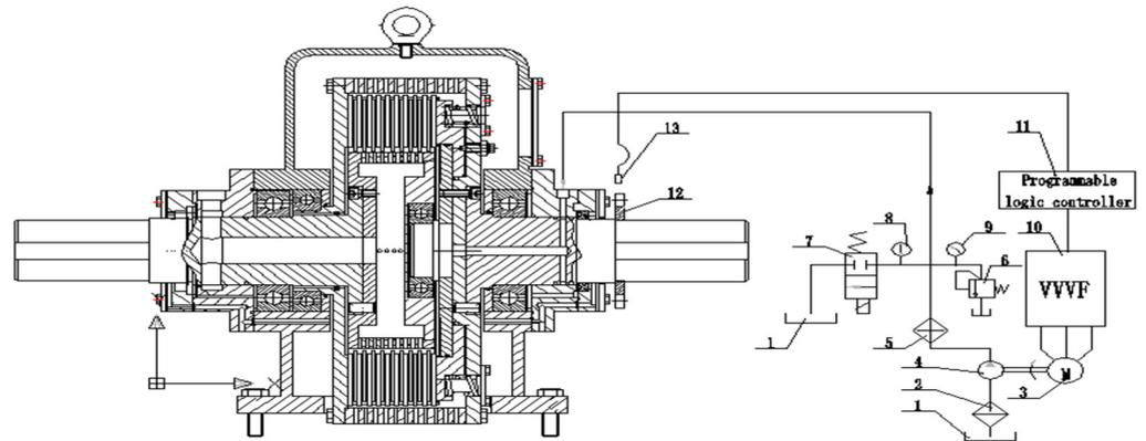
**Figure 3.** New hydraulic pump control system for HVC. 1. Hydraulic oil tank; 2. filter; 3. gear pump motor; 4. gear pump; 5. chiller; 6. safety valve; 7. electromagnetic valve; 8. thermometer; 9. manometer; 10. frequency converter; 11. PLC; 12. measuring speed gear; 13. speed sensor.
