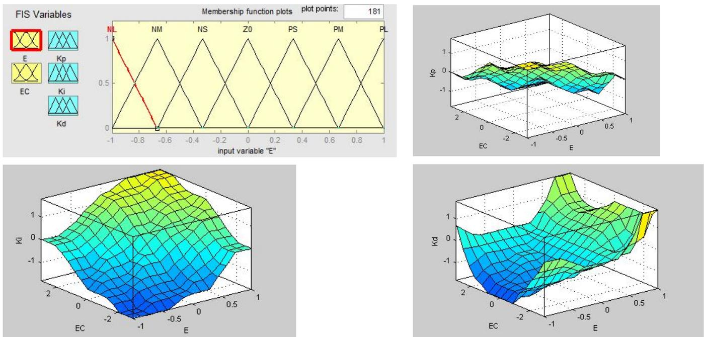
Figure 7. The membership function and surface viewer of the Fuzzy-PID controller.
