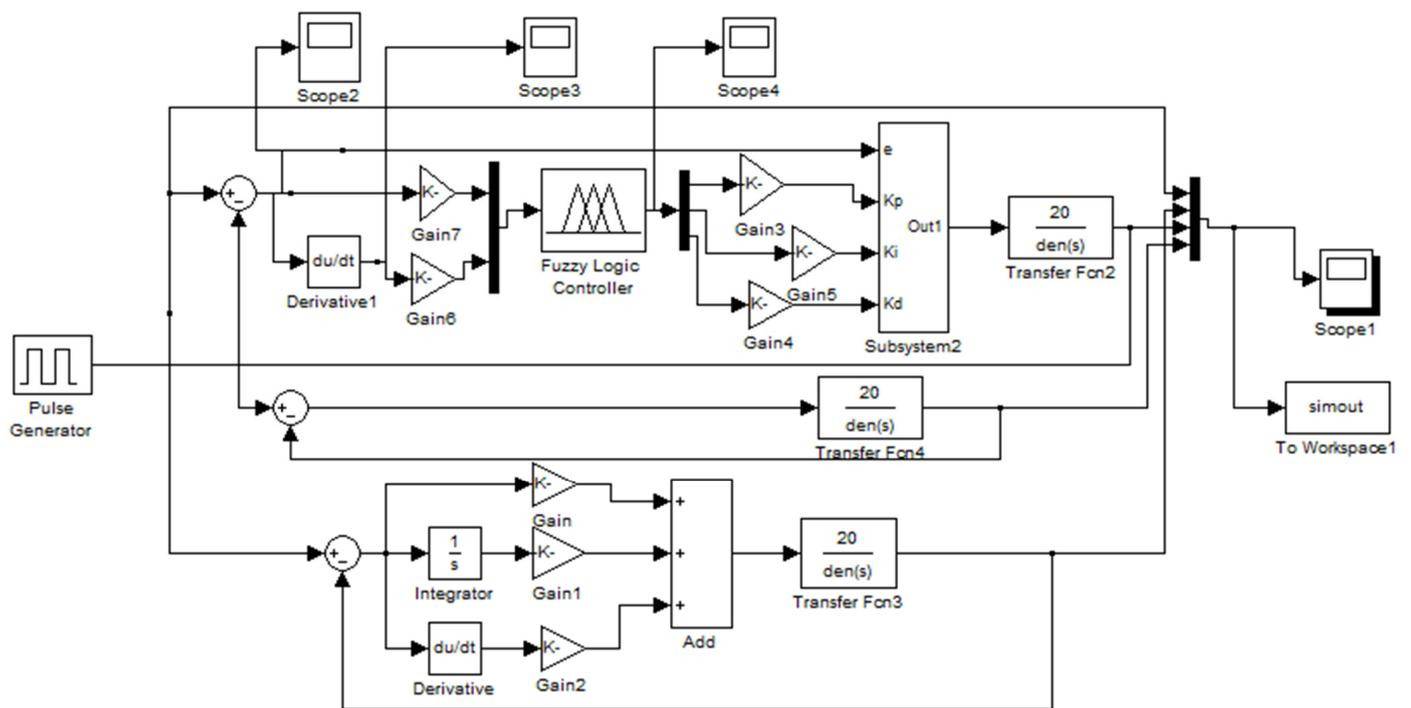
Figure 6. Structural diagram of Fuzzy-PID controller.
