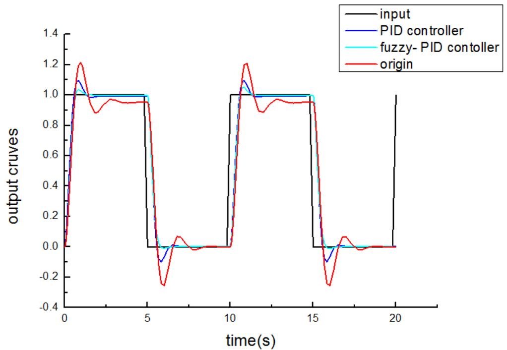
Figure 8. Response curves of different control methods.
