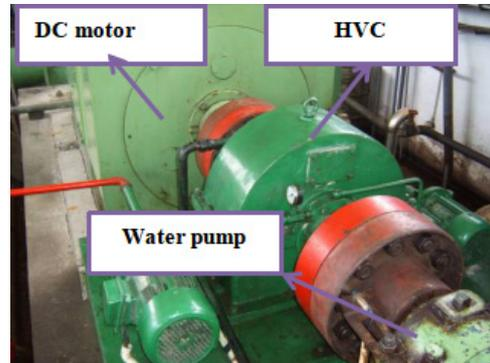
Figure 10. Test field of HVC.
