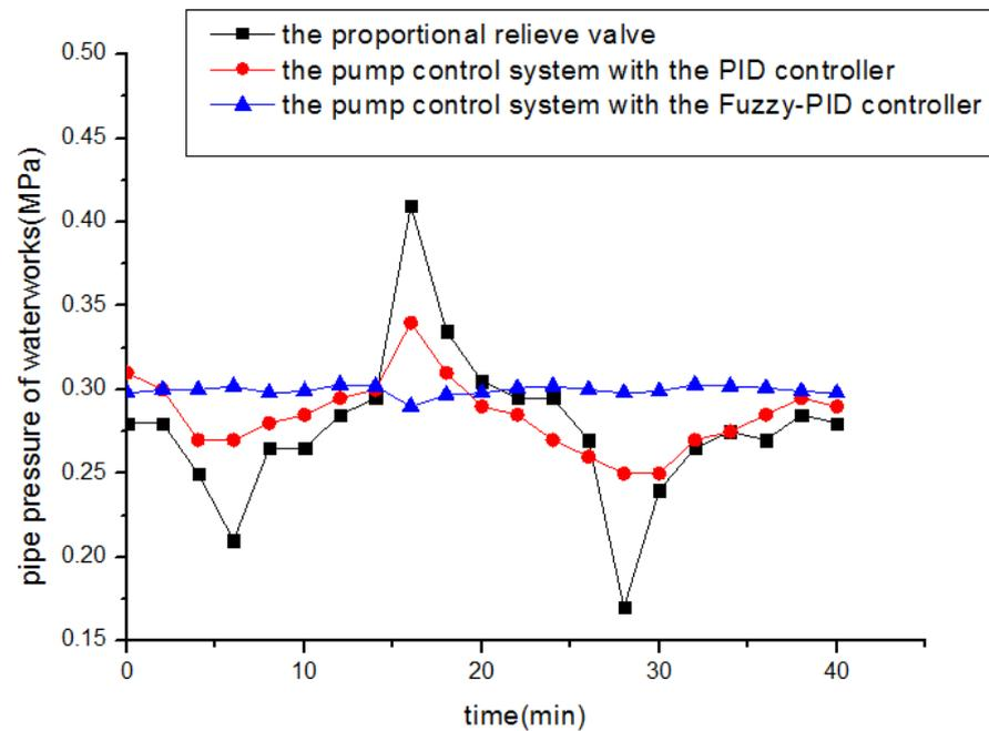
**Figure 13.** Pipe pressure fluctuation when transmission ratio = 0.84.
