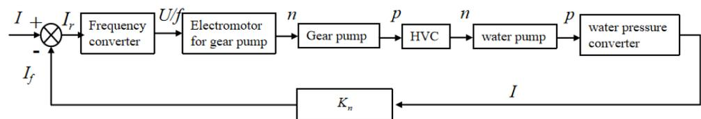
Figure 1. Diagrammatic sketch of HVD control system.
