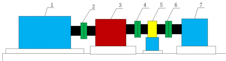
Figure 2. Schematic diagram for the HVD control system. 1. electric motor; 2, 4, 6. flexible coupling; 3. HVC; 5. speed sensor; 7. water pump.
