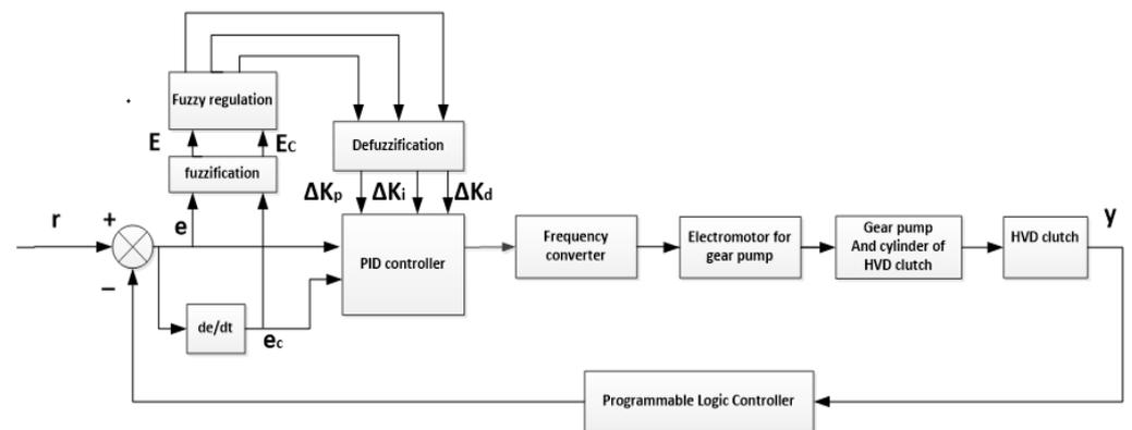
Figure 4. System block diagram based on the Fuzzy-PID controller.
