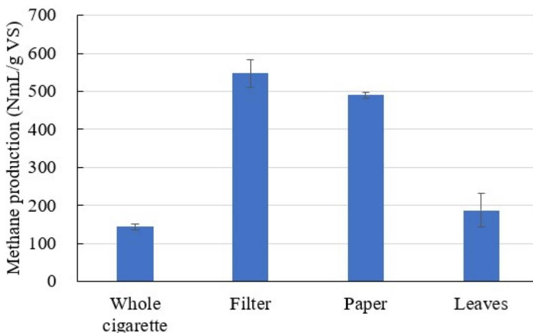
**Figure 2.** Amount of methane produced by each component of cigarette butts. Methane production was normalized using the division by volatile solids (VS).
