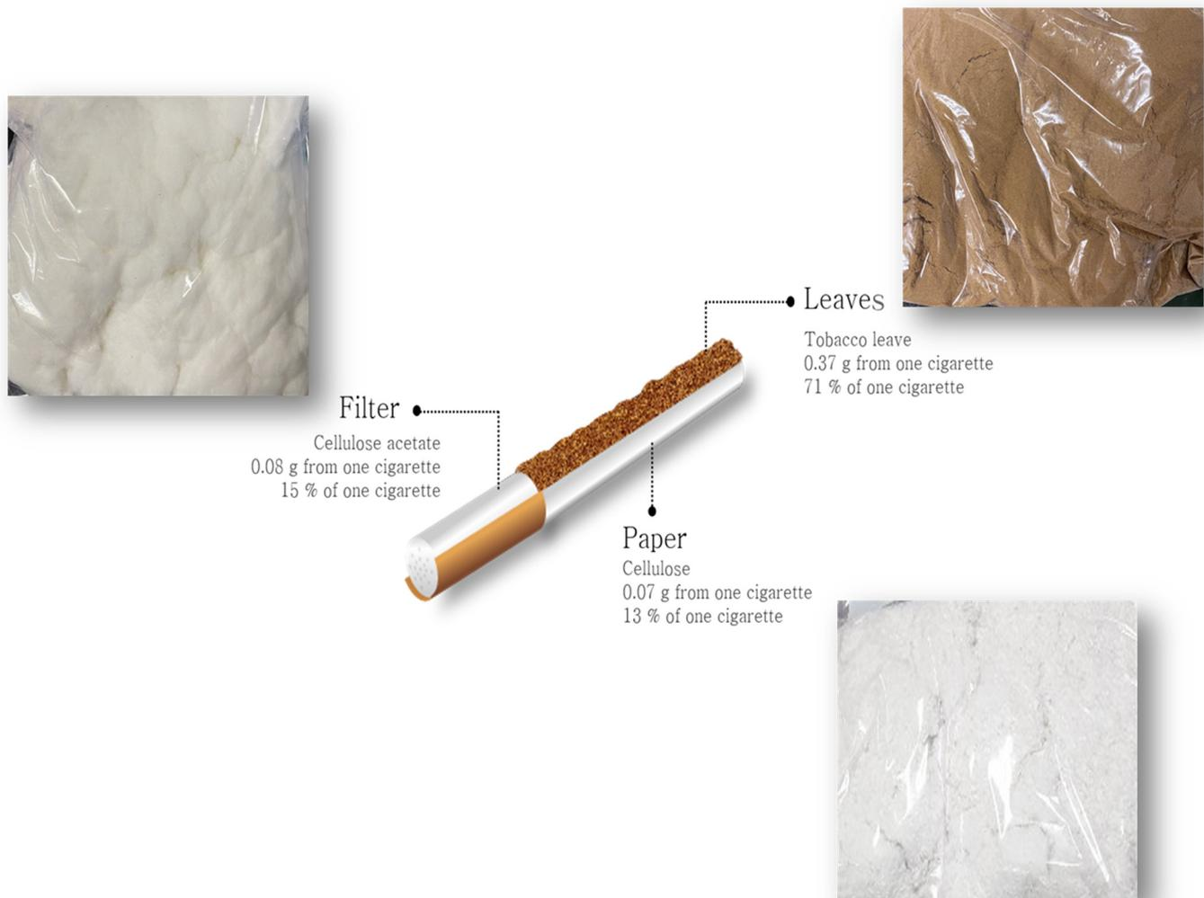
**Figure 1.** Cigarette composition used for anaerobic digestion. The inserted pictures show the powder after the chopping process.
