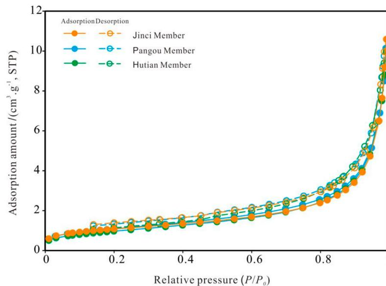
**Figure 7.** Nitrogen adsorption curve of the Benxi Formation shale.
