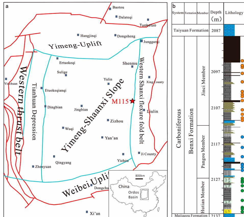
**Figure 1.** Structural diagram of the Ordos Basin (a) and histogram of the Benxi Formation (b). Green, blue, and orange circles represent samples from Hutian, Pangou, and Jinci members, respectively.
