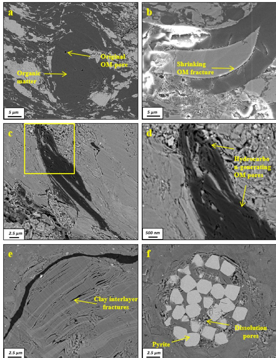
**Figure 9.** Scanning electron microscope microscopic characteristics of typical shale samples of the Benxi Formation. (a) Pores related to the structure of inherited primitive organisms; (b) shrinkage fractures and micro-fractures of organic matter; (c,d) Hydrocarbon generating organic matter pores; (e) clay interlayer fractures; (f) pyrite framboids and dissolution pores.
