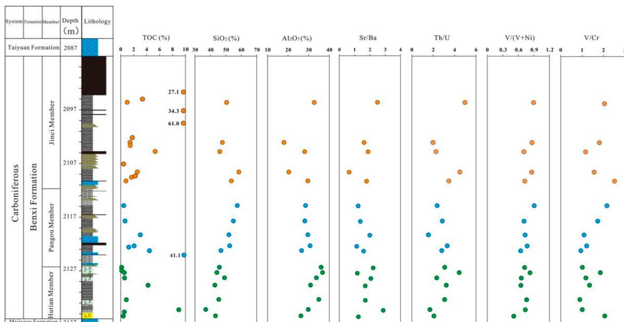
**Figure 2.** Vertical distribution characteristics of elemental geochemical parameters of the Benxi Formation shale.
