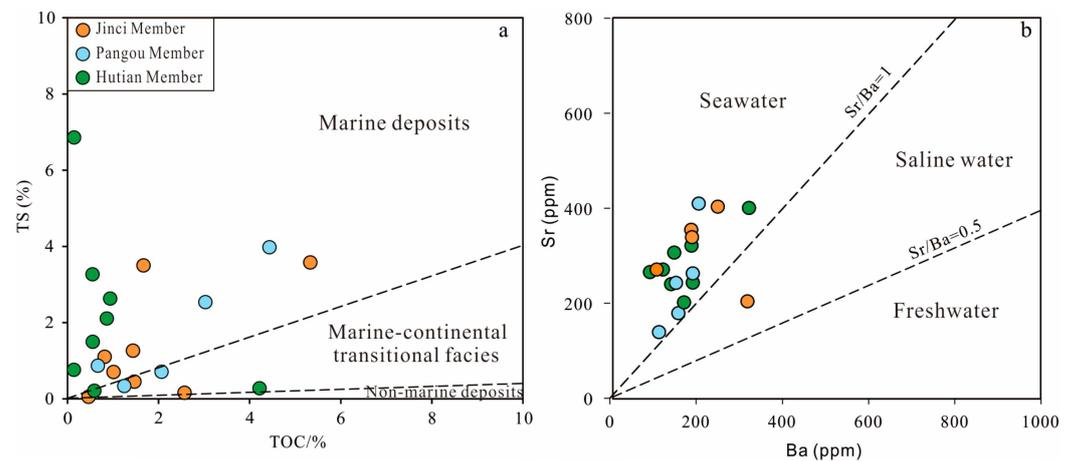
**Figure 3.** Identification of salinity of ancient water bodies for mud shale in the Benxi Formation. (a) Cross plot of total sulfur (TS) vs. total organic carbon (TOC), (b) Cross plot of Sr content vs. Ba content.
