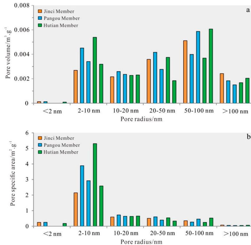
**Figure 8.** Distribution characteristics of pore volume (a) and pore specific surface areas (b) of the Benxi Formation shale.
