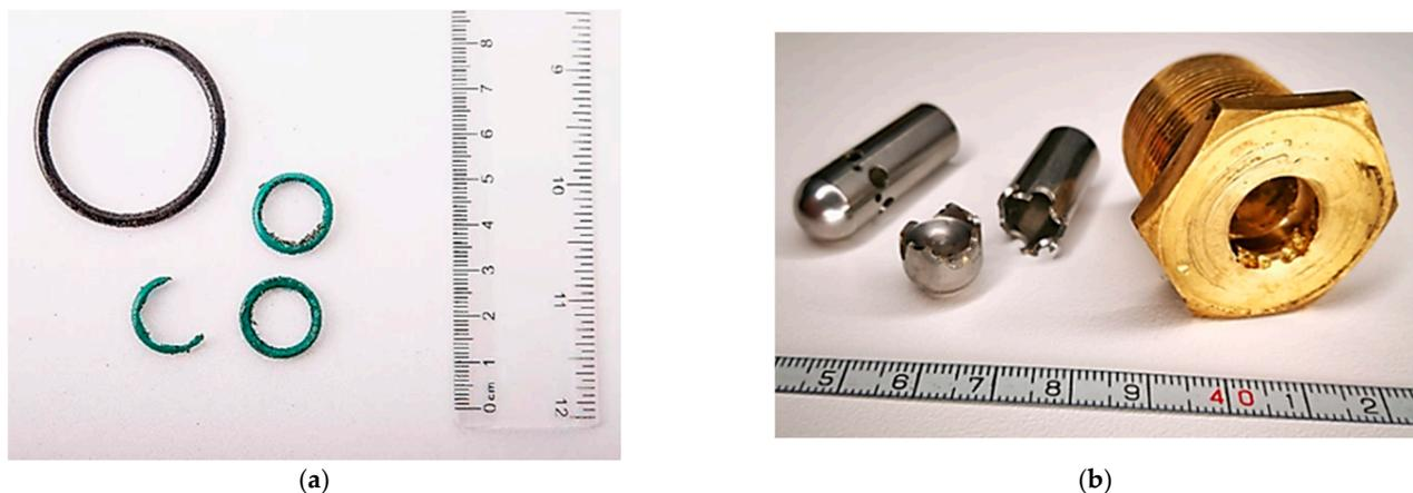
**Figure 4.** Examples of overflow valve damage: (a) damaged O-rings, (b) damaged pistons.
