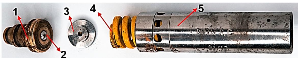
**Figure 3.** An example of the overflow valve: 1–O-ring of slide piston, 2–slide piston, 3–piston disc, 4–spring, 5–adjusting nut cover.
