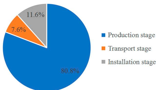
**Figure 7.** Proportion of carbon emissions at various stages in the whole construction process of CG-2 composite beams.
