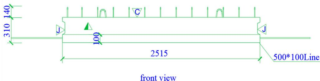
Figure 6. Front view of CG-2 composite beam.
