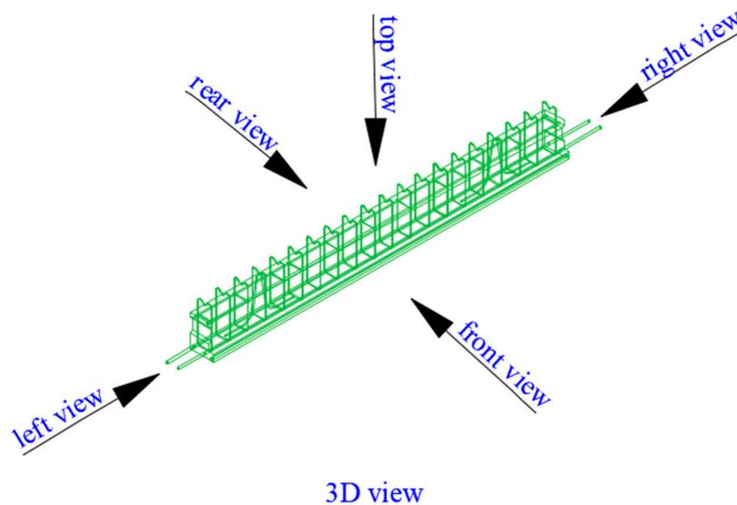
Figure 5. 3D view of CG-2 composite beam.
