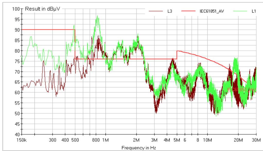
**Figure 9.** Conductive disturbance of the charging station, DC module operation (80% of power).
