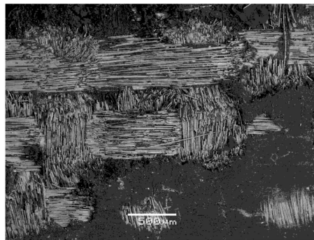
Figure 16. SEM image of the surface of the textolite material with very strong degradation effects (40 times magnification). The resin on the top layer of the material had been largely melted, charred and burned out. In the visible textile support, the fibre bundles were damaged and moved.
