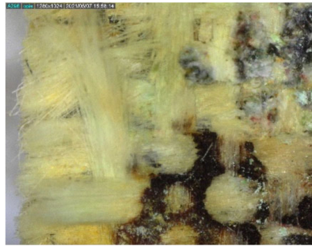
Figure 15. MO image of the marginal part surface of the textolite support, which was heavily degraded (40 times magnification). In the immediate vicinity of the edge, the resin had been almost completely burned out; the exposed textile support is visible.
