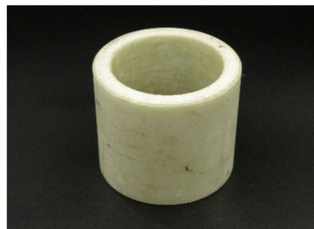
Figure 1. Textolite bushing support that came from an operated 110 kV surge arrester. Due to the lack of any degradation effects, the element was taken as a reference sample.
