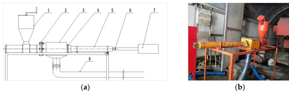
**Figure 5.** Dust hood testing system: (a) cross-section of the product: 1—screw-driven dust-generating device; 2—sealing pipeline; 3—dust hood; 4—dust control device; 5—drill pipe; 6—KJ25 interface; 7—air compressor; 8—dust collection pipe; (b) real product.
