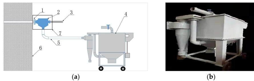
**Figure 3.** Dust control system for directional drilling in SBCS: (a) structure chart. 1—pre-embedded extraction pipe; 2—dust hood; 3—drill pipe; 4—dry dust collector; 5—dust collection pipeline; 6—coal mass; 7—dust control system in drilling; (b) real product.
