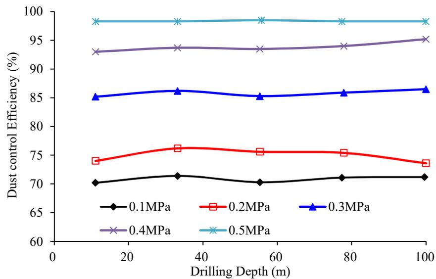
**Figure 8.** Dust control efficiency at different drilling depths.
