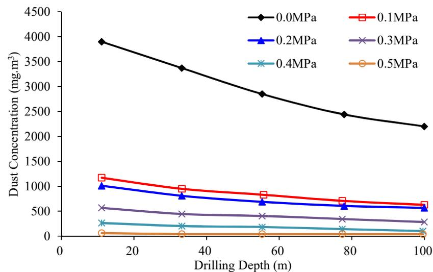
**Figure 7.** The dust concentration at different drilling depths.
