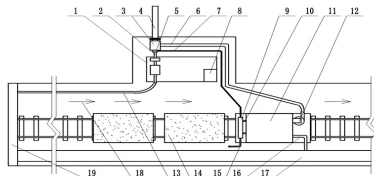
**Figure 6.** Layout of field-test device: 1—directional drilling rig; 2—drill pipe; 3—dust hood; 4—sealing casing; 5—pressure air sealing device; 6—slag discharge pipe; 7—KJ25 rubber hose; 8—drill driver’s position; 9—air storage tank; 10—air supply pipe of ejector; 11—bag filter; 12—cyclone dust collector; 13—air supply pipe for screw motor; 14—mine car; 15—air supply pipe for dust collector; 16—connection pipe of drainage system; 17—gas drainage pipe; 18—airflow direction; 19—air damper.
