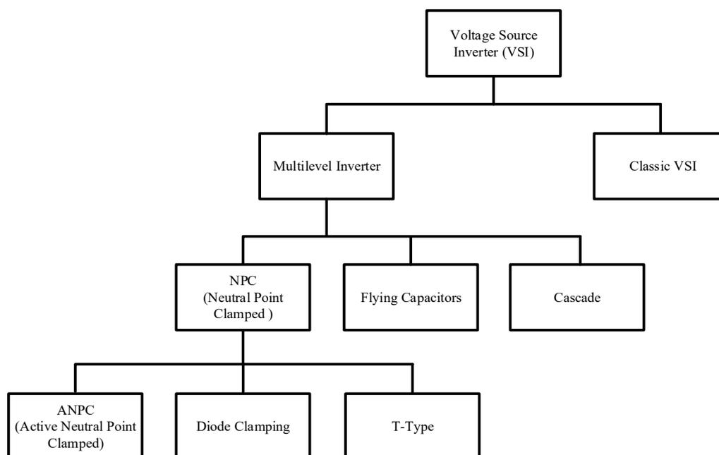
**Figure 1.** DC-AC converter classification.
