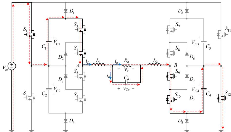
Figure 11. Current flow direction of stage III when the switch  $S_{10}$  is on.
