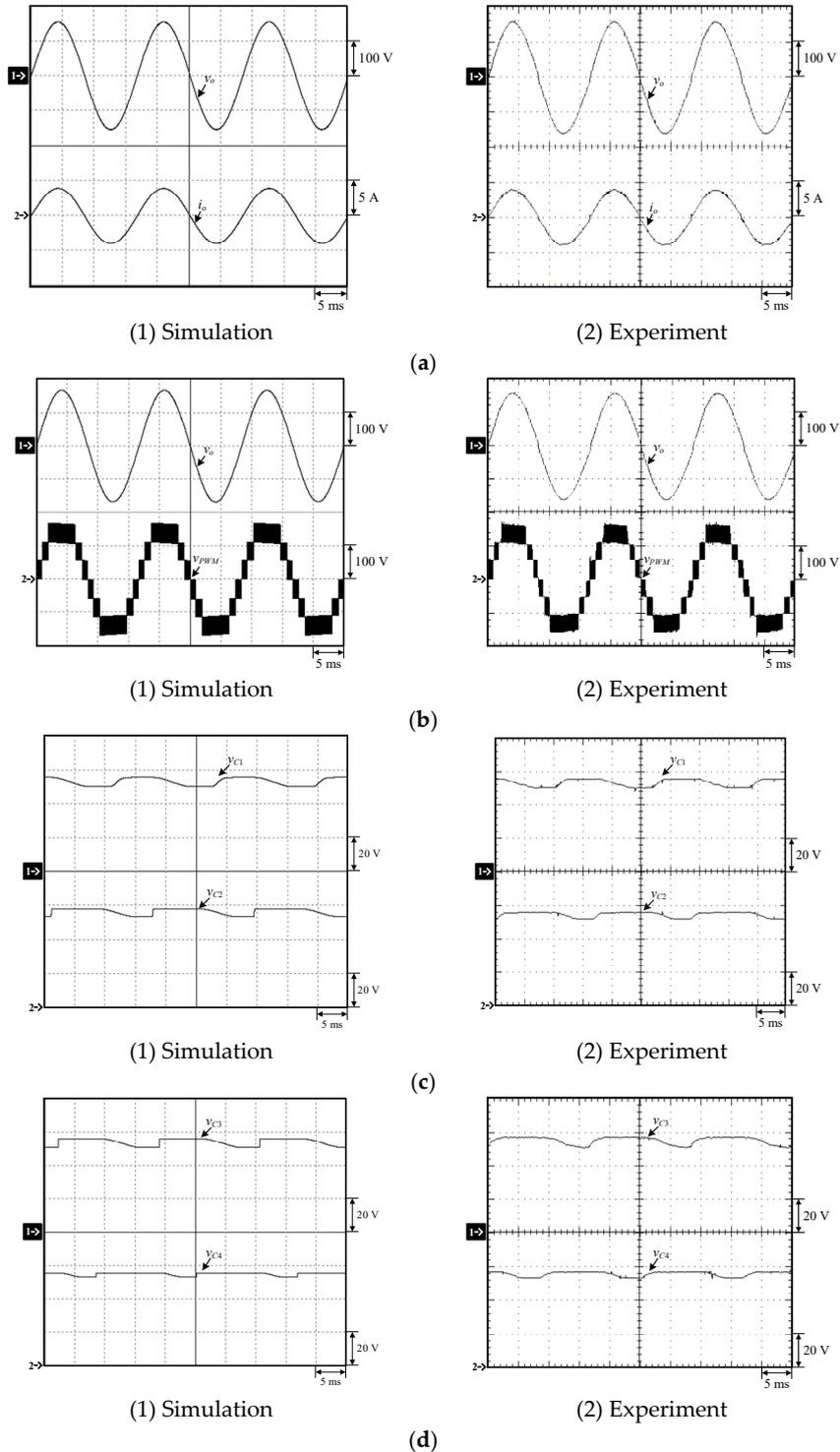
**Figure 16.** Simulated and experimental waveforms of the proposed DC-AC converter: (a)  $v_o$  and  $i_o$ ; (b)  $v_o$  and  $v_{PWM}$ ; (c)  $V_{C1}$  and  $V_{C2}$ ; (d)  $V_{C3}$  and  $V_{C4}$ .
