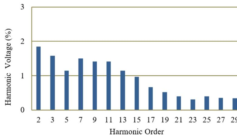
Figure 18. Distribution of harmonic voltages at minimum load.
