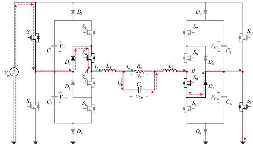
Figure 5. Current flow direction of stage I when switch  $S_1$  is on.
