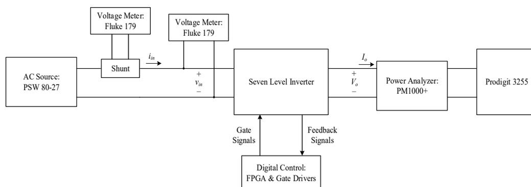
Figure 20. Block diagram of efficiency measurement.
