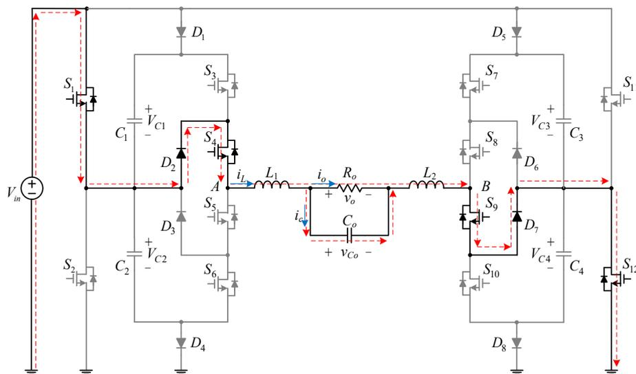
Figure 9. Current flow direction of stage II when switch  $S_3$  is off.
