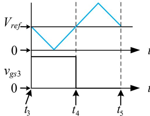
Figure 10. Gate driving signal for  $S_{10}$ .
