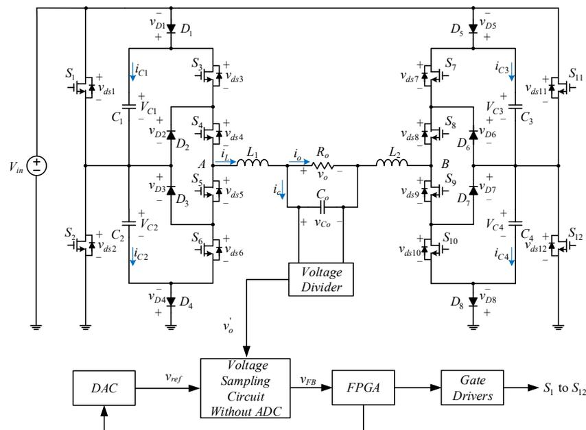
Figure 15. System block diagram of the proposed 7-level DC-AC converter.
