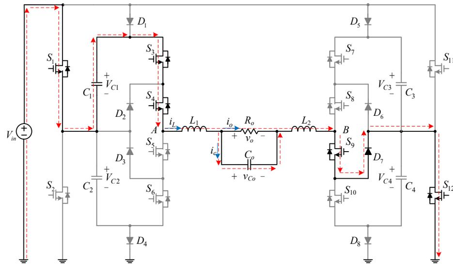
Figure 8. Current flow of stage II when switch  $S_3$  is on.
