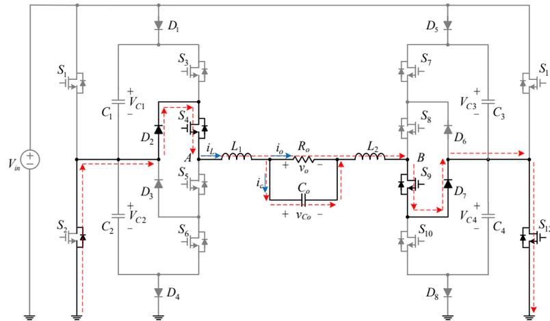
Figure 6. Current flow direction of stage I when switch  $S_1$  is off.
