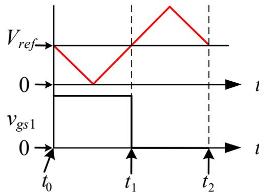
Figure 4. Gate driving signal for  $S_1$ .
