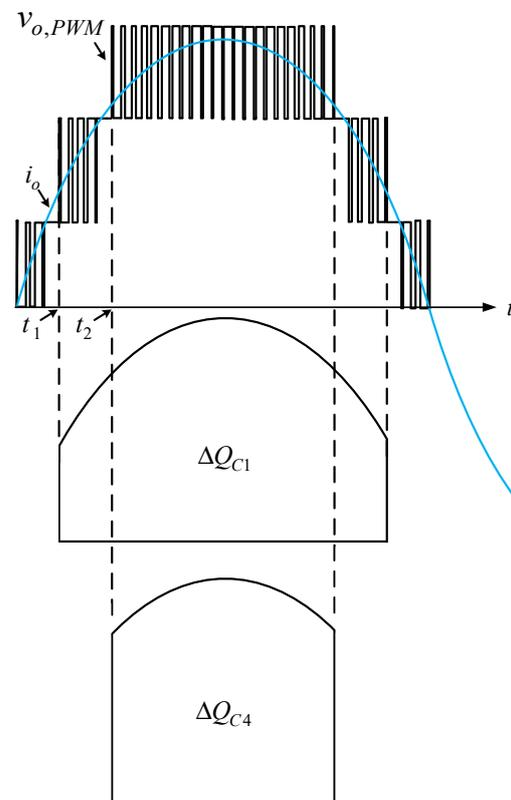
Figure 13. Charge of energy-transferring capacitors  $C_1$  and  $C_4$  during the discharge period.
