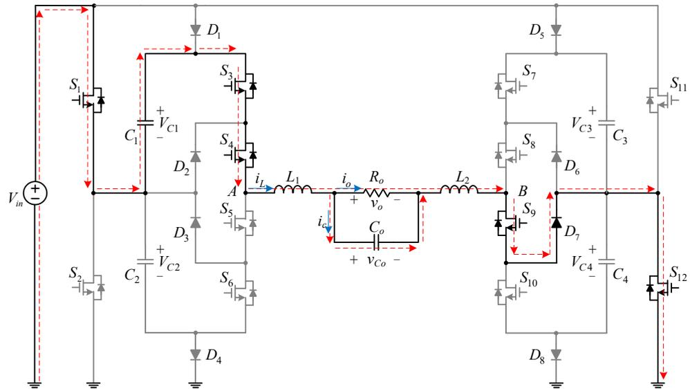
Figure 12. Current flow direction of stage III when switch  $S_{10}$  is off.
