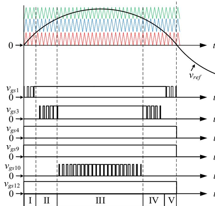
Figure 3. Waveforms of the gate driving signals for switches.
