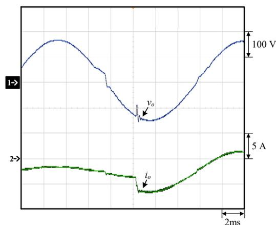
Figure 19. Load transient response due to step load current change from 25% to 100% load: (1)  $v_o$ ; (2)  $i_o$ .
