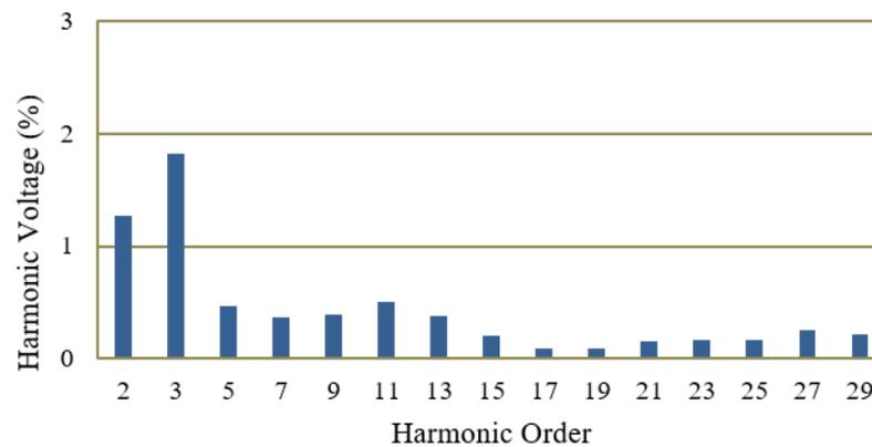
Figure 17. Distribution of harmonic voltages at rated load.
