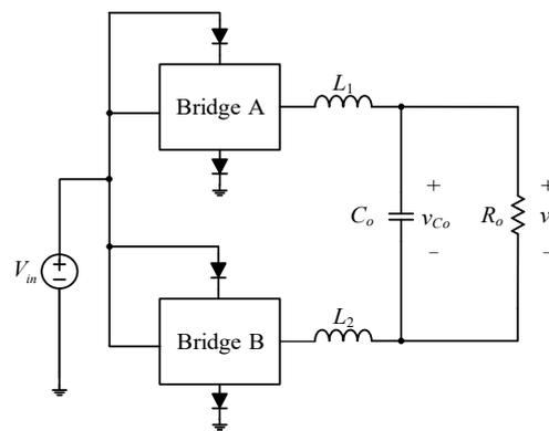
**Figure 14.** Filter circuit diagram for the output load.
