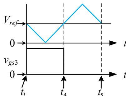
Figure 7. Gate driving signal for  $S_3$ .
