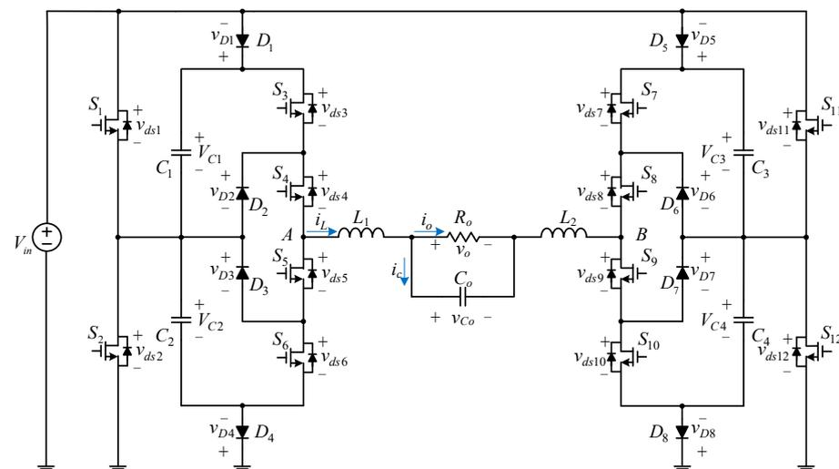
Figure 2. Single-voltage-source Class-D 7-level DC-AC converter.
