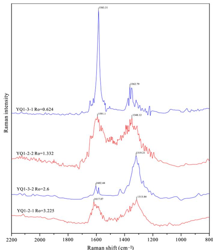
**Figure 6.** LRS of reservoir bitumen in Qingshuiying Formation in Well YQ-1. Red line: sampling depth is 4248.45 m; Blue line: sampling depth is 4249.9 m.
