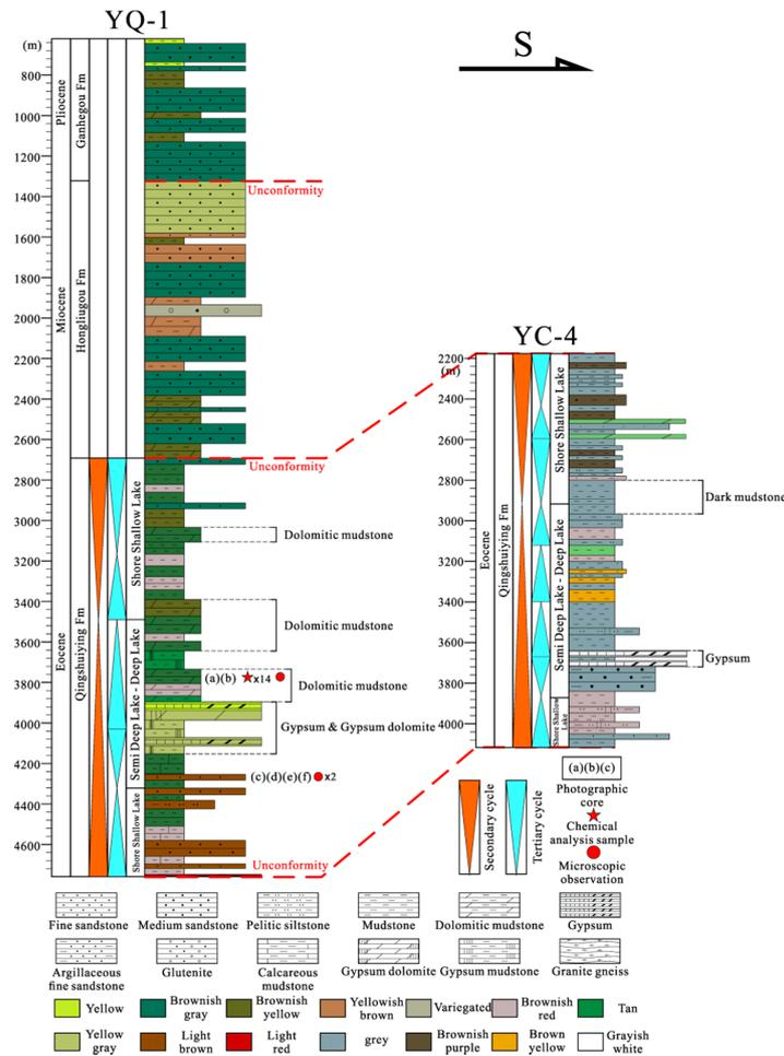
Figure 2. Logging interpretation of Well YQ-1 and Well YC-4 (see YQ-1 and YC-4 in Figure 1 for location) (Adapted from [6]).
