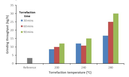
Figure 4. Grinding throughput of raw and torrefied corncobs.
