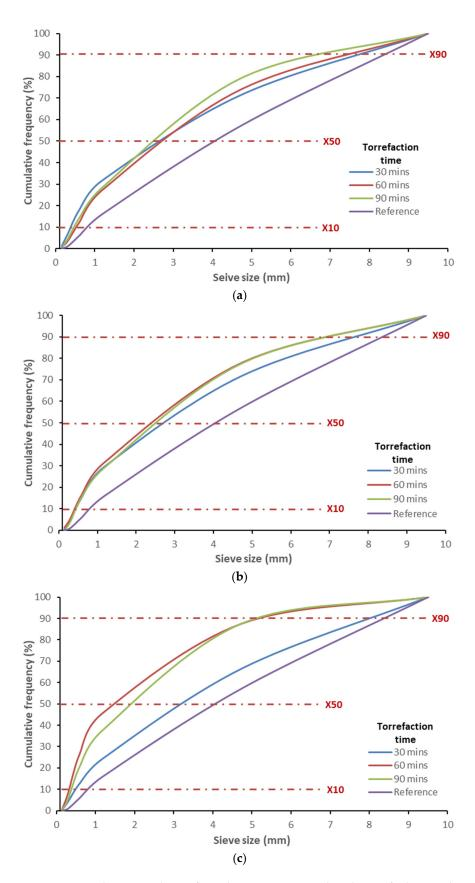
**Figure 5.** Particle size analysis of raw biomass compared with torrefied corncobs at: (**a**) 200 °C; (**b**) 240 °C; (**c**) 280 °C.
