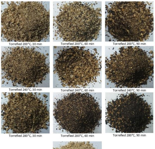
of carbon black. The milled products showing the changes in appearance of the torrefied corncobs with different treatment conditions are presented in Figure 3.
