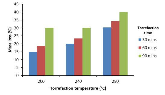
Figure 2. Mass loss during torrefaction of corncobs.
