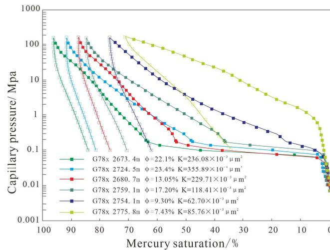
**Figure 7.** Mercury injection curves from pressure-controlled mercury injection of typical samples of Ek1 Formation in the Wang Guantun area.
