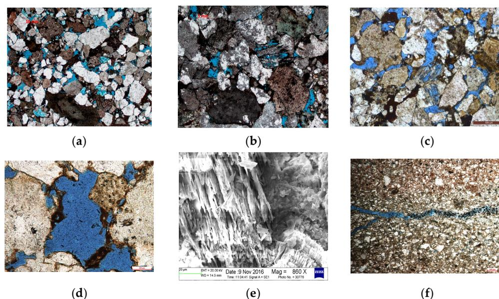
**Figure 6.** Pore types of reservoirs of Ek1 Formation in the Wang Guantun area. (a) Intergranular pore; (b) Intergranular dissolution pore; (c) Intergranular dissolution pore; (d) Mold pore; (e) Solution pores in feldspar; (f) Microcracks.
