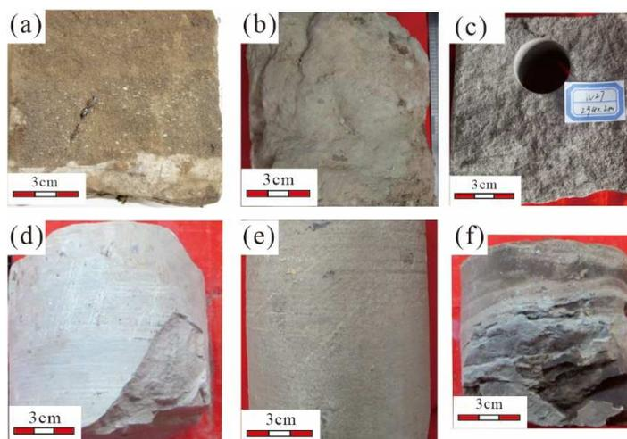
**Figure 3.** Core photos of Ek1 member in the Wang Guantun Area. (a) pebbly sandstone; (b) coarse sandstone; (c) medium fine sandstone; (d) siltstone; (e) argillaceous siltstone; (f) mudstone.
