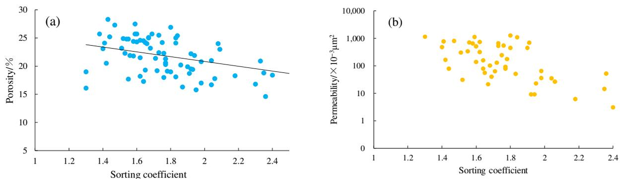
**Figure 11.** Relationship between sorting and physical properties of ZII<sub>3</sub> in the Wang Guantun area. (a) porosity and sorting coefficient; (b) permeability and sorting coefficient.
