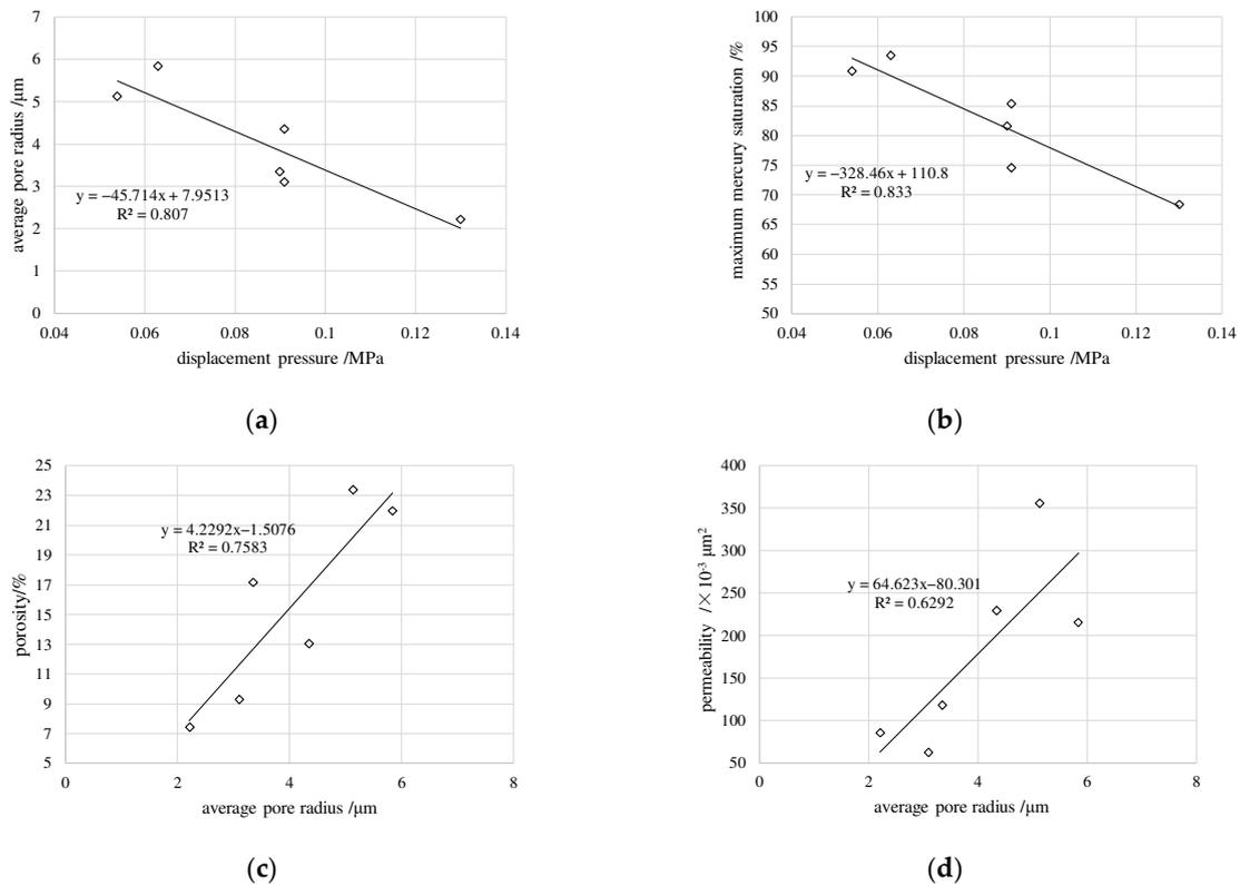
**Figure 8.** Relationship between parameters of pore structure and porosity, permeability of typical samples of Ek1 member in the Wang Guantun Area. (a) displacement pressure and average pore radius, (b) displacement pressure and maximum mercury saturation, (c) average pore radius and porosity, (d) average pore radius and permeability.
