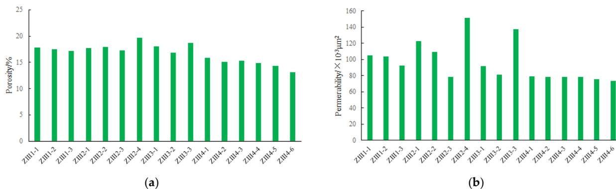
**Figure 5.** Reservoir properties of sub-sublayers of ZIII in the Wang Guantun Area. (a) porosity; (b) permeability.
