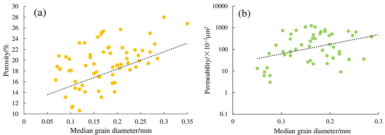
**Figure 10.** Relationship between particle size and physical properties of ZII<sub>3</sub> in the Wang Guantun area. (a) porosity and median grain diameter; (b) permeability and median grain diameter.
