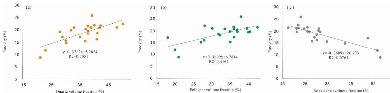
**Figure 9.** Correlation between clastic composition and porosity of Ek1 Formation in the Wang Guantun area. (a) porosity and quartz volume fraction; (b) porosity and feldspar volume fraction; (c) porosity and rock debris volume fraction.
