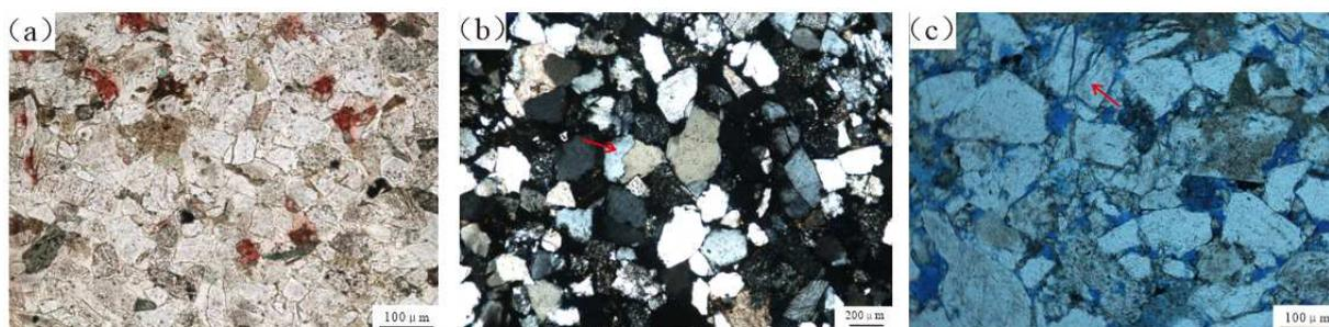
**Figure 13.** Compaction characteristics of Ek1 Formation in the Wang Guantun area (a) Well G50-5 1917.5 m (b) Well G106 3053.75 m, arrow refers to concave–convex contact (c) Well G11-13 2467.34 m, arrow refers to fracture.
