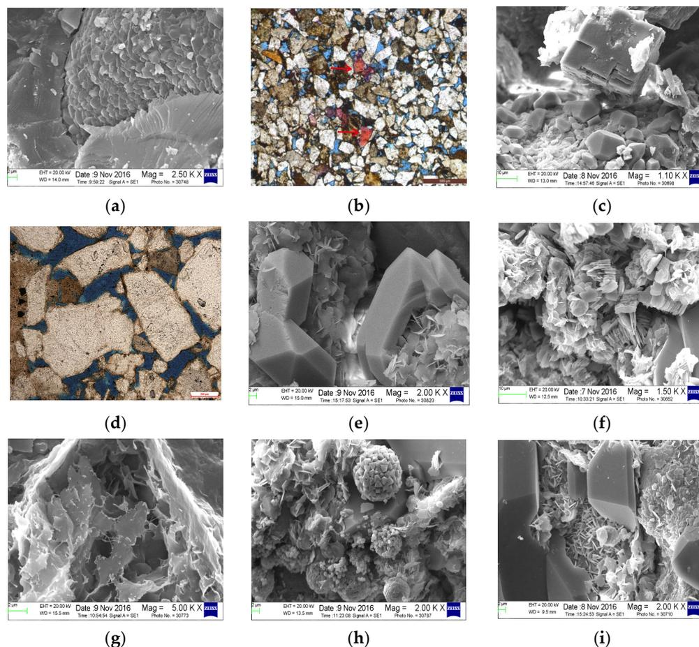
**Figure 15.** Cementing features. (a) Calcite; (b) Ferroan calcite; (c) Dolomite; (d) Secondary quartz; (e) Authigenic quartz; (f) Kaolinite; (g) Filiform Illite; (h) Pyrite; (i) Coniferous chlorite and Filiform Illite.
