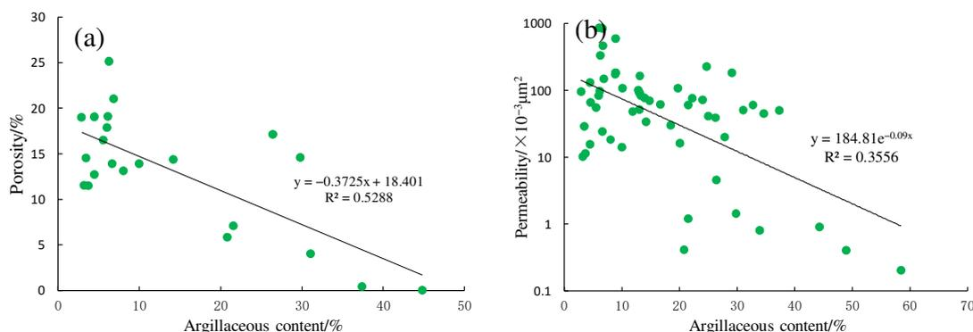
**Figure 12.** Relationship between shale content and physical properties of ZII<sub>3</sub> in the Wang Guantun area (a) argillaceous content and porosity (b) argillaceous content and permeability.
