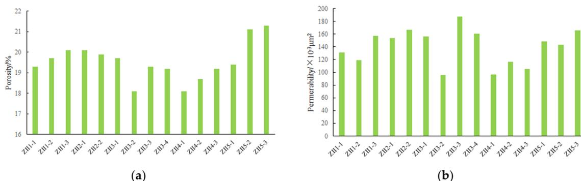
**Figure 4.** Reservoir properties of sub-sublayers of ZII in the Wang Guantun Area. (a) porosity; (b) permeability.
