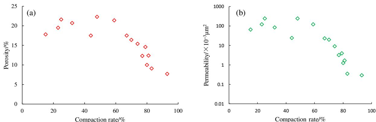
**Figure 14.** The relationship between porosity, permeability and compaction of Ek1 Formation in the Wang Guantun area. (a) porosity and compaction; (b) permeability and compaction.
