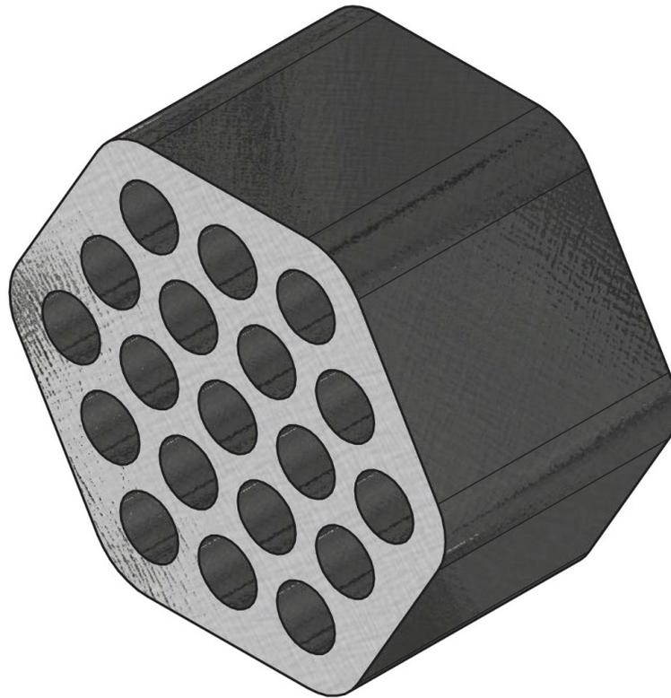
**Figure 5.** Isometric view of the SIRIUS-CAL fuel specimen.
