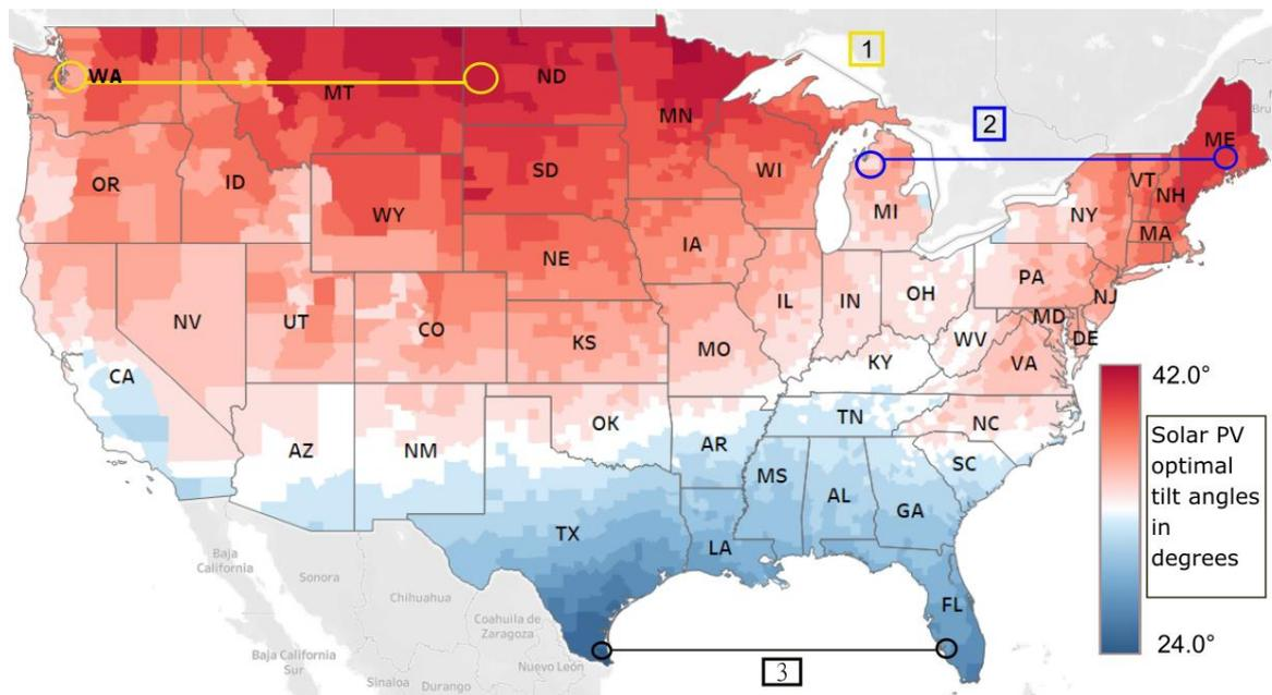
Figure 5. Solar PV optimal tilt angle in degrees for every United States county, showing locations of interest where optimal tilts differ at similar latitudes. The circles connected with lines, labeled with the boxed values 1, 2 and 3, indicate counties of similar latitude that are used for comparison cases.
