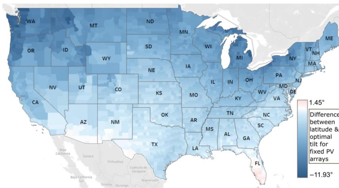
**Figure 6.** Calculated difference between optimal tilt angle and location latitude.
