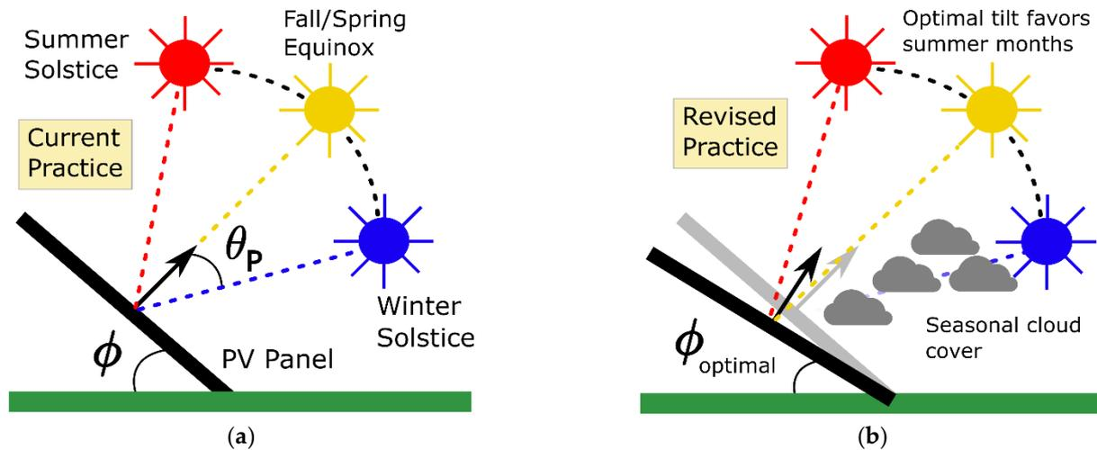
**Figure 1.** (a) A depiction of a commonly accepted practice for deploying PV panels, where the tilt angle is equivalent to the latitude of the PV panel geographic location. (b) A revised practice where the PV tilt angle is revised to reflect seasonal weather patterns and seasonal variations in daylight hours.
