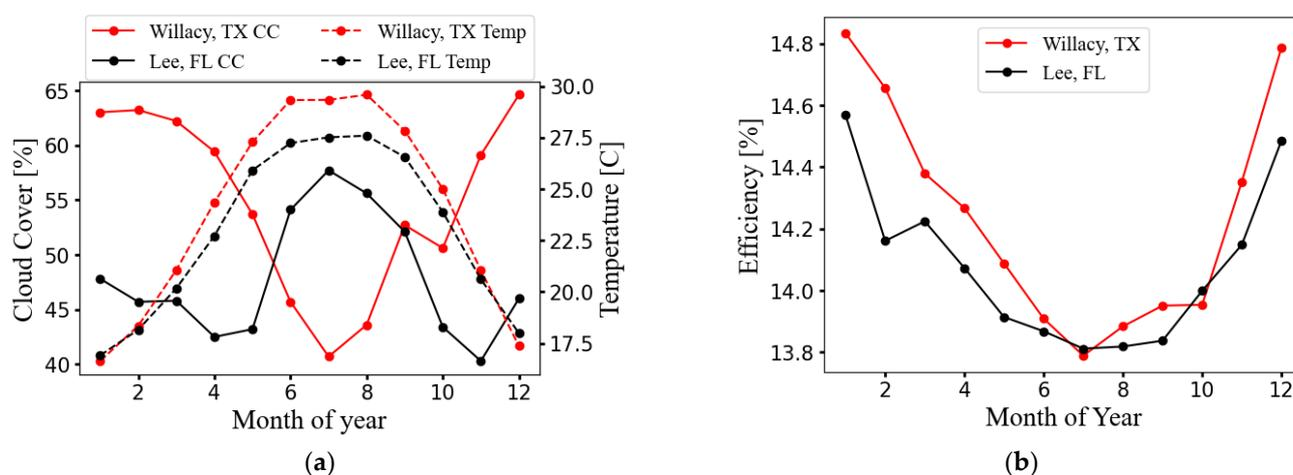
**Figure 10.** (a) Comparison of seasonal cloud cover and ambient temperatures for case 3 indicated in Figure 5. (b) The temperature dependent efficiency of PV panels for case 3 locations.
