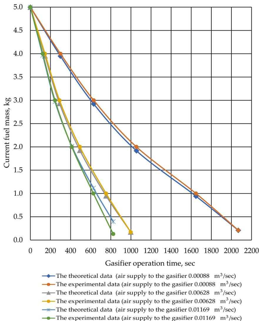
**Figure 4.** Comparison of the experimental and theoretical indicators of a change of fuel mass when using wood in pieces.
