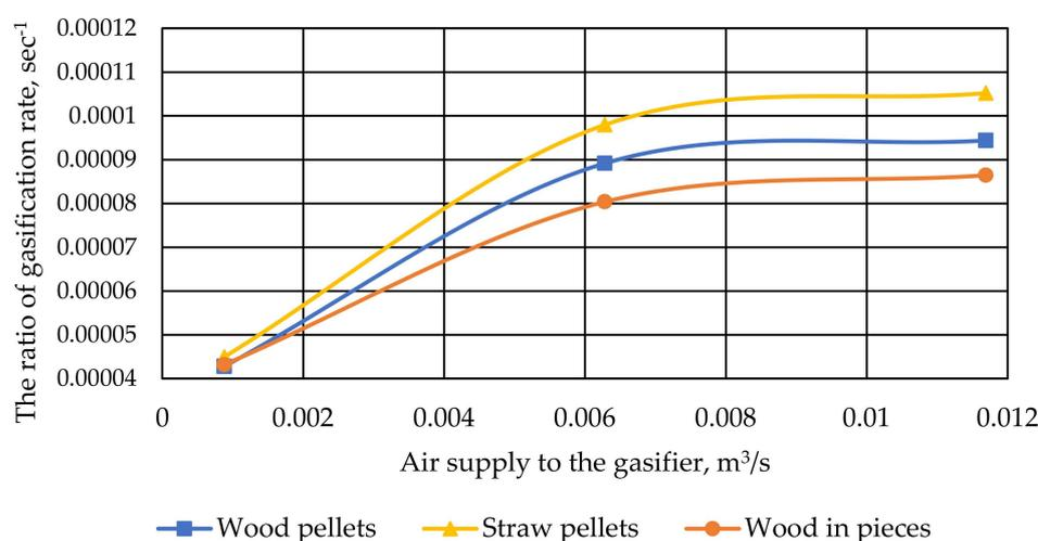
**Figure 5.** Change of the coefficient of gasification rate depending on air supply.
