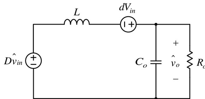
Figure 11. Small-signal AC model of the proposed inverter.
