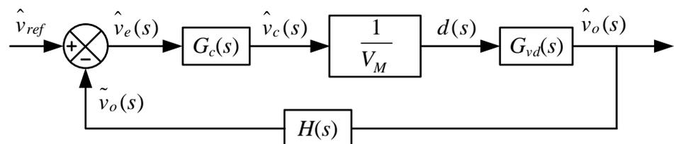
Figure 12. System block diagram for voltage feedback control of the proposed circuit.
