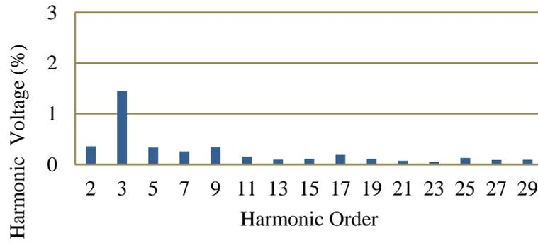
Figure 22. Voltage harmonic distribution at 100% load.
