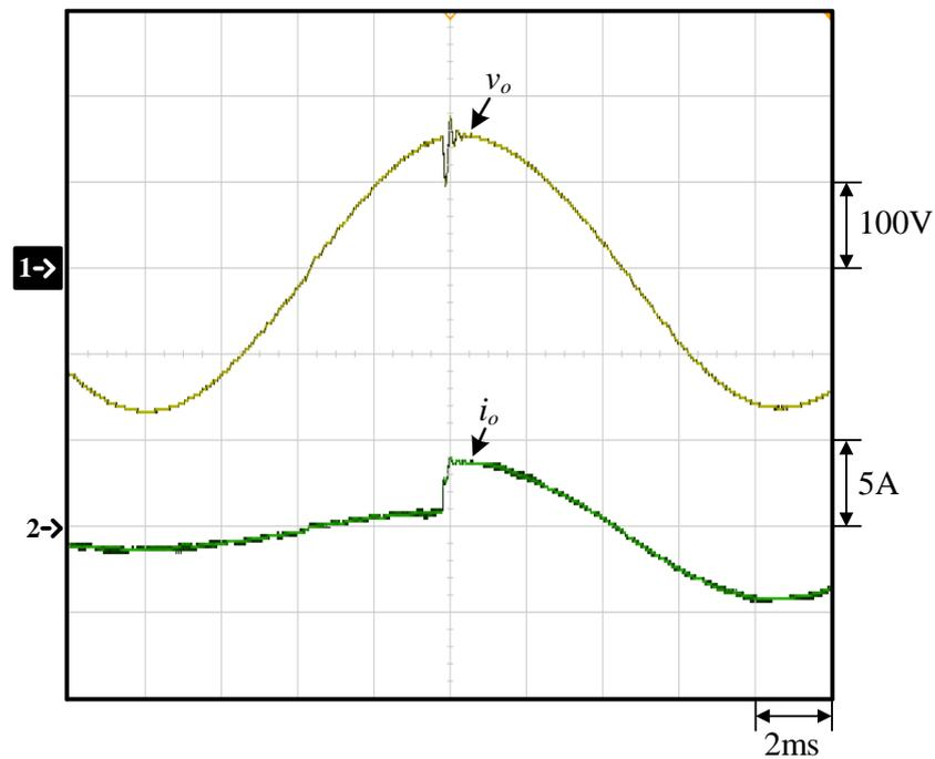
Figure 20. Measured waveforms of uploading from 25% load to 100% load: (1)  $v_o$ ; (2)  $i_o$ .
