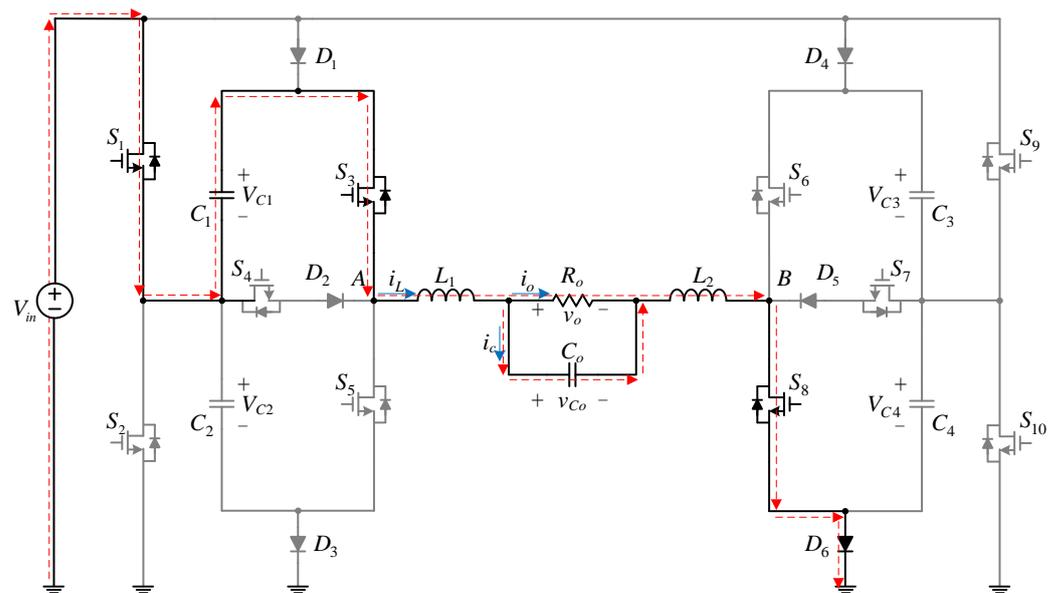
Figure 7. Power flow as  $S_3$  is conducted.
