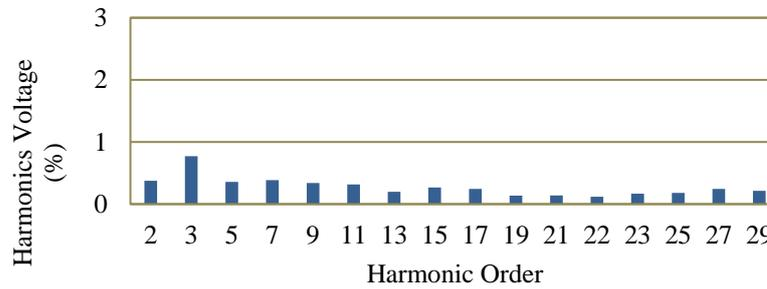
Figure 23. Voltage harmonic distribution at 25% load.
