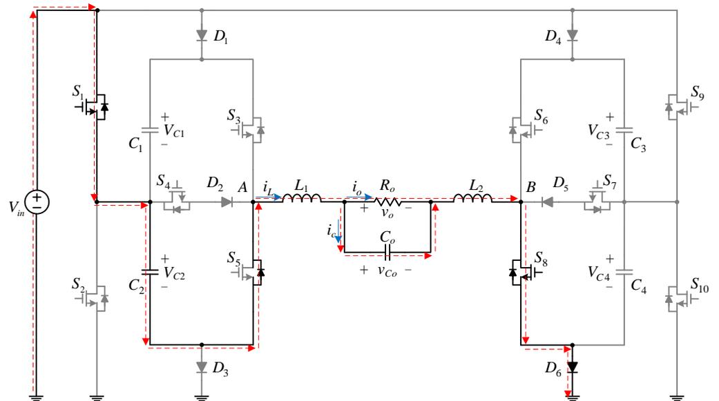
Figure 5. Power flow as  $S_4$  is cut off.
