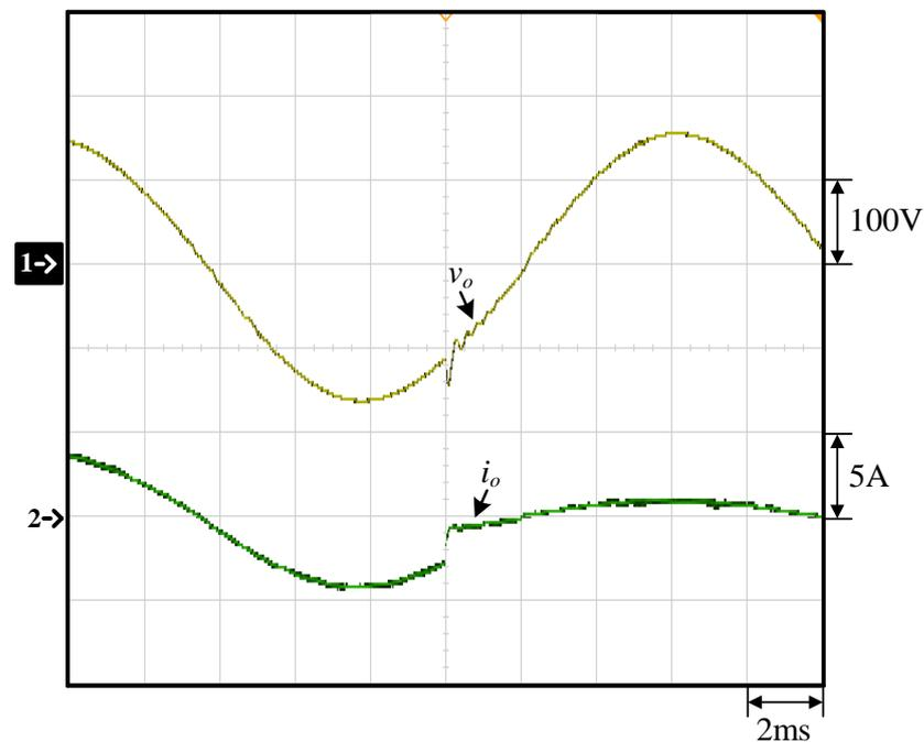
Figure 21. Measured waveform of downloading from 100% load to 25% load: (1)  $v_o$ ; (2)  $i_o$ .
