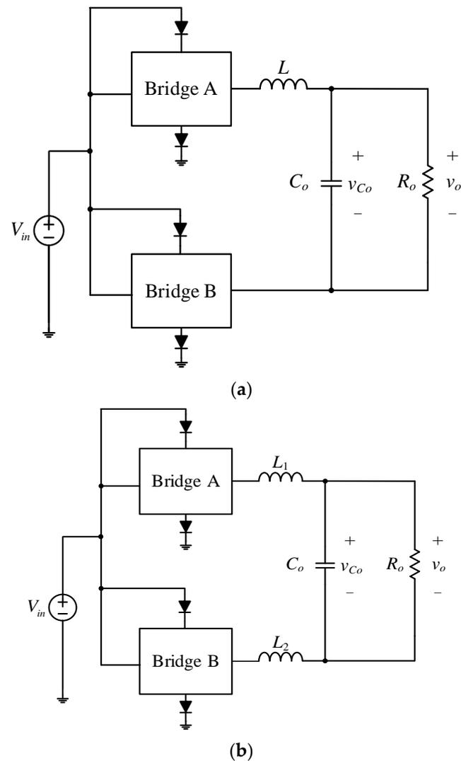
**Figure 10.** Filter circuit diagram from the point of view of the output load with the inductance of (a)  $L$ ; (b)  $L_1$  and  $L_2$ .
