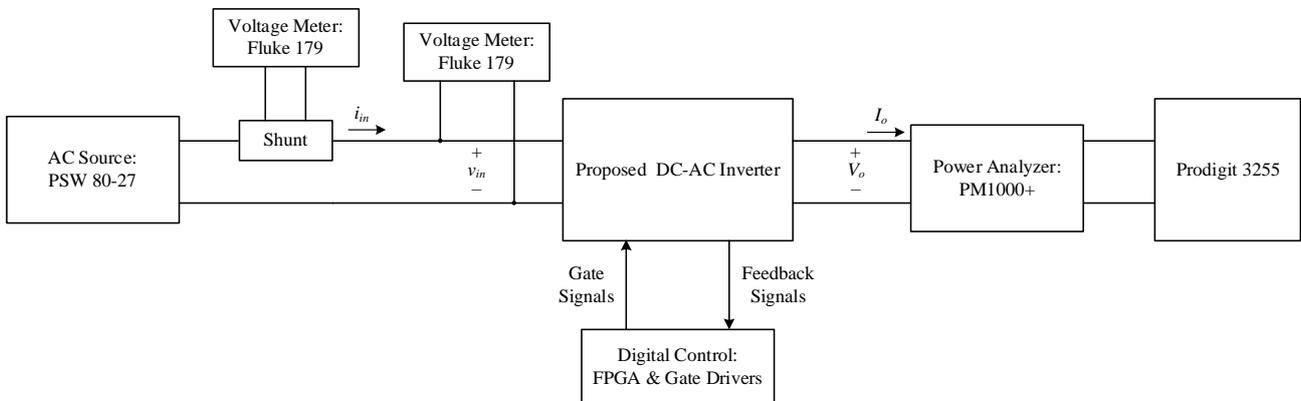
Figure 24. Efficiency measurement block diagram.
