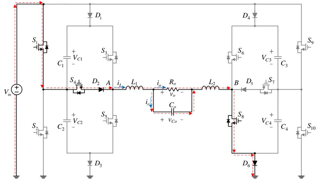
Figure 4. Power flow as  $S_4$  is conducted.
