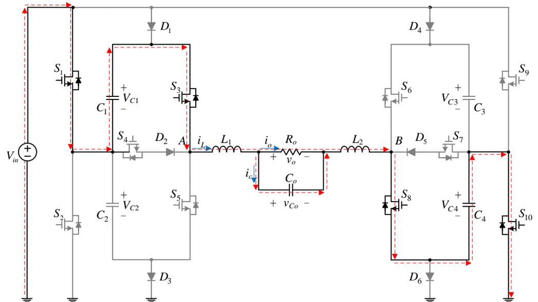
Figure 9. Power flow as  $S_{10}$  is conducted.
