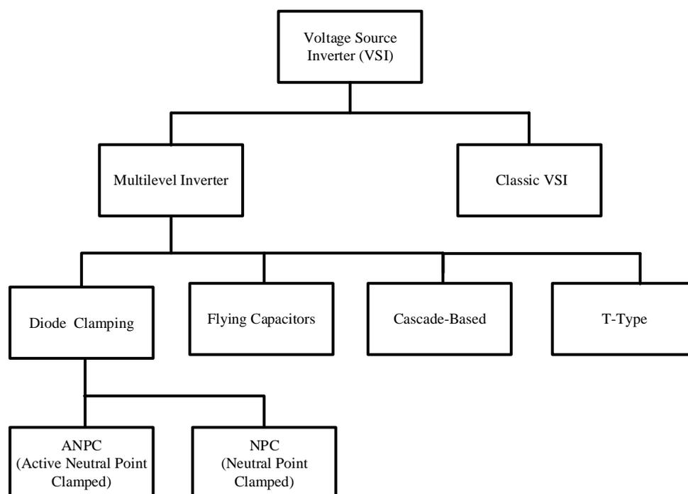
**Figure 1.** Voltage source DC-AC inverter classification.
