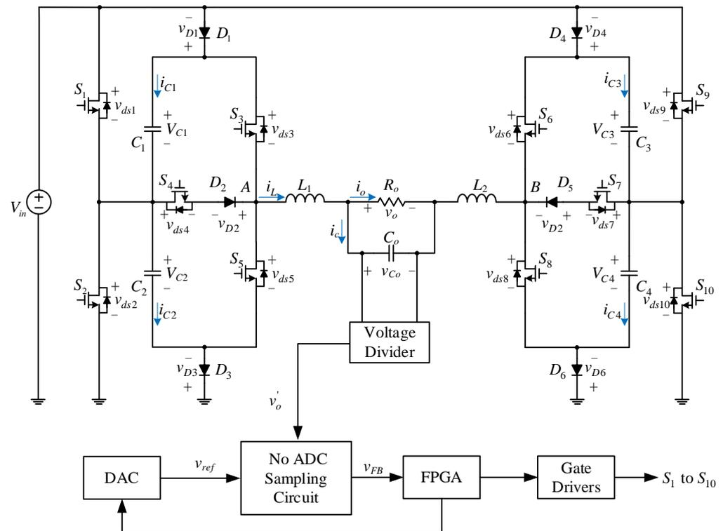
**Figure 14.** System configuration for the 7-level single-phase DC-AC inverter.
