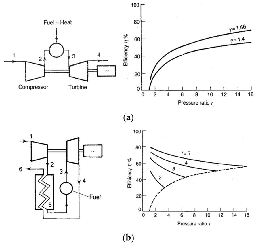
**Figure 8.** Cycle efficiency based on pressure ratio, (a) simple cycle, (b) regenerative cycle [49]. In schematic diagrams of gas turbine cycles in (a,b), the numbered locations are: 1. engine inlet, 2. compressor outlet, 3. combustor outlet, 4. turbine outlet. additional locations in (b): 5. recuperator outlet—cold-side and 6. recuperator outlet—hot-side. In efficiency diagram of (b)  $t$  is defined as ration of turbine inlet temperature to engine inlet temperature.
