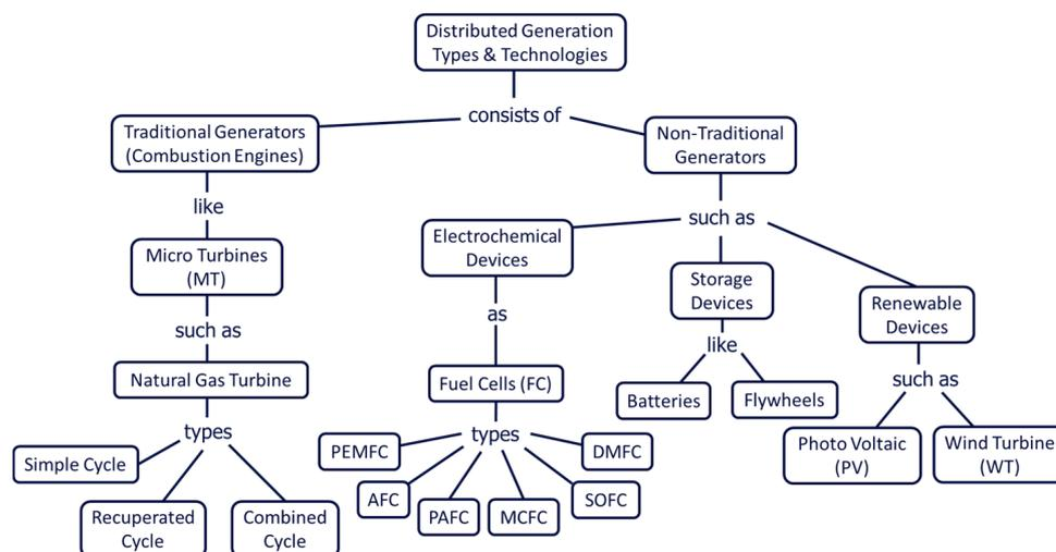
**Figure 2.** Distributed generation types and technologies [8].
