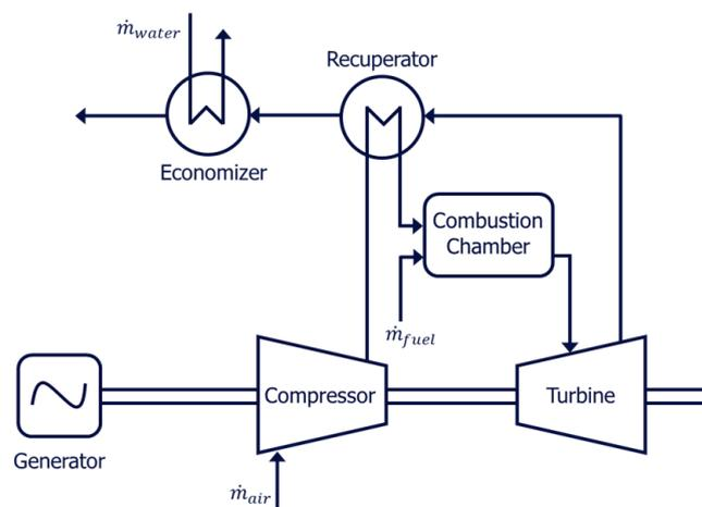
**Figure 9.** Typical MGT cycle with recuperator and economizer for combined heat and power generations.
