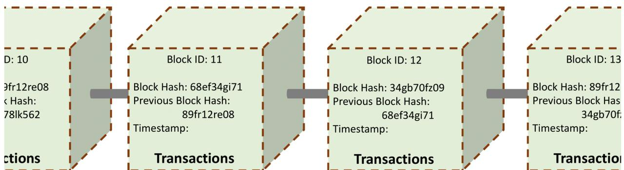
Figure 4. General structure blocks in the Blockchain concept.
