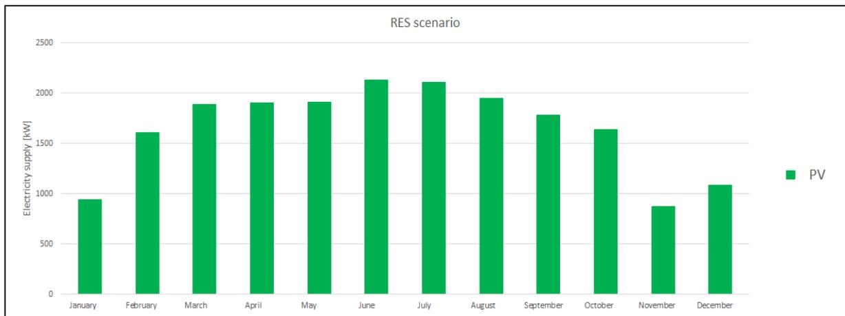
Figure 8. Average PV systems' output power values for Scenario 2.
