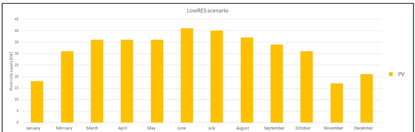
**Figure 7.** Average PV systems’ output power values for Scenario 1.
