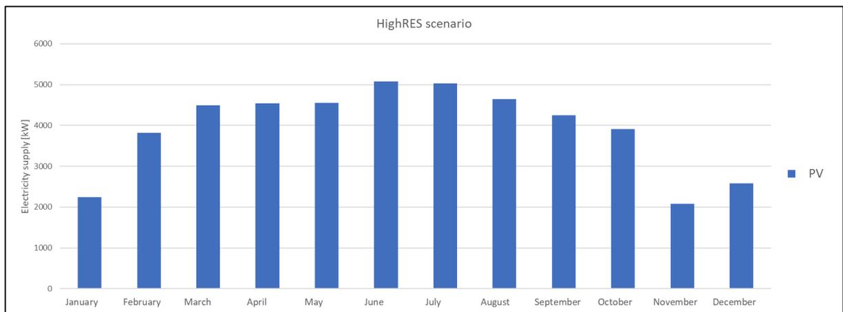
Figure 9. Average PV systems' output power values for Scenario 3.
