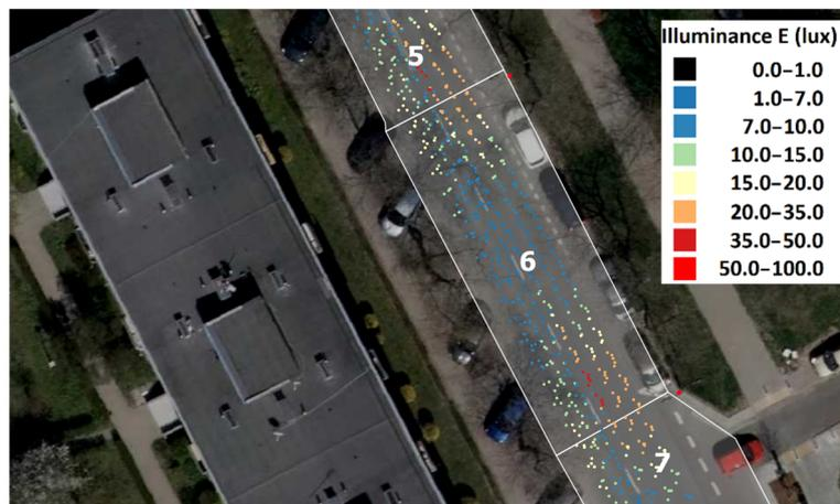
Figure A4. Example of five illuminance measurements in field No. 6.
