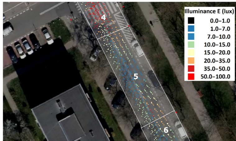
Figure A3. Example of five illuminance measurements in field No. 5.
