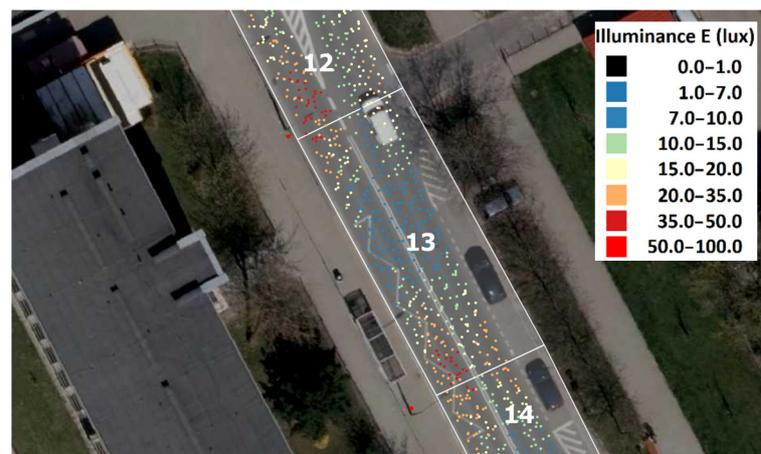
Figure A8. Example of five illuminance measurements in field No. 13.
