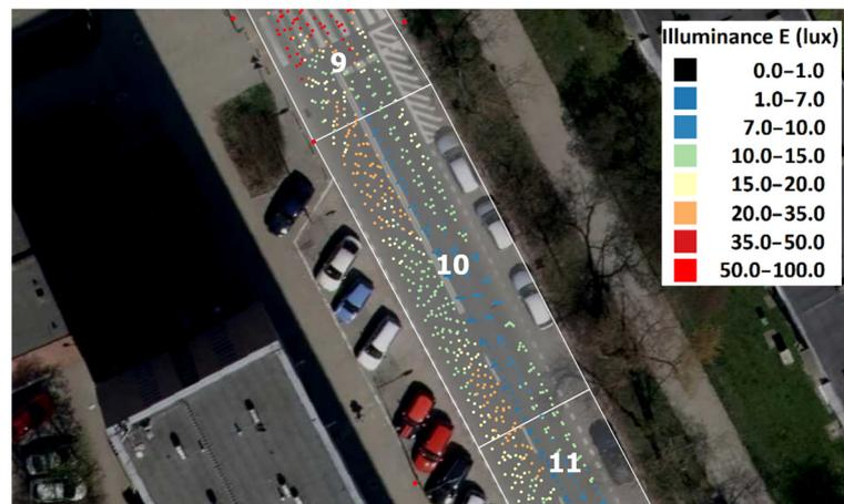
Figure A6. Example of five illuminance measurements in field No. 10.
