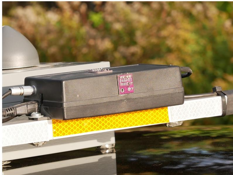
**Figure 7.** Illuminance sensors for horizontal and vertical plane measurement located in the central position of the measurement system.
