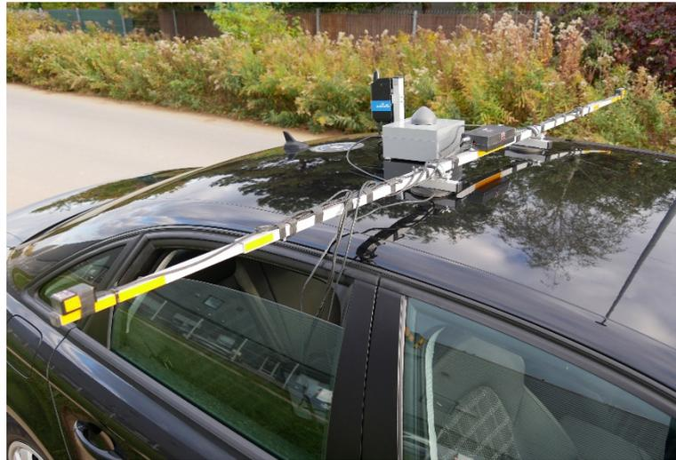
**Figure 5.** Light intensity measuring system with GPS RTK mounted on the roof of the vehicle.
