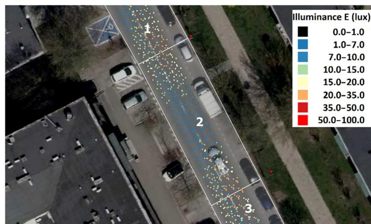
Figure A1. Example of five illuminance measurements in field No. 2.
