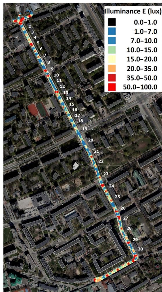
**Figure 12.** Illumination intensity map recorded with the geolocated GPS RTK measurement system along the entire section of Smocza Street, with the measurement field numbers marked.
