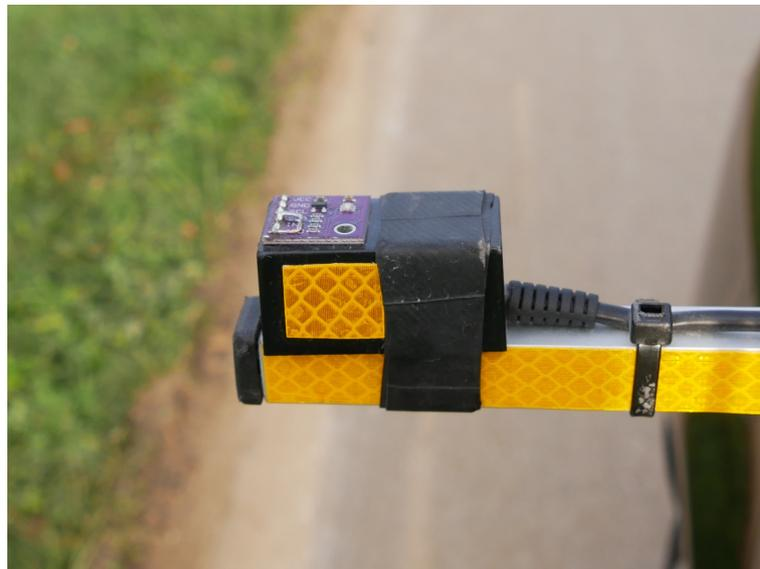
**Figure 6.** Illuminance sensor for horizontal plane measurement.
