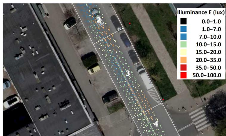
Figure A2. Example of five illuminance measurements in field No. 3.
