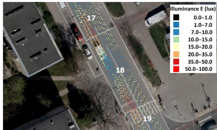
Figure A9. Example of five illuminance measurements in field No. 18.
