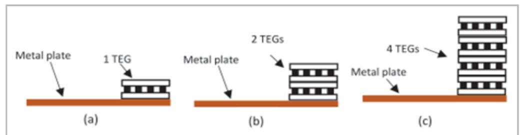
**Figure 13.** TEG module configurations; (a)  $4 \times 1$ , (b)  $2 \times 2$ , (c)  $1 \times 4$  [92].
